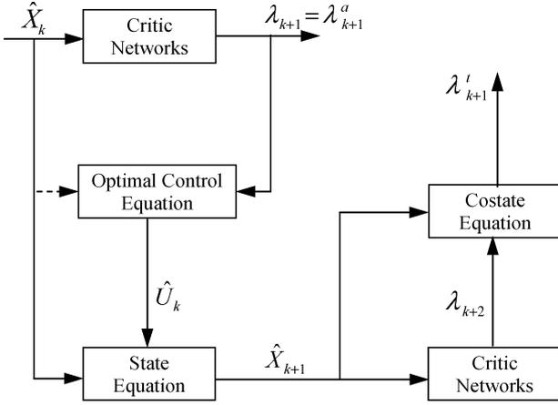
Fig. 1. Schematic of simplified adaptive critic neural-network synthesis.
