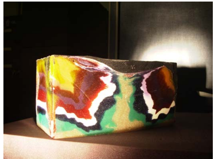
Fig. 5. Cutaway view of sand layers (originally horizontal) as they were deformed beneath the surface of a crater.
