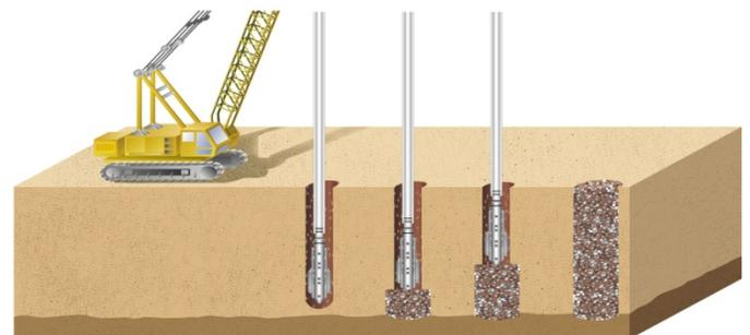
Fig 5. Stone column installation procedure, left to right..
