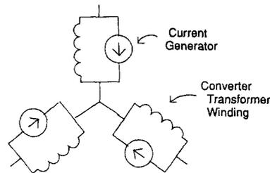
Figure 2: Separate Current Generators Used with Each Winding
