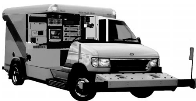
FIGURE 6 Cutaway of data acquisition vehicle showing video camera, computers, video recorders, and camera.
