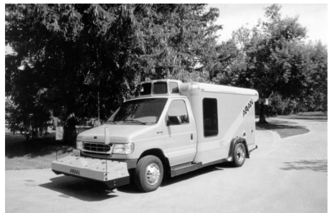
FIGURE 4 Roof-mounted video for panoramic view.
