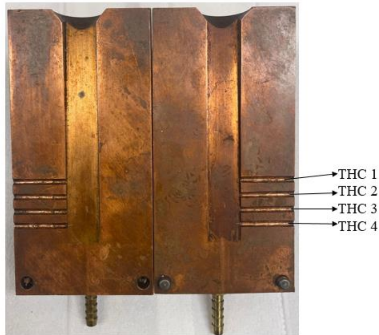
Figure 3.4: Copper mold with machined K-type thermocouple hollow.
