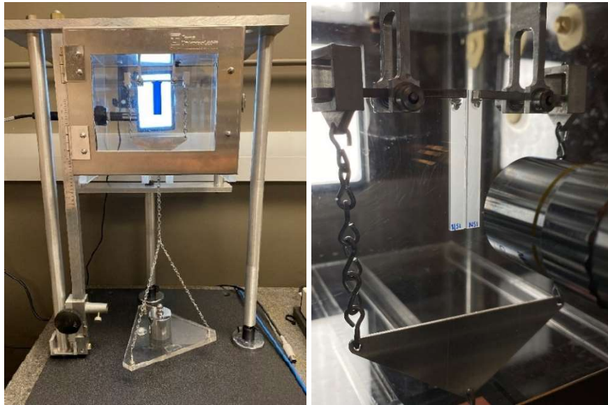
Figure 2.1: Environmental chamber and DCB assembly used to measure crack velocity at different stress intensities.
