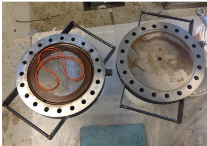
Figure 3.7 High-Pressure Injection Mold (Top Plate, Spacer, and O-rings on left; Bottom Plate on Right)
