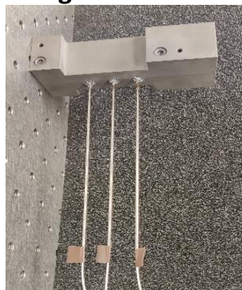
Figure 4. Flux mold, EFPI sensors installed with shielding. a) shows the back components of the mold and point gap sensors after EFPI installation, step profile can be observed. b) the front component bolted to the back components after EFPI installation such that the wall is facing the sensor. c) Top view of the mold setup, where the synthetic molten flux sample is poured. d) Stainless-steel tubing protection to the SMF cables coming out of the back side of flux mold.
