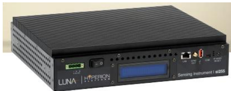
Figure 2.2. Micron-optics Hyperion SI-255 EV Optical Interrogator. The Micron-optics Hyperion SI-255 EV optical interrogator was used to measure the real-time EFPI interferogram for the gap and thickness measurements in high temperature applications in this research. It has a 16-channel capacity and provides APIs (application programming interface) for developing data acquisition tools. It has a swept laser source with a sweeping rate of 10 Hz and a wavelength range of 1460 nm to 1620 nm.
