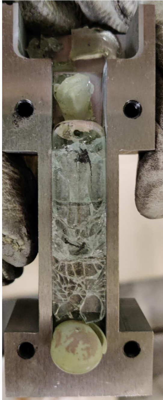
Figure 16. Cracking seen during solidification of H2-9 flux film sample. The solidifying flux sample vibrates during crack formation which leads to the noisy air gap measurement as shown in Figure 15. The effects of cracking can be minimized by pre-heating the mold before the experiment.
