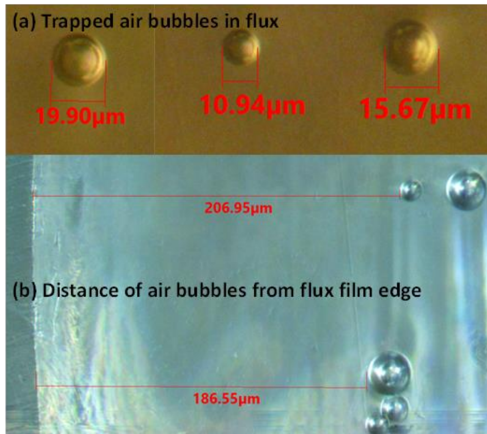
Figure 20. Flux sample with air bubbles in EFPI path. a) Trapped air bubbles in flux and b) Distance of air bubbles from flux film edge facing EFPI sensor. After a portion of light gets reflected at the flux film's edge in the air gap, some light penetrates the flux film boundary and goes through the flux, where again some light gets reflected by the trapped air bubble within the flux. The air bubbles shown here are at 206.95 μm and 186.55 μm from the flux film boundary.
