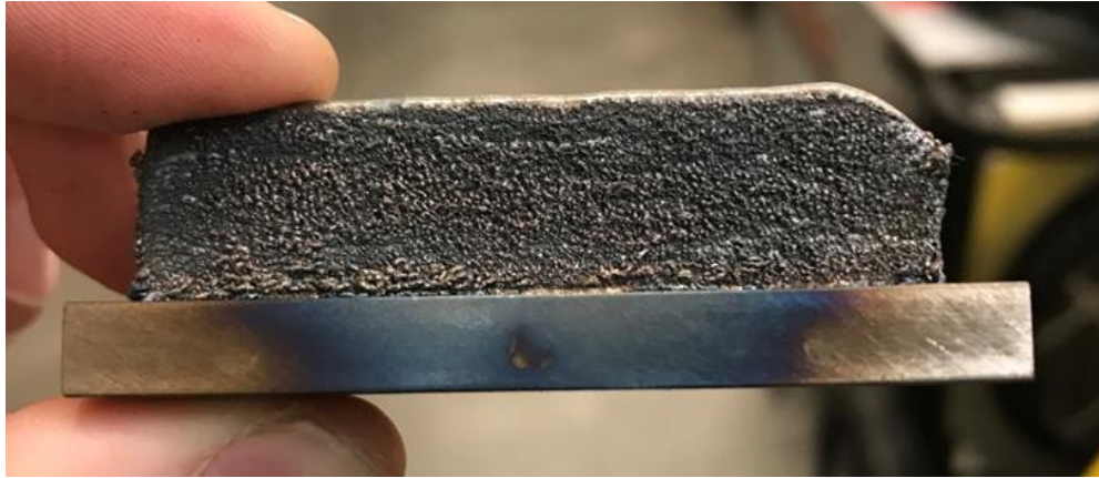
Figure 2.10 One of the 21 Single-track DOE Samples in Stage 2.
