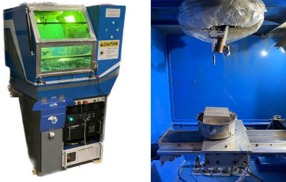
Figure 2.4 The Hybrid Cell DED system used in Stage 1 Equipped with One 1000w Pulse Laser Driving a 2 mm Diameter Laser Beam, One Wheeling Feeder, and One 3-degree of Freedom Gantry Controlled by the LinuxCNC.
