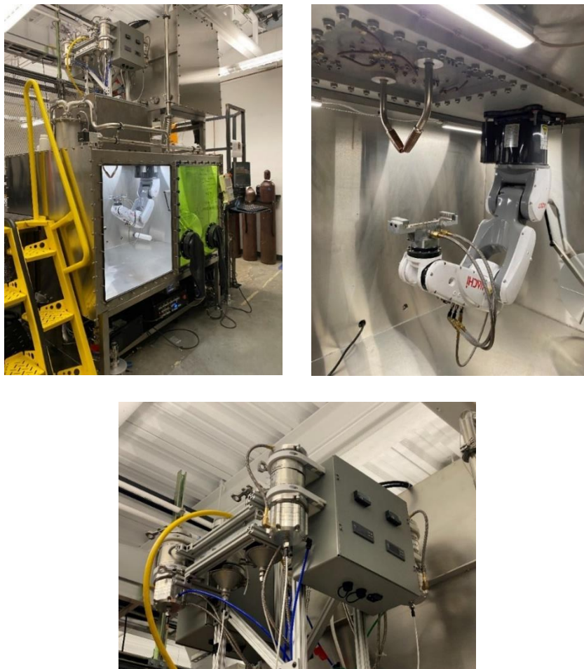
Figure 2.5 The NSF Cell Used in Stage 2 Equipped with One 2000 W Diode Laser Driving a 2 mm Diameter Laser Beam and One 100 W Pulse Laser, As Well As Six Powder Feeders, Each for one Specific Type of Powder and With Six Individual Process Heads with Individual Water-cooled Shielding Nozzles to Each Feeder. One Six-degree of Freedom Nachi Robot for Jogging. The Process Environment is Enclosed in a Big Glove Box to Prevent Samples Being Oxidized During the Manufacturing Process.
