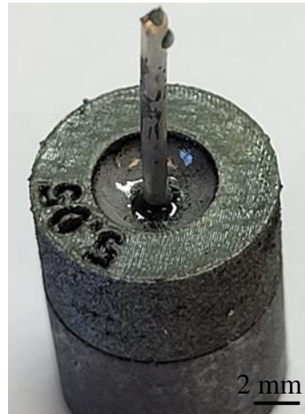
Figure 17: Hermetic ingle pin seal produced with a DLP printed glass preforms, an SLM printed 304L shell, and an Alloy-52 pin.
