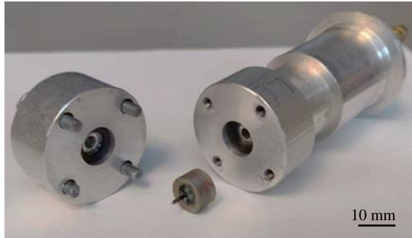
Figure A.1: Image of the custom fixture used to test seals hermeticity.
