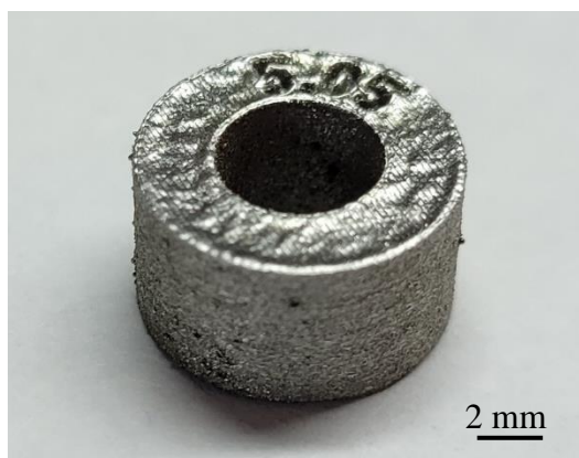
Figure 4: Image of an as-printed 304L stainless steel shell after removal from the SLM build plate by EDM.
