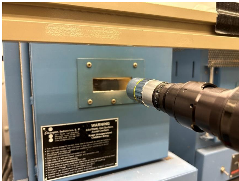
Figure 6: Image of a camera setup for the measuring the cross-section of sintering preforms.
