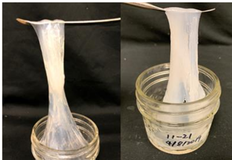
Figure 5.6 Thermal Effect on F-RPPG. 1. Newly re-assembled gel; 2. Gel after 1-year aged in a 65°C oven
