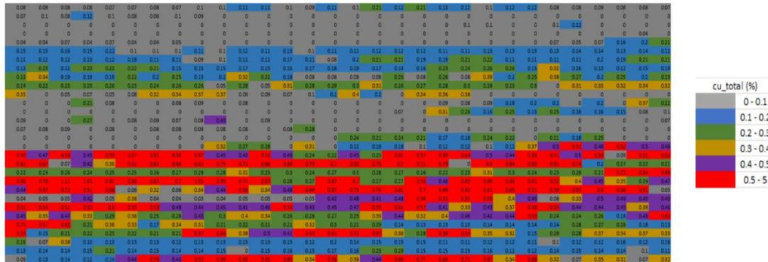
Figure 4.3 Copper Grade of Blocks of 30×30 Bench Section
