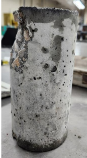
Figure 5.14 Cylinder Broken Once
