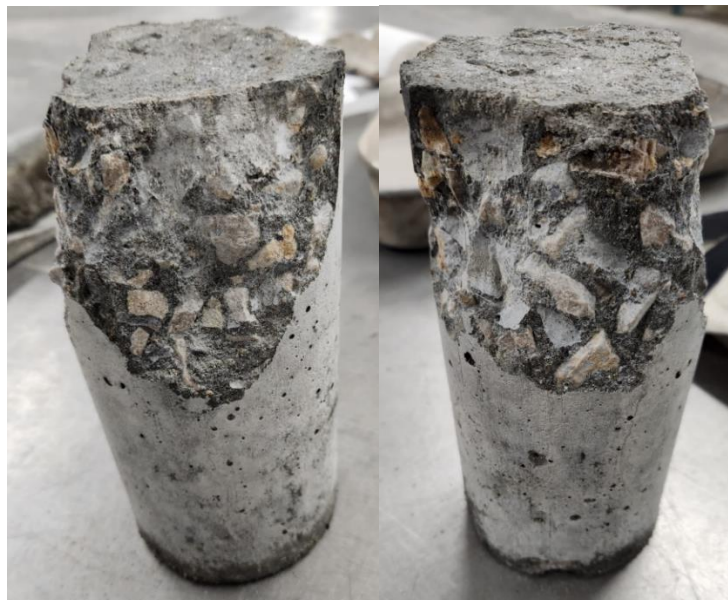
Figure 5.15 Cylinder Broken Twice
