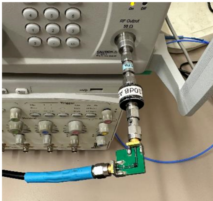
Figure 3.5. Diode Characterization Setup
