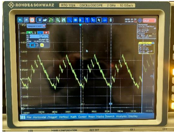
Figure 4.11. Camera Sensor Output Voltage Waveform
