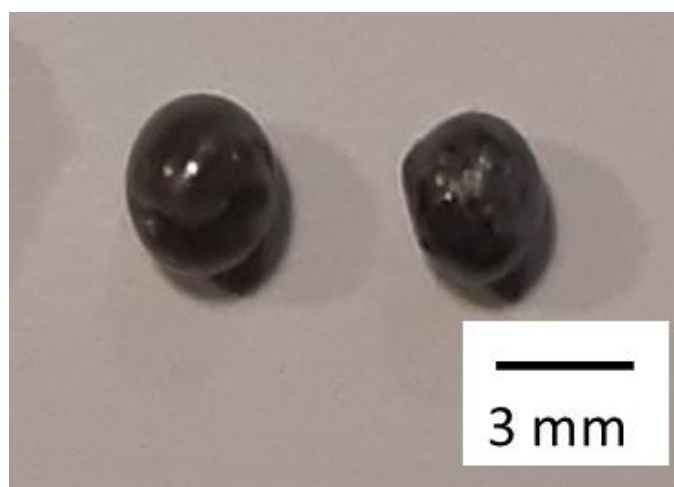
Figure 4: Specimens melted in N_2 at atmospheric pressure (left) and at 10.3 MPa (right) with melted regions visible by the dome structure and unmelted regions noted by non-spherical shapes.
