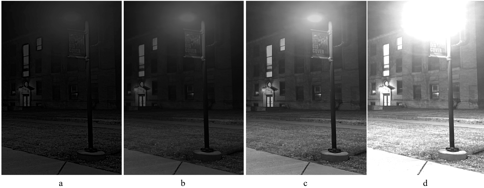
Figure 3.2 Illustrations approximating illuminance orders of magnitude. a) 0.01 fc (0.1 lx). b) 0.1 fc (1 lx). c) 1 fc (~10 lx). d) 10 fc (~100 lx).
