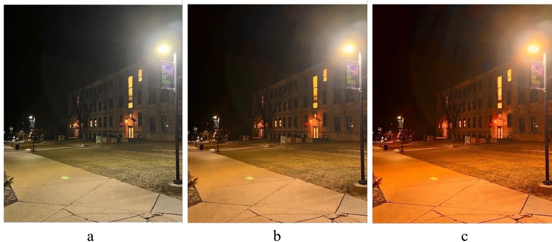
Figure 3.4 Simulated photos for the perception survey. a) 5000K. b) 2700K. c) 1800K.
