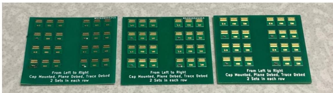
Figure 7. Manufactured PCBs for Characterization. From left to right, 0.2 mm, 0.4 mm, and 1 mm dielectric thicknesses
