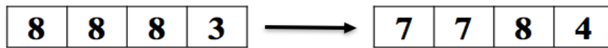
Figure 10. Example of target mutation. Decap #8 mutates to #7, decap #3 mutates into #4. The solution is mutating 'inwards' towards the best decap for a violating point.
