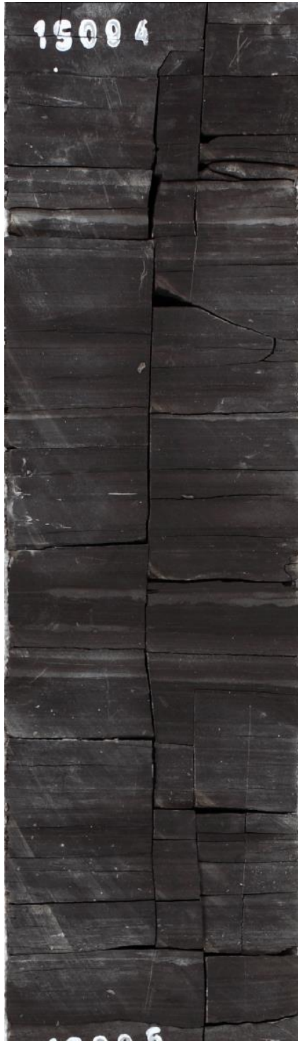
Figure 4.7: Photograph of Core #5 of vertical and horizontal fractures in the TMS.
