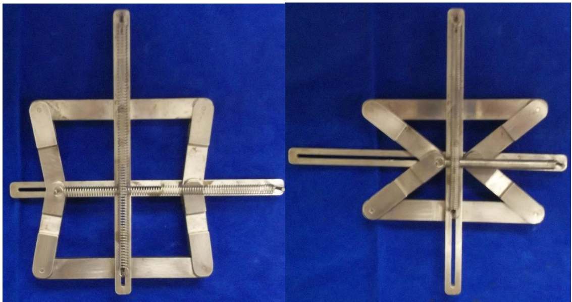
Figure 4.9. Constant-Force 6-Bar Mechanism in Deflected and Undeflected Position
