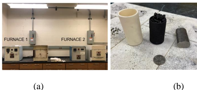
Figure 3.4 Muffle Furnaces (a), MgO Crucible, Glass, and Steel Sample (b) Used in Experiments.
