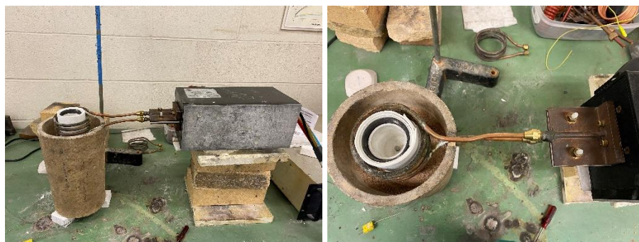
Figure 4.6 Experimental Setup with Ceramic Cylinder Filled with MgO Dry Vibe.
