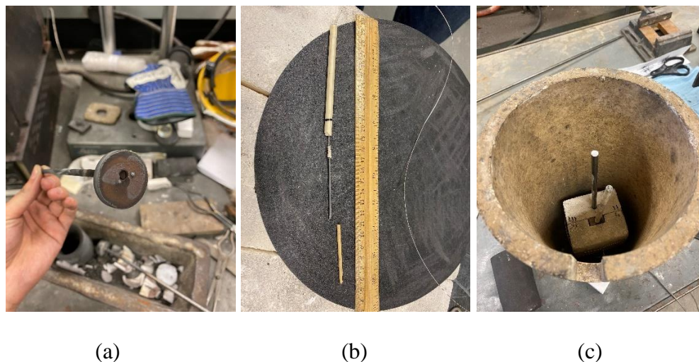
Figure 4.2 Pictures of Graphite (a), \text{ZrB}_2 (b) and Steel (c) Electrodes Used in Experiments.
