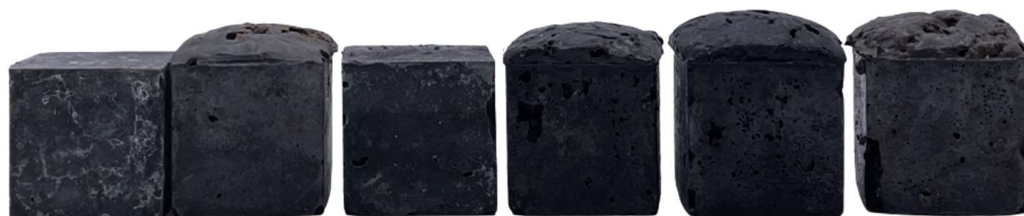
Figure 4.6 Photos of cement pastes incorporating (from left to right): FA, BA, SA, SD, FC, and FD.
