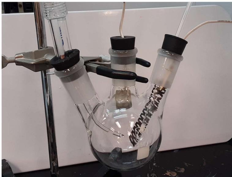
Figure 1. The three-electrode corrosion cell setup. The reference electrode is in the left neck, the working electrode is in the middle neck, and the counter electrode and sparging tube are in the right neck.
