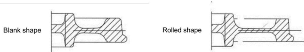
Figure 2.8. Schematic diagram indicating the wheel blank shape prior to wheel rolling, and after wheel rolling. The main difference being a slight reduction in the rim thickness and an elongation in the plate with a slight reduction in web thickness.<sup>34</sup>
