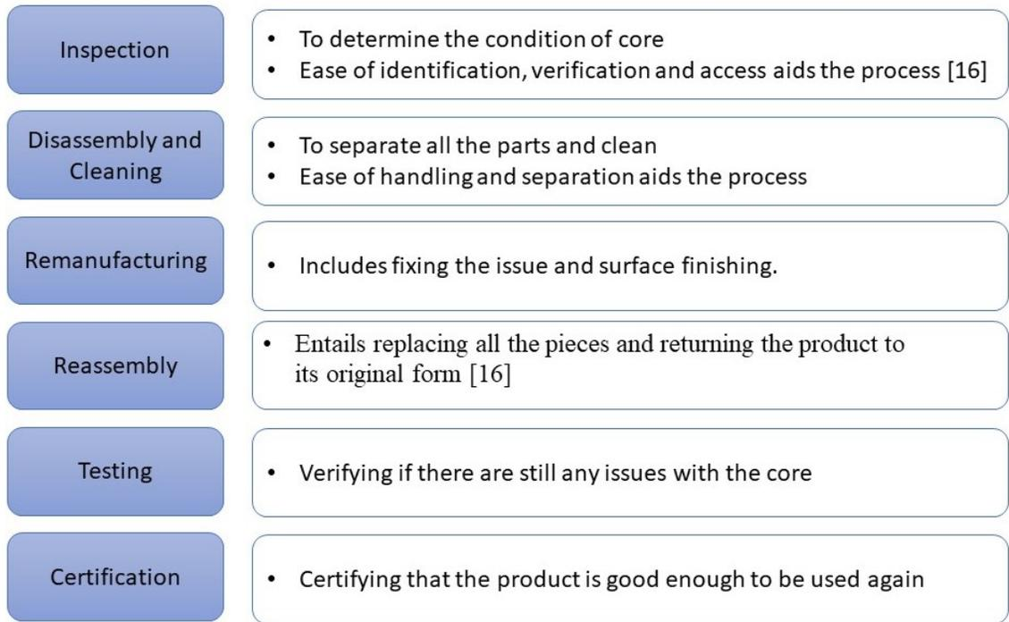
Figure 3.2. The various stages of remanufacturing are depicted and, each step is further discussed in the following paragraph
