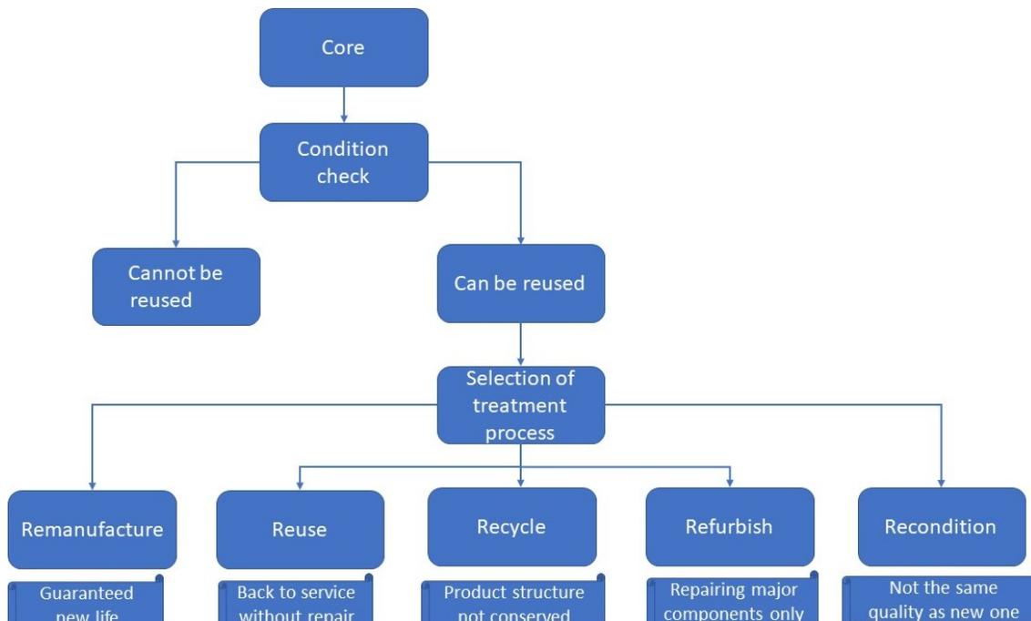
Figure 1.1. The idea behind this illustration is to clarify the misconceptions related to remanufacturing, reuse, recycle, refurbish and recondition
