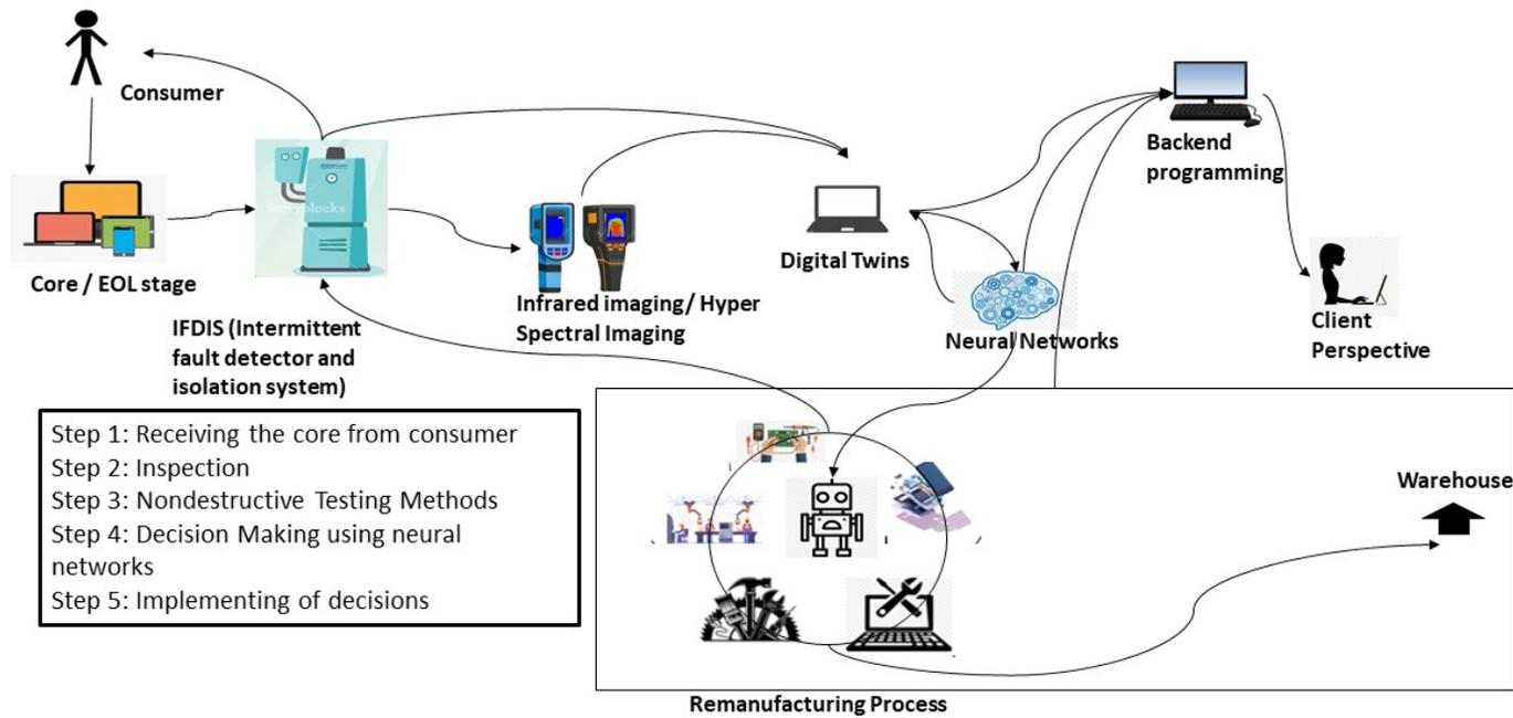
Figure 4.1. This method is believed to be the best feasible possibility of smart remanufacturing electronic devices considering the challenges faced by the current state remanufacturing process
