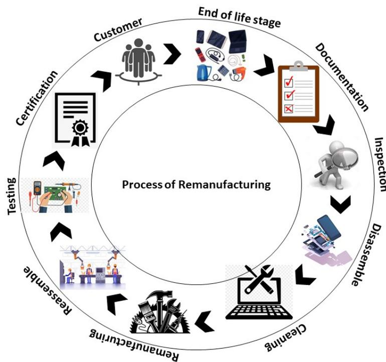
Figure 3.1. Remanufacturing consists of various stages which begins with inspection of the core, disassembling the core, cleaning it, remanufacturing and reprocessing it, reassembling, testing and it is good to be sold to the customer
