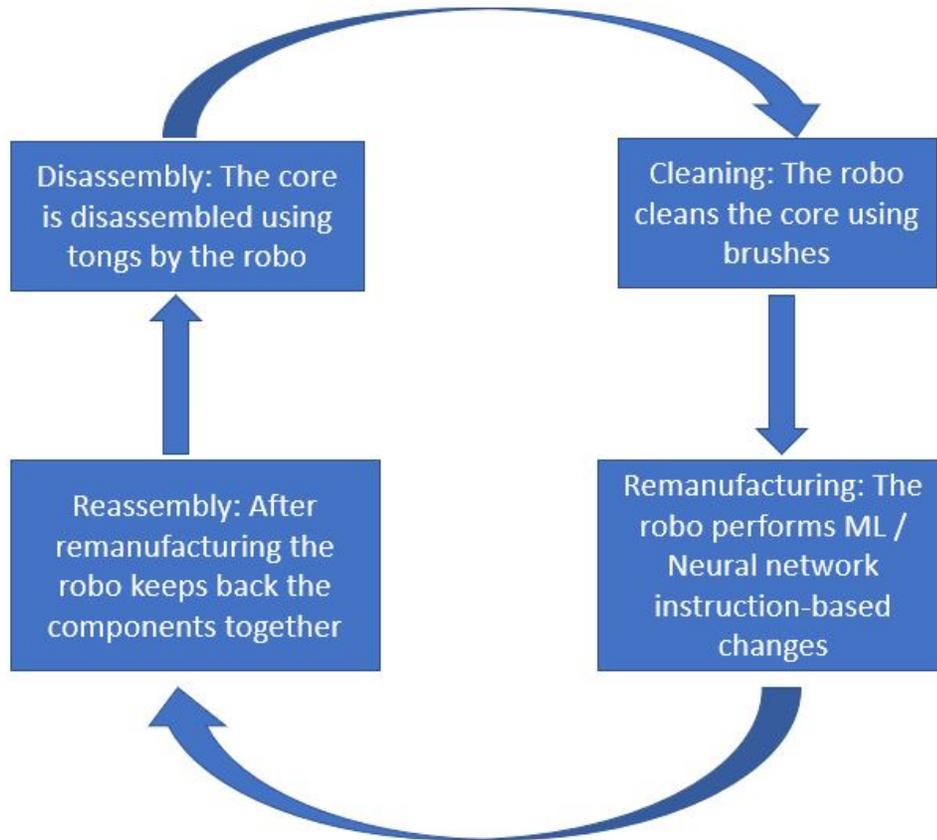
Figure 4.5. The robots are installed in remanufacturing process to make it simpler
