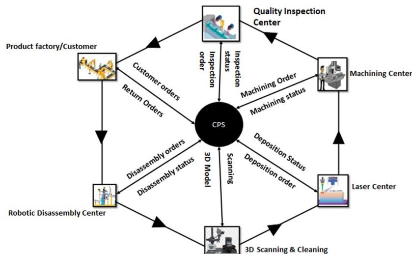
Figure 1.4. The futuristic model of smart remanufacturing is a part of cyber physical system and, all the operations are controlled by a computer.
