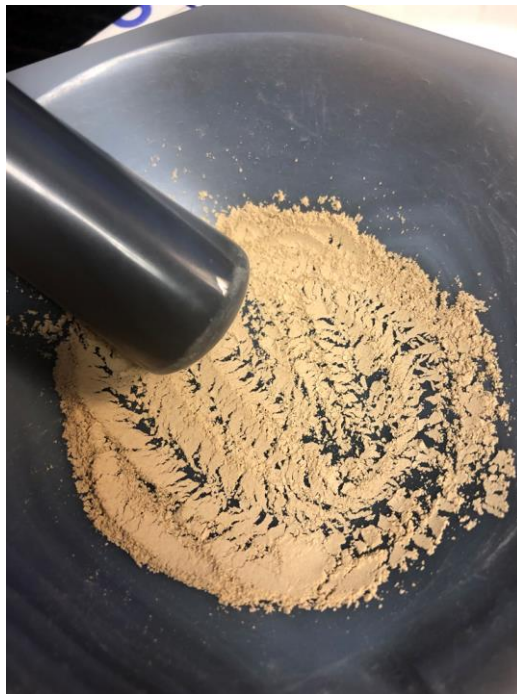
Figure A.45 A Sample After It Has Been Ground Into A Fine Powder.
