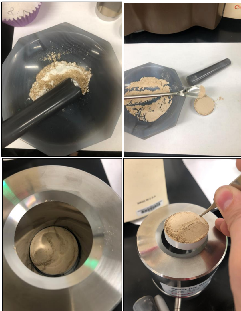
Figure A.46 Steps for Pressing a Sediment Sample Into a Pellet, where a) Mixing of the Sample and Binder, b) Filling of the Pellet Cup, and c) the Loading of the Pellet Cup Into the Press Machine Chassis.
