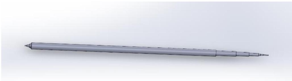
Figure 4.4. Fully Assembled Hyperdermic Assembly
