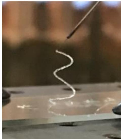
Figure 4.18. Free-Standing Spiral Deposited with Fiber-Fed Process
