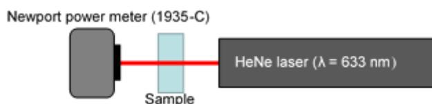
Figure 4.10. Schematic of Transmissivity Measurement Setup
