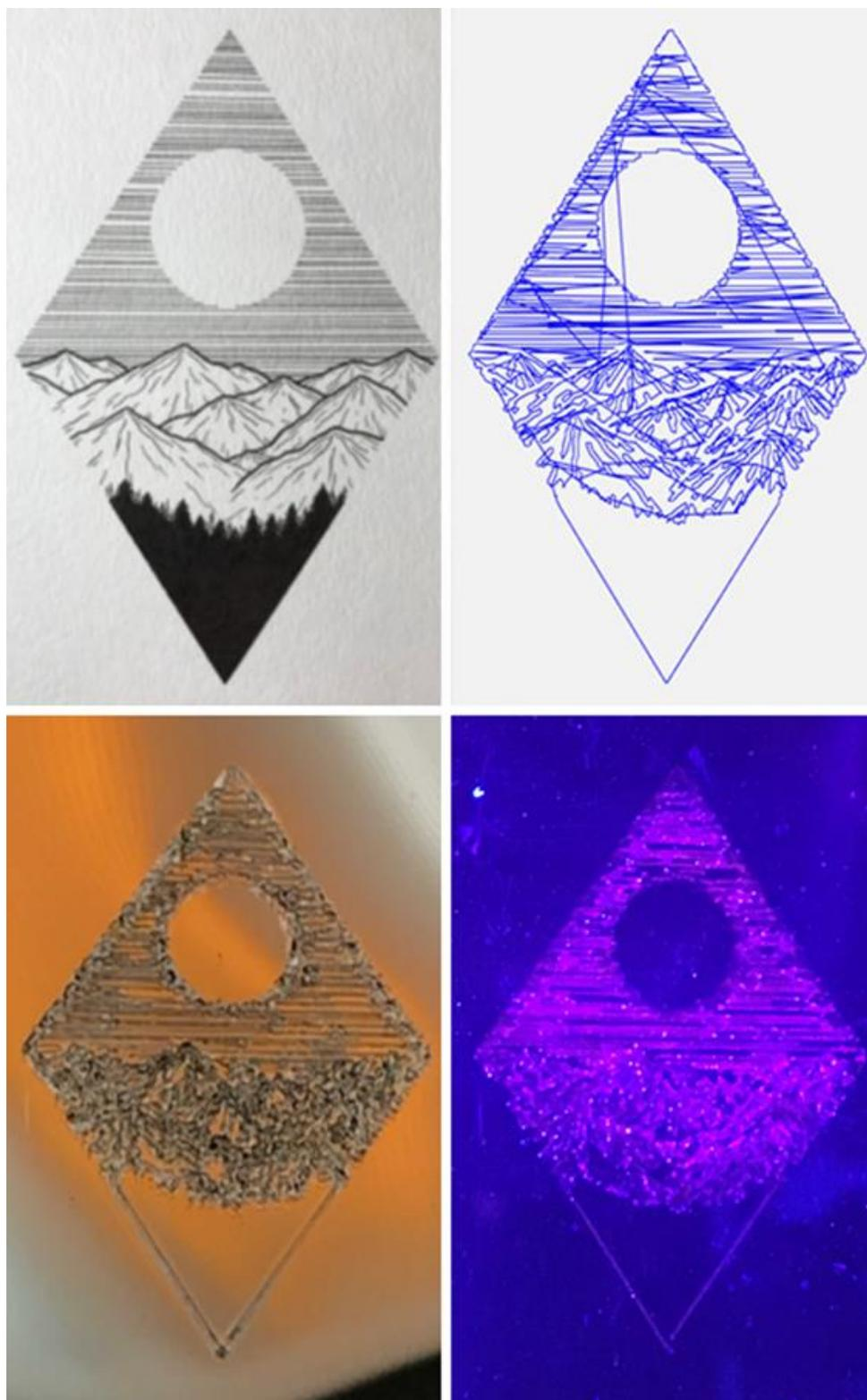
Figure 4.17. Artwork Desired to be Deposited (top left), Path Generated for Deposition (top right), Pattern Post-Deposition (bottom left), Pattern Fluorescing Under  $\lambda = 405$  nm Light (bottom right)
