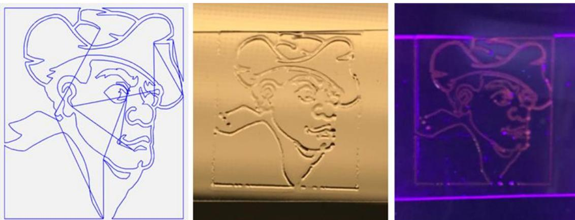
Figure 4.15. Deposition Path Generated for 'Joe Miner' Profile (left), Pattern Post-Deposition (middle), Pattern Fluorescing Under  $\lambda = 405$  nm Light (right)
