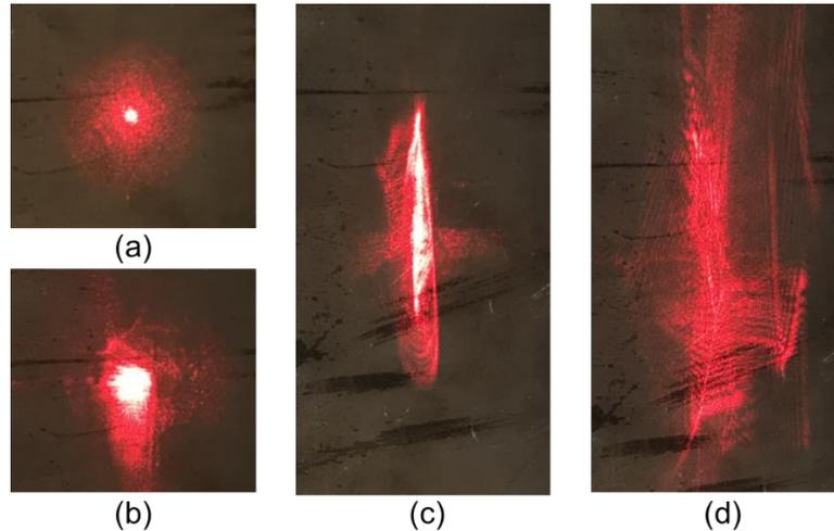
Figure 4.27. HeNe Laser Beam Incident on Wall After Transmission Through: (a) Air, (b) Printed Quartz Block, (c) Quartz Wall Printed at  $P = 10.8$  W, and (d) Quartz Wall Printed at  $P = 6.6$  W
