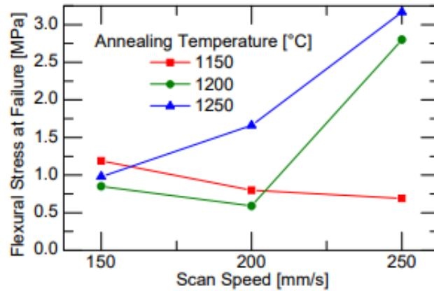
Figure 2.11. Flexural Strength of Silica Deposited at Varying Scan Speeds
