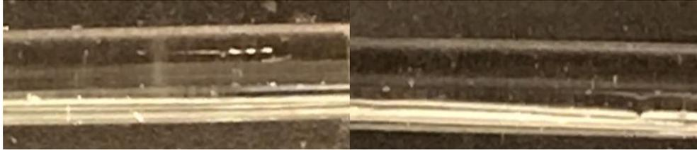
Figure 3.15. Single Track Scans of 2mm Diameter Soda-Lime Filaments with Gaussian Beam (left), Shaped Beam (right)
