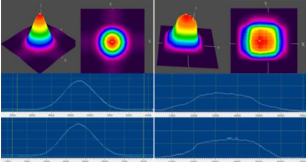
Figure 3.12. Comparison of Unshaped Beam (left), Shaped Beam (right)
