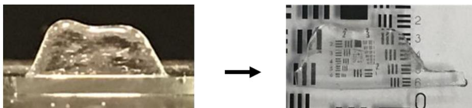
Figure 4.9. 2D Wall Post-Deposition (left), After Polishing to Create Transmissivity Sample (right)
