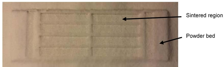
Figure 2.3. Powder Bed Showing Recessed Sintered Regions
