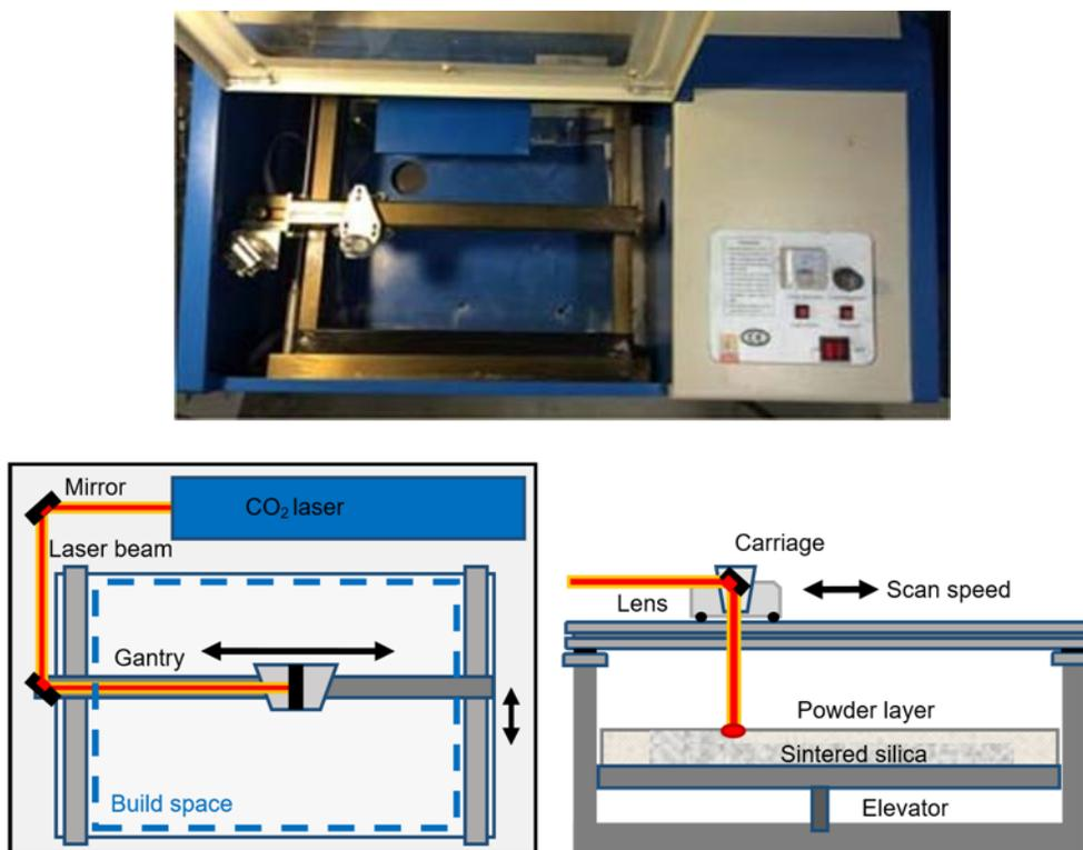
Figure 2.1. Experimental SLS Platform (top) Powder Bed AM Technique Diagram (bottom)
