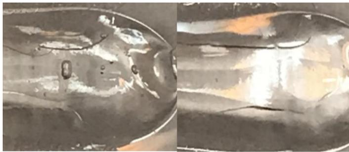
Figure 3.16. Borosilicate Track Scanned with Gaussian Beam (left), Quasi-Uniform Intensity Beam (right)
