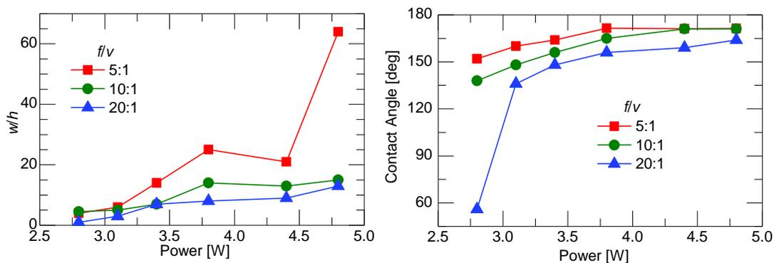
Figure 4.8. Recorded Dimensions of Single Track Morphology as a Function of Process Parameters
