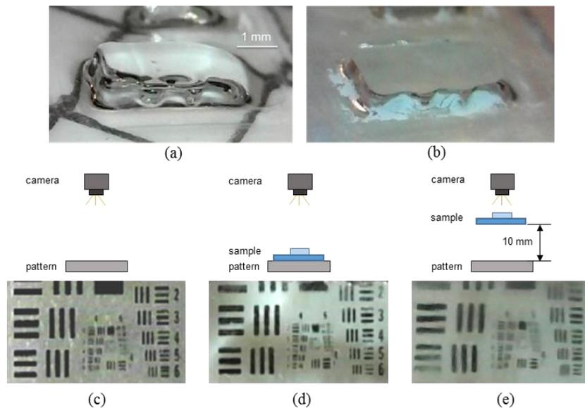
Figure 4.26. Inclusion-Free Block of Quartz Glass ( $3 \times 1 \times 1$  mm) Deposited with Fiber-Fed Approach
