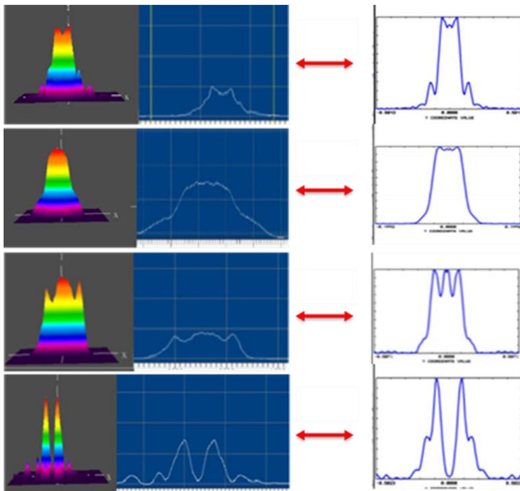
Figure 3.8. Intensity Profiles Measured Away from The Focal Plane (left) Compared to Theoretical [29] Counterparts (right)
