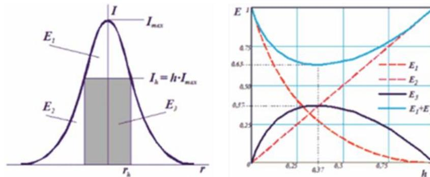
Figure 3.1. Illustration of Energy Lost for Expansion Beam Shaping [22]
