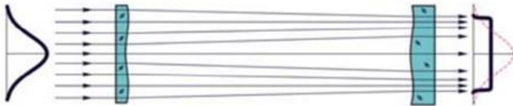
Figure 3.2. Ray Diagram of Uniform Intensity Beam Shaping Optical Element [24]
