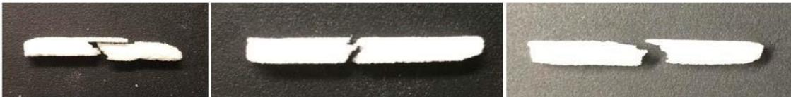
Figure 2.9. Fractured Silica Beams Post Three-Point Bending Test
