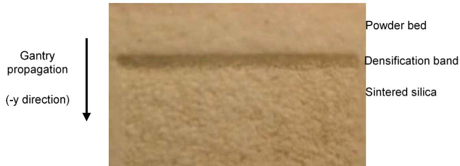
Figure 2.4. Densification Band in The Powder Bed
