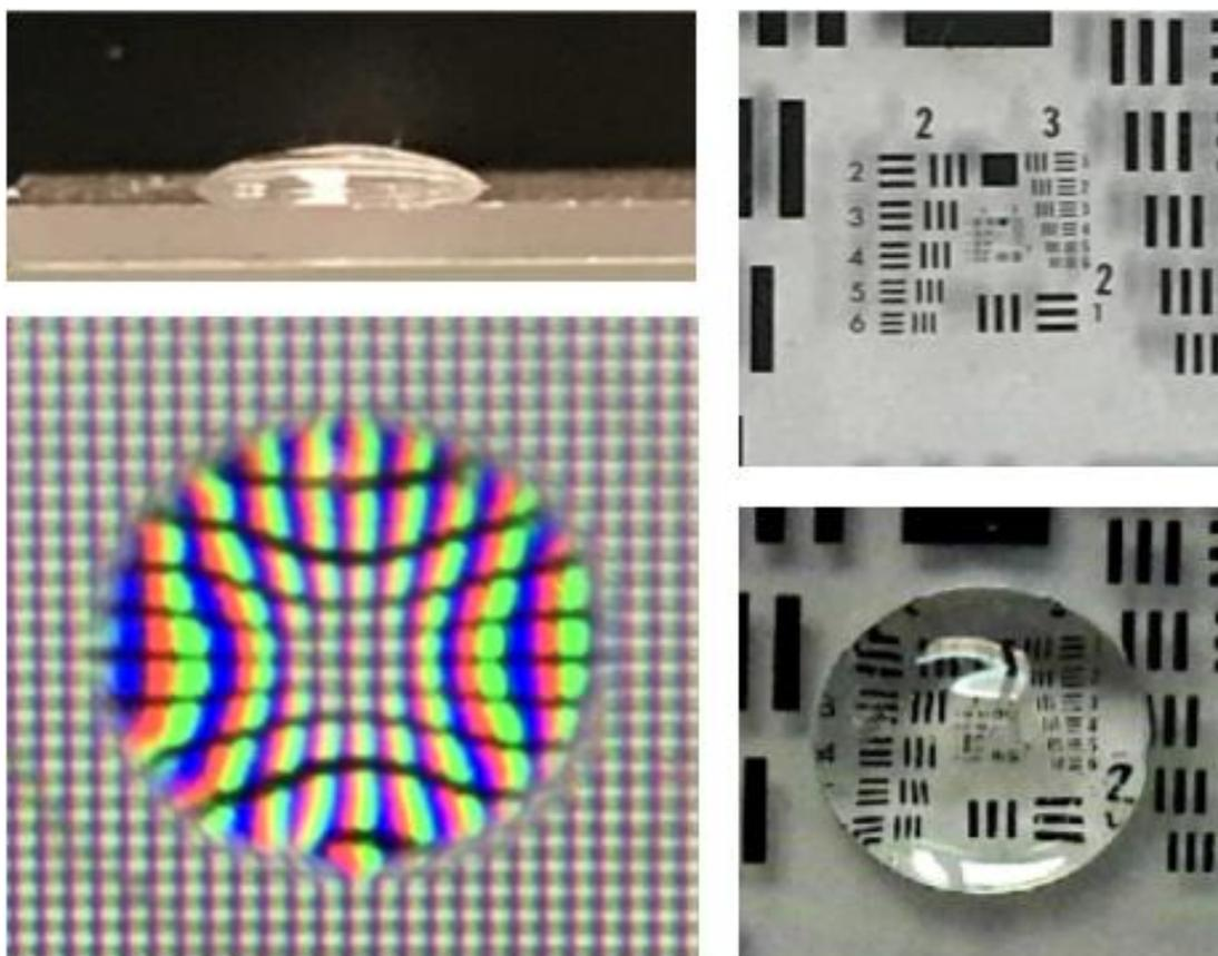
Figure 4.32. Profile of Spherical Lens (top left), Lens Imaging Pixels on LCD Monitor (bottom left), AFRL Resolution Test Chart with No Lens (top right), AFRL Resolution Test Chart Imaged Through Spherical Lens (bottom right)
