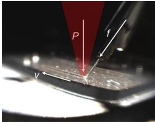
Figure 4.2. Process Parameters for Fiber-Printing Specified for Their Effect on the Deposited Glass
