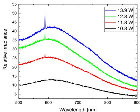
Figure 4.25. Radiation Spectra of Quartz Fiber Melt Pools Around Vaporization Threshold
