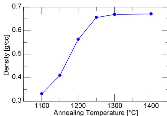
Figure 2.7. Densification Resulting from Annealing Silica Samples
