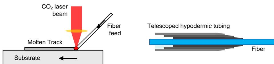
Figure 4.3. Schematic of Telescoping Hypodermic Tubing Used to Prohibit Fiber Deflection
