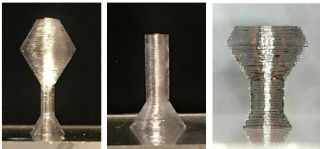
Figure 4.33. Simple Geometries Deposited with Quartz SMF
