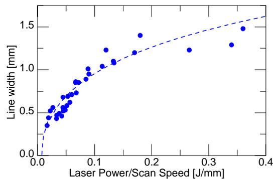
Figure 2.2. Dimensional Excess Associated with Different Ratios of Laser Power to Scan Speed
