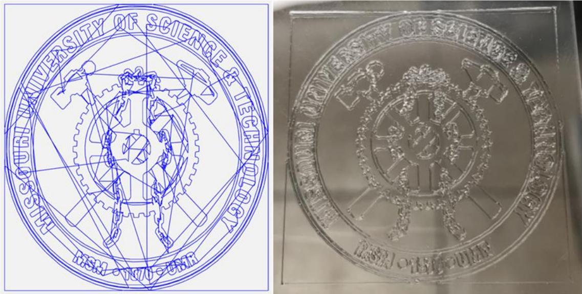
Figure 4.14. Path Generated to Deposit S&T Cog (left) Deposited Soda-Lime S&T Cog Pattern (right)
