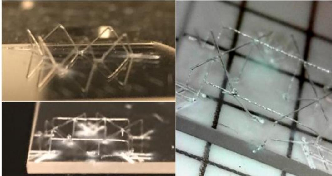
Figure 4.35. Fiber Truss in Various Stages of Deposition
