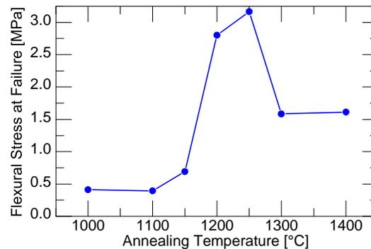
Figure 2.8. Flexural Strength of Silica Samples Annealed at Various Temperatures
