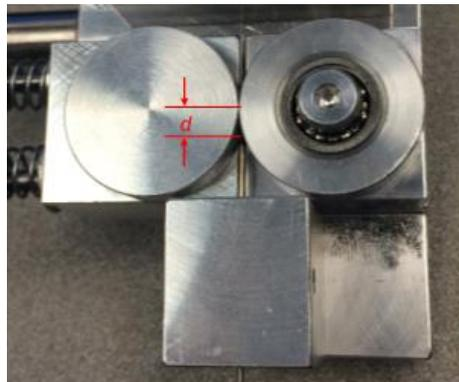
Figure 4.6. Fiber Feeder with Span,  $d$ , Identified as Critical Parameter to Prevent Fiber Buckling
