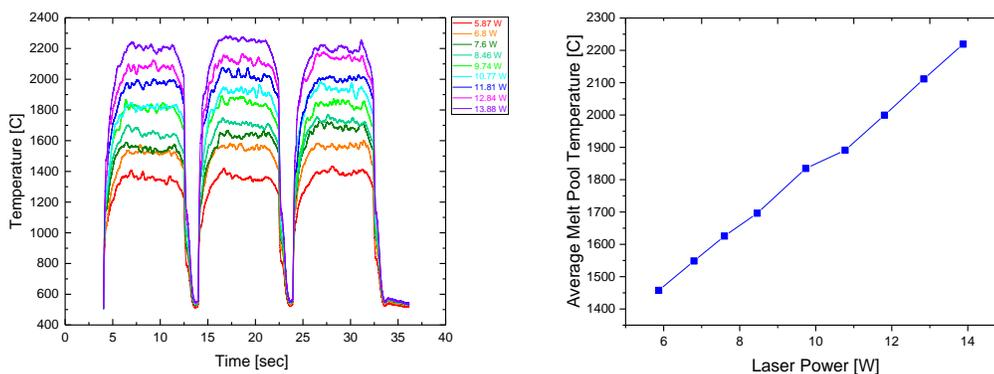
Figure 4.24. Melt Pool Temperature Data Collected During Monolayer Deposition for Various Laser Powers (left), Average Melt Pool Temperature Versus Laser Power (right)
