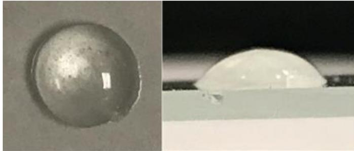
Figure 4.12. Simple Lens Printed with Soda-Lime Fiber Post-Deposition: Top View (left), Side View (right)
