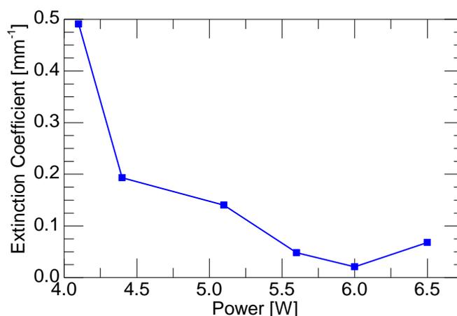
Figure 4.11. Measured Extinction Coefficient of Deposited Fiber Versus Laser Power
