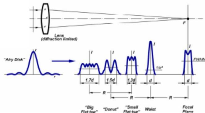
Figure 3.5. Theoretical Intensity Profiles Near Focal Plane [29]
