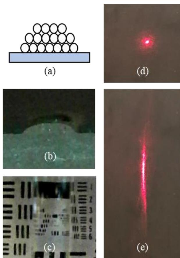
Figure 4.28. (a) Monolayer Patterns Used to Create Cylindrical Profile, (b) Polished Cross-Section of Deposited Cylindrical Lens, (c) Cylindrical Lens Imaging 1951 AFRL Resolution Test Chart, (d) Bare HeNe Laser Beam, (e) HeNe Beam Transmitted Through Cylindrical lens
