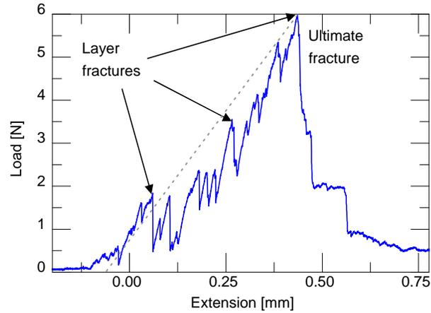
Figure 2.10. Characteristic Load vs. Deflection Experimental Data for Fractured Silica Samples
