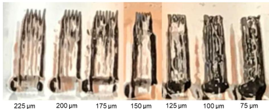
Figure 4.21. Monolayers Deposited with Various Track Spacings
