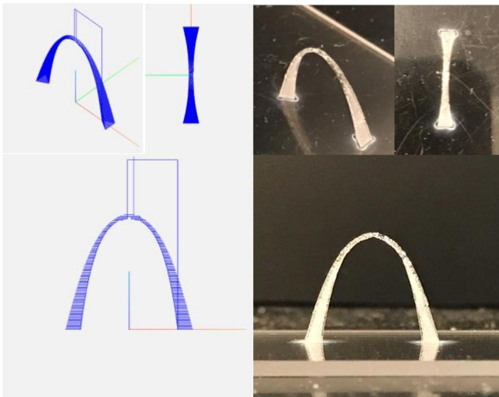
Figure 4.34. St. Louis Gateway Arch Generated Deposition Path (left) Structure Post-Deposition (right)
