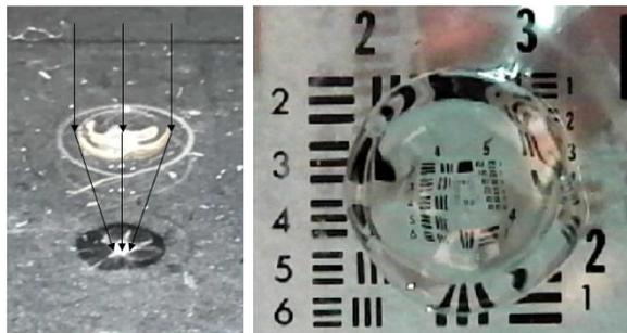
Figure 4.30. Simple Lens Optically Focusing Light (left) Imaging AFRL Resolution Test Chart (right)
