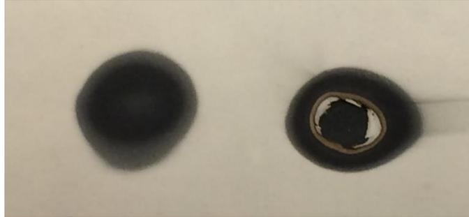
Figure 3.13. Scorch Marks on Photoreactive Beam of Shaped Beam (left), Unshaped Beam (right)
