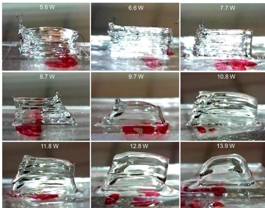
Figure 4.22. Walls Deposited with Quartz Fiber for Transmissivity Measurement
