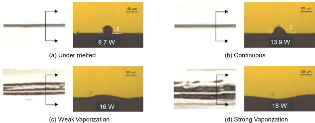
Figure 4.20. Regimes of Single Track Fiber Deposition
