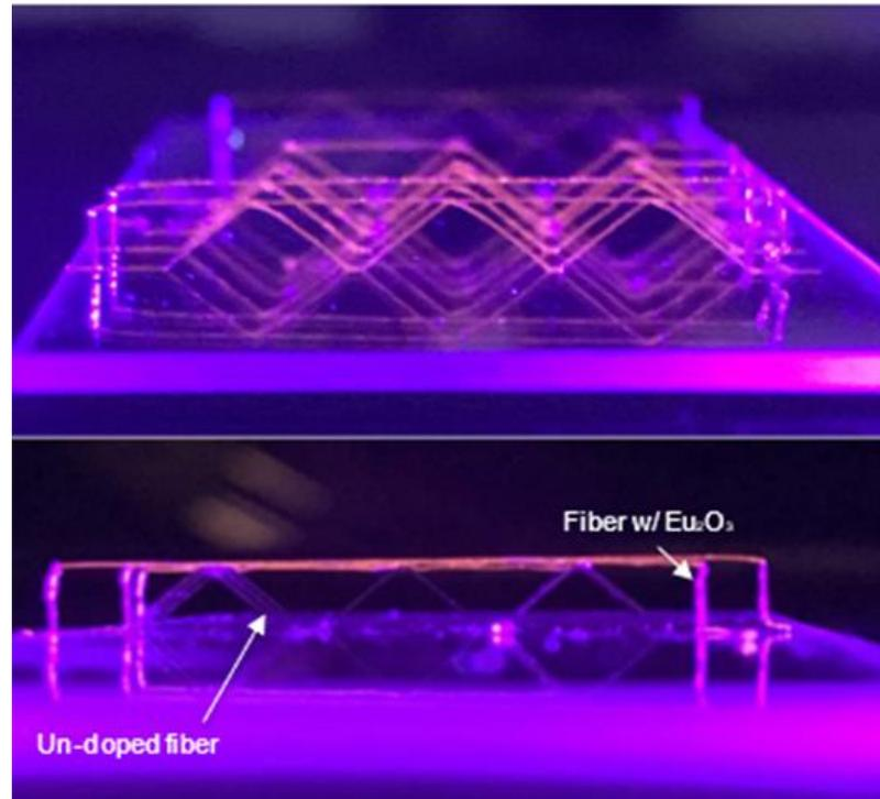
Figure 4.19. A-Frame Truss Walls Deposited Entirely with  $\text{Eu}_2\text{O}_3$  Fiber (top) A-Frame Truss Walls Deposited with Soda-Lime Fiber Both Doped and Un-Doped with  $\text{Eu}_2\text{O}_3$  (bottom)
