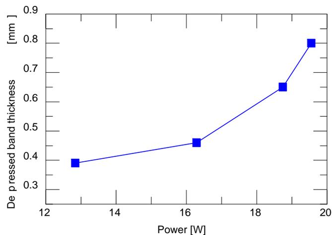
Figure 2.5. Effect of Laser Power on Densification Band Thickness
