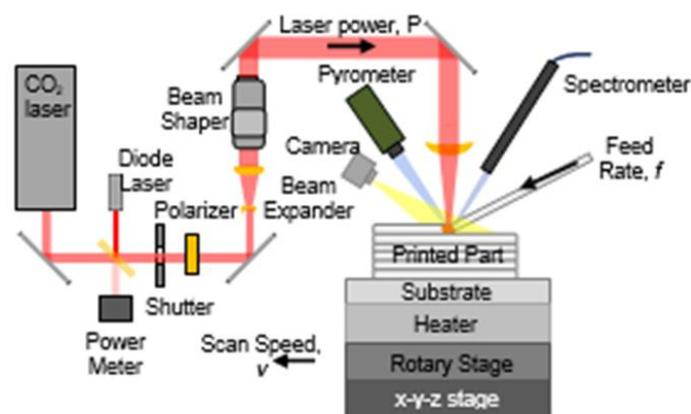
Figure 4.1. Schematic of Experimental Platform
