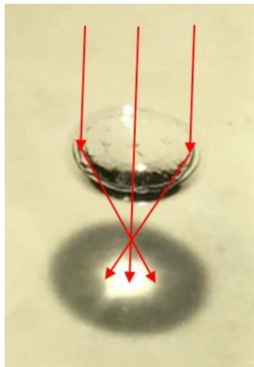
Figure 4.13. Printed Lens Post-Deposition Demonstrating Ability to Focus Light
