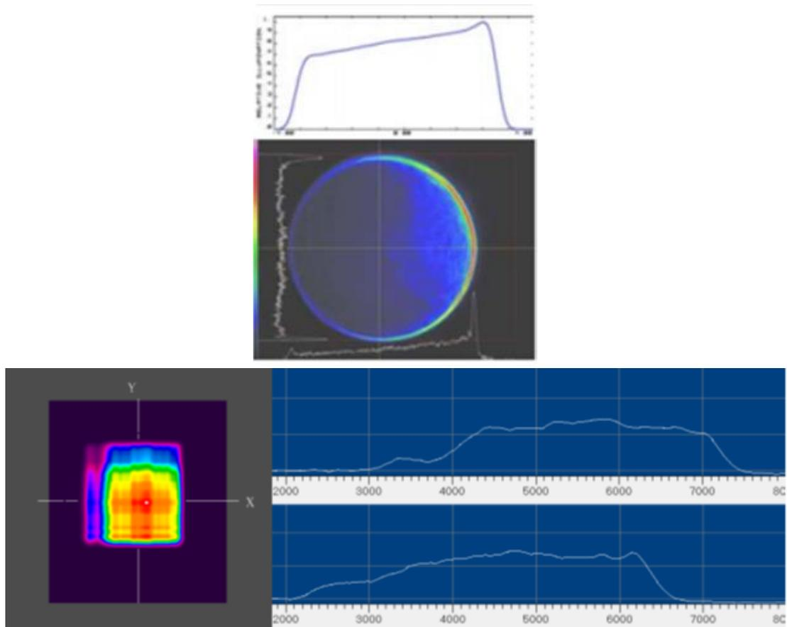
Figure 3.11. Theoretical Model of Intensity Distribution in Beam with Misaligned Beam (top), Experimental Profile of Misaligned Beam (bottom)
