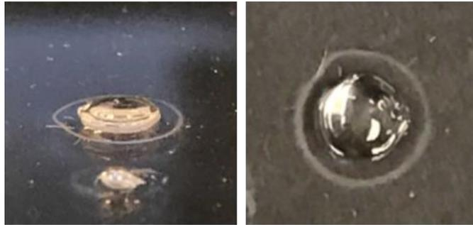
Figure 4.29. Oblique View (left) and Top-Down View (right) of Simple 3D Printed Quartz Lens
