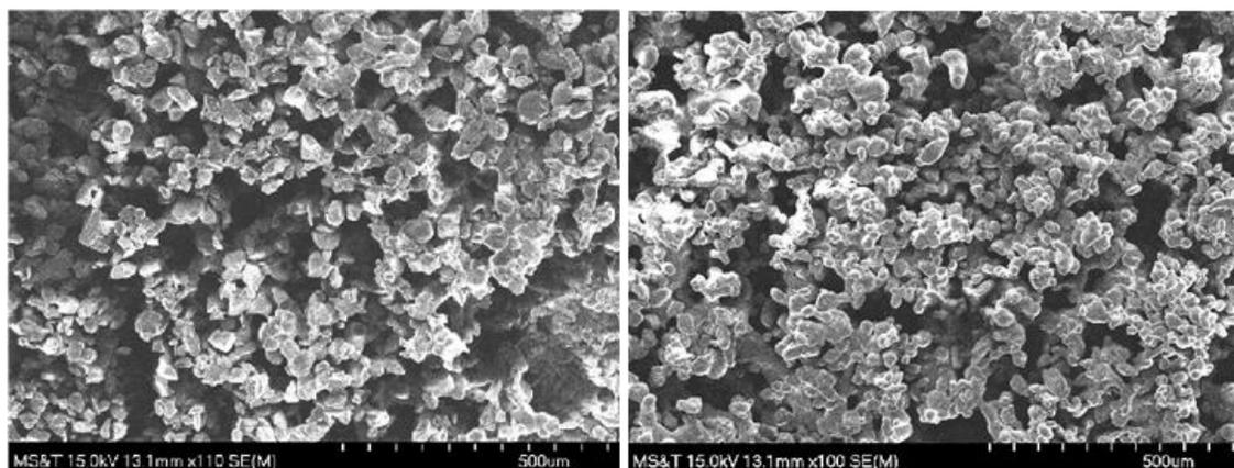
Figure 2.6. SEM Images of Sintered Silica Post-Deposition (left) And Post-Annealing at 1400 °C (right)
