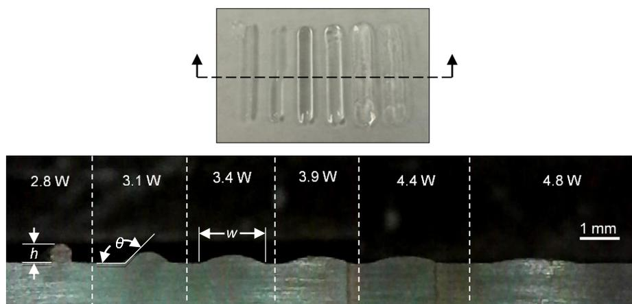
Figure 4.7. Cross Section of Single Tracks with Measured Dimensions Labeled
