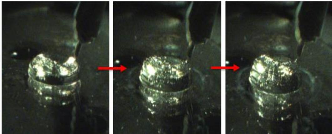
Figure 4.31. Cross-Section of Lens Profile Design (top) Progression of Lens Deposition (bottom)
