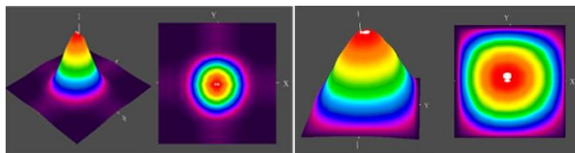
Figure 3.3. Beam Size Before Expansion (left) After Expansion (right)
