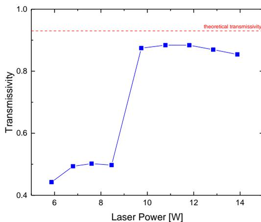
Figure 4.23. Transmissivity of Quartz Walls Deposited at Various Laser Powers
