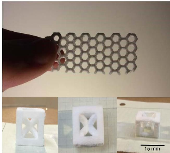
Figure 2.12. Structures Created via SLS Platform (As-Printed)
