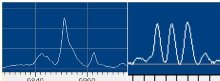
Figure 3.7. Possible Shaped Intensity Profiles: Waist (left), And Flattop (right)
