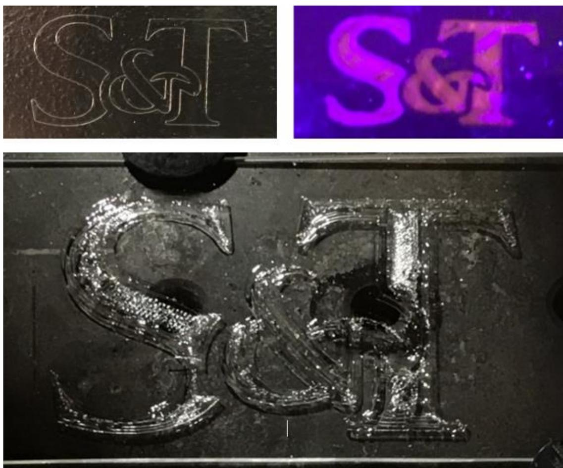
Figure 4.16. S&T Logo Outlined with Fiber (top left) Filled S&T Logo Prior to Reflowing (bottom) S&T Logo Fluorescing Under a Blacklight Post Reflowing (top right)
