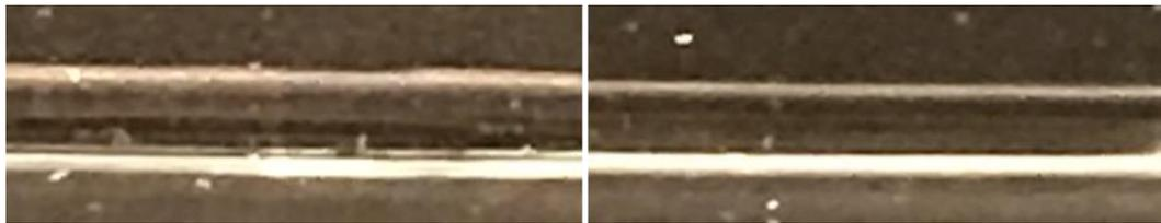
Figure 3.14. Single Track Scans of 1 mm Diameter Soda-Lime Filaments with Gaussian Beam (left), Shaped Beam (right)
