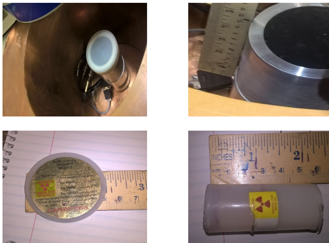
Figure 4.1. Clockwise from top left, end-cap with protective cover, end-cap without protective cover showing carbon window, mixed isotope cylinder with active disk, Europium disk source
