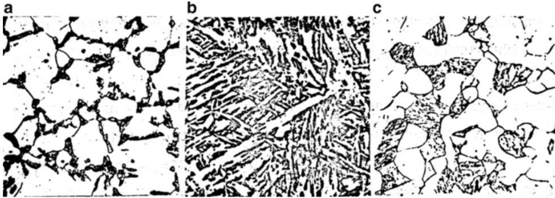
Figure 1.14. Three different types of DP microstructures resulting from different heat treatments of the same chemistry. Dispersed (a) was created by annealing and quenching a cold rolled sample. Acicular (b) was obtained by austenitizing a sample with an acicular ferrite microstructure. Globular (c) was produced by cooling from the austenite region and performing an intercritical isothermal hold [75].
