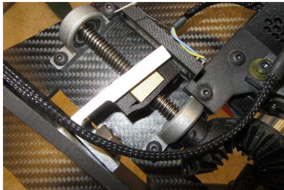
Figure 4.11. Delamination of Onyx Material at Lead Screw Bracket
