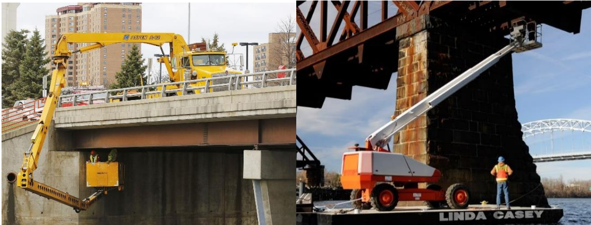
Figure 1.1. Common Aerial Work Platforms: Snooper Truck (left) [5], Boom Lift Secured to Barge (right) [6]
