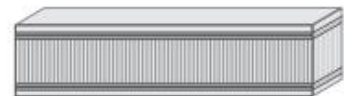
127 layer HSHT Sandwich Beam: (not to scale) 117 layers nylon, 10 layers HSHT Glass CFF (~10% by vol.) Heat Deflection: 140 °C
