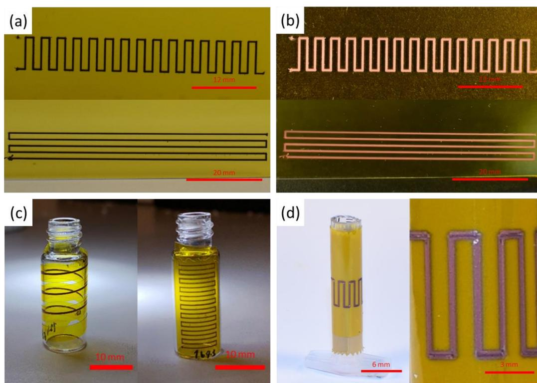
Figure 2. Sintered and unsintered printed patterns: (a) Unsintered planar patterns. (b) Sintered planar patterns. (c) Unsintered non-planar patterns. (d) Sintered non-planar patterns.
