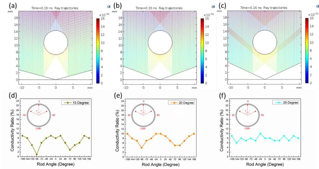
Figure 7. Beam Density results based on angle comparison on non-planar surfaces. (a), (d) 15°, (b), (e) 20°, (c), (f) 25°
