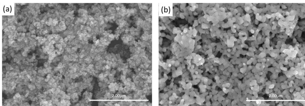
Figure 3. The SEM images of Copper Nanoparticles in different conditions: (a) Before sintering. (b) After sintering.
