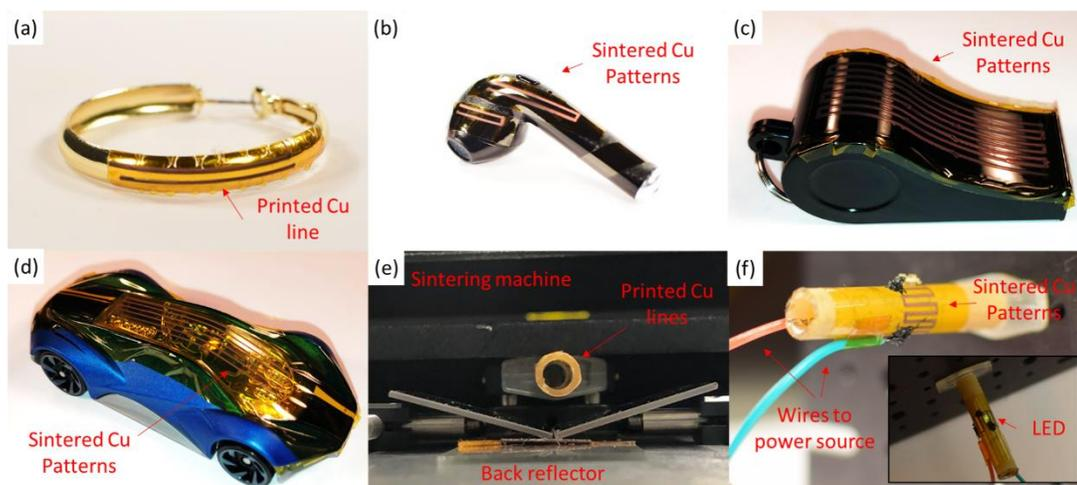
Figure 8. Applications of conductor are demonstrated on non-planar surfaces: (a) Printed lines on a earring. (b) Sintered patterns on a wireless earphone. (c) Sintered patterns on a whistle. (d) Sintered patterns on a toy car. (e) Printed lines on cylindrical rod with back reflector before flash sintering. (f) Cylindrical rod conductors after sintering.
