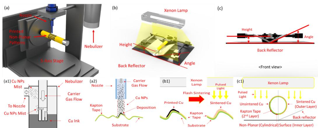
Figure 1. Schematics of non-planar printing and sintering setup with back reflector mirrors: (a) Printed patterns on non-planar surface with aerosol jet printing method. (b) Printed patterns got 3-D sintered under the lamp. (c) The back reflector. (a1) The Cu NPs were nebulized from Cu ink. (a2) The Cu NPs were sprayed from the nozzle. (b1) Sintered Cu after flash sintering. (c1) The application of the back reflector.
