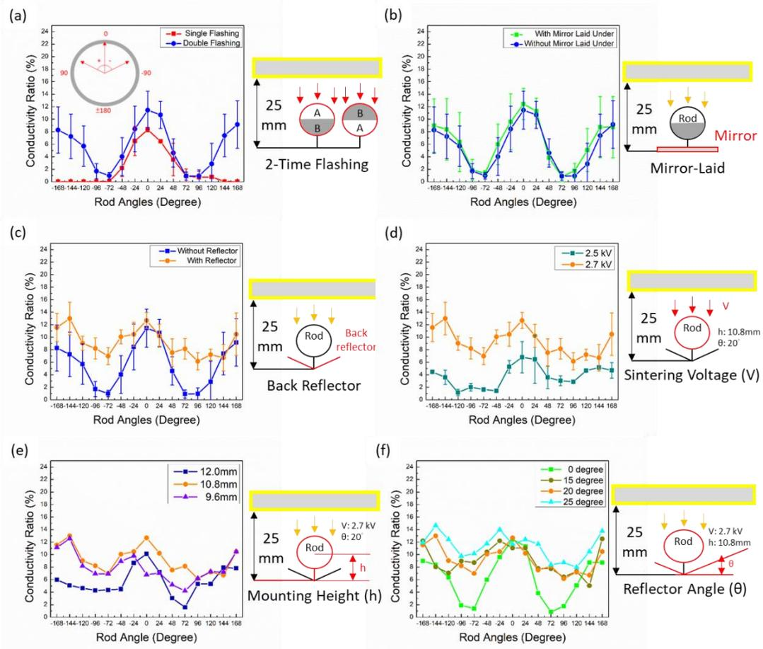
Figure 6. Conductivity results at rod angles based on: (a) Flashing times at 2.7kV. (Second-time is flashing after flipping the rod 180°.) (b) Comparison in horizontal back reflector laid during 2-time sintering. (c) Comparison of the tilted back reflector. (d) Local differences in sintering voltages. (e) Mounting heights. (f) Back reflector angles comparison on non-planar surfaces.
