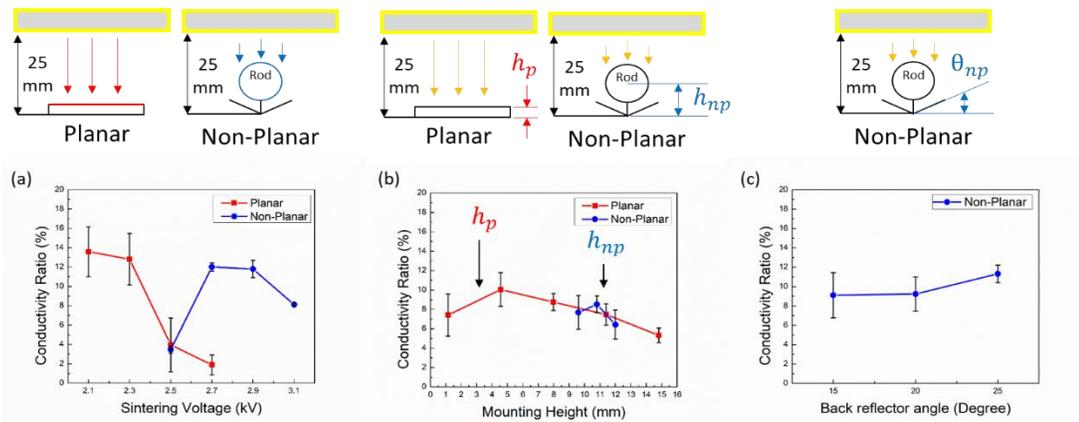
Figure 5. Conductivity results based on: (a) Voltages (V). (b) Heights (h). (c) Back reflector angles ( $\theta$ ).
