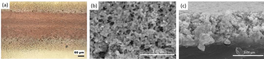
Figure 4. The Microscopic images of non-planar copper layers. (a) Top-view microscopic image. (b) Top-view SEM image. (c) Cross-section SEM images.
