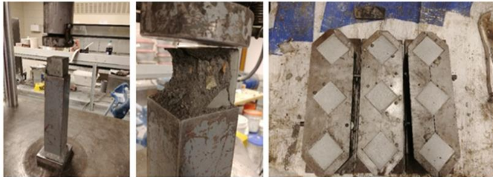
Figure 3.2 Compressive strength test setup
