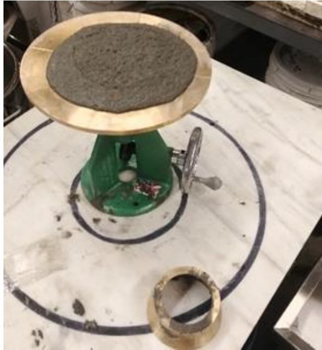
Figure 3.3 Flow table test setup
