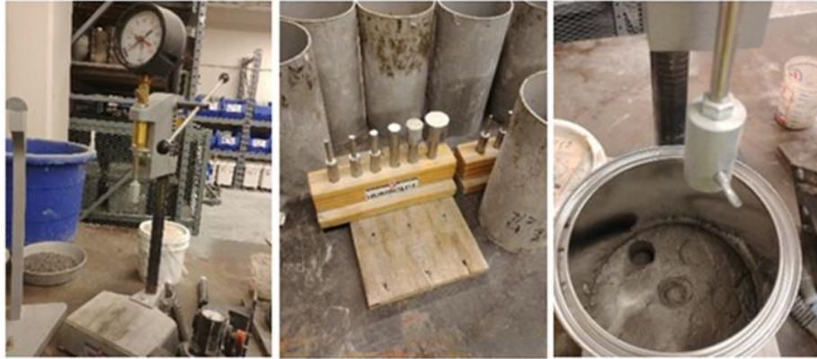
Figure 3.4 Setting time test set up.
