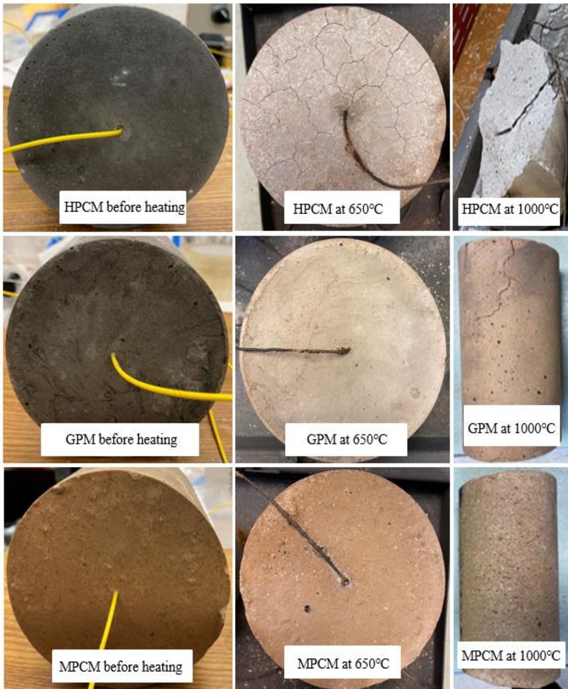
Figure 4.5 Fire resistance. (a) high-temperature monitoring, (b) representative image of cracking. (cont.)
