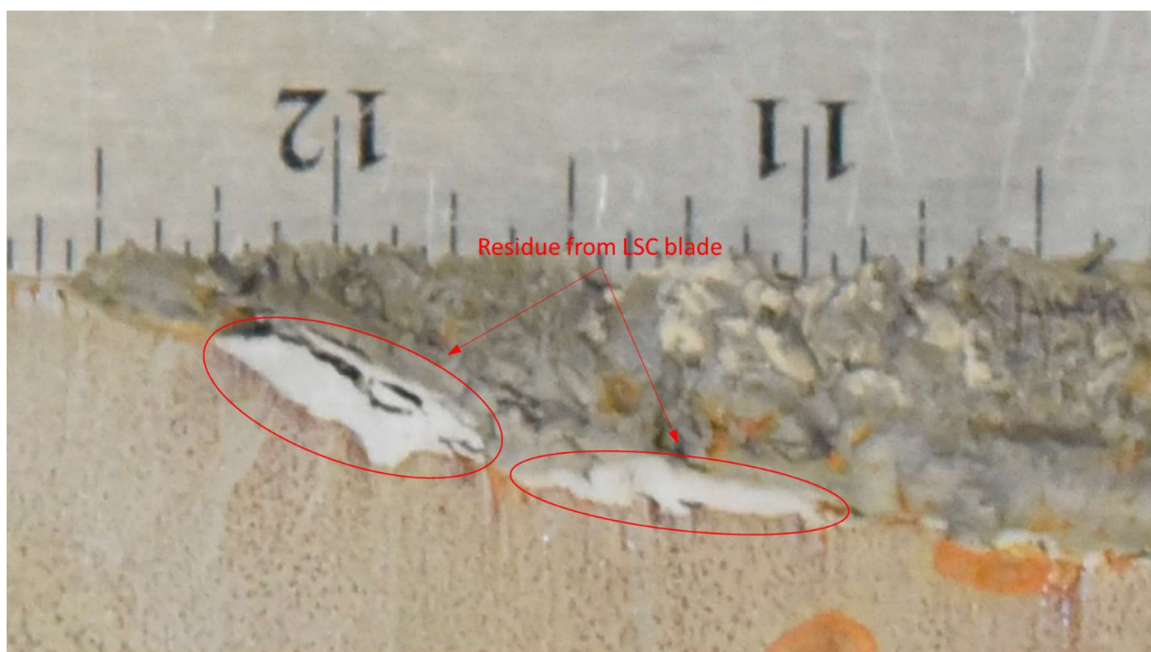
Figure 4.3 Close-up of residue left over from the LSC blade.
