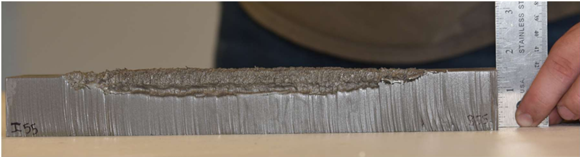
Figure 3.7 Steel target plate cut in half, buffed, and coated to perform analysis on.
