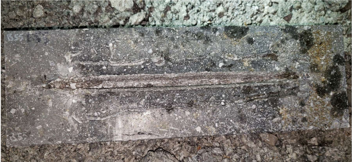
Figure 4.1 Steel target results post-blast from 55° LSC.
