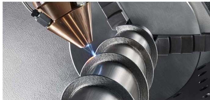
Figure 2.14 Directed energy deposition. [25]
