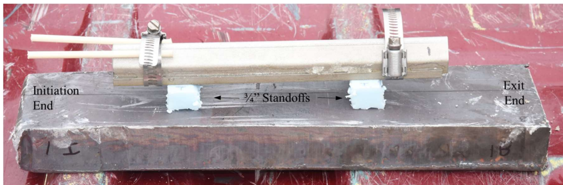
Figure 4.11 Side view of test setup with \frac{3}{4} " standoffs.
