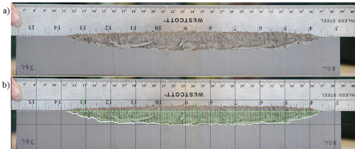
Figure 4.2 Image analysis of penetration depth. a) Image of 70° LSC target. b) Image of 70° LSC target with depth measurement overlay through OMAX LAYOUT.
