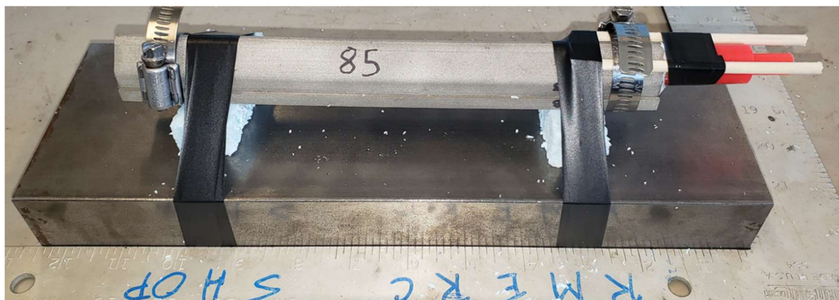
Figure 3.5 Side view of 85° LSC on top of 1 \frac{1}{2} “ steel target. 8g stinger is used to ensure full shock front propagation is achieved. Styrofoam standoffs are \frac{3}{4} ” high.
