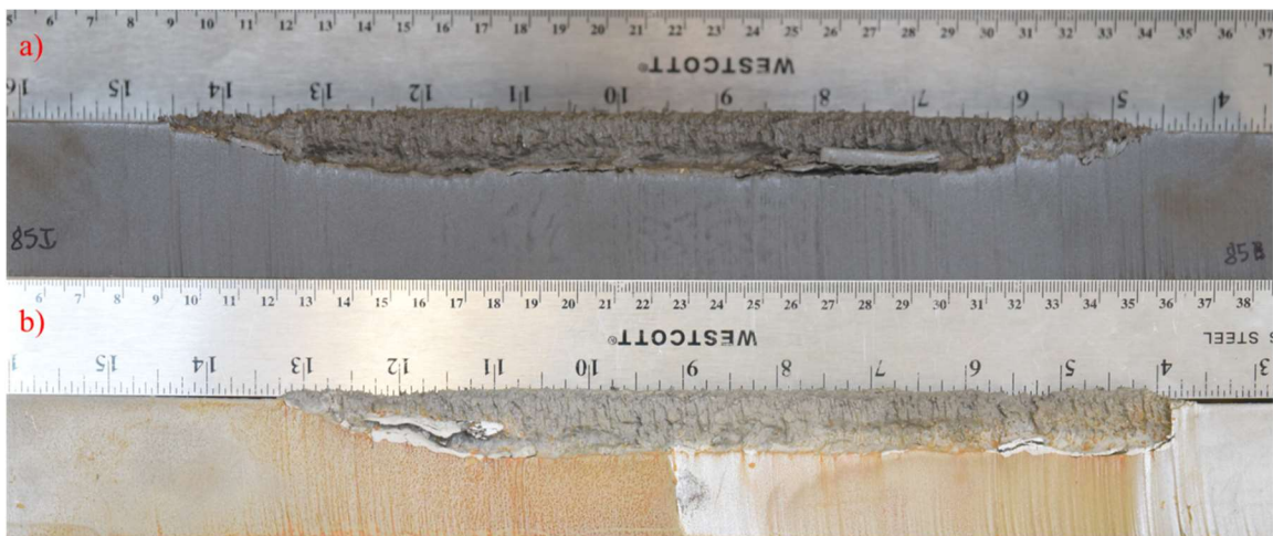
Figure 4.8 Comparison of “Run up” and “Run down” test results. a) Results from 85^\circ apex angle LSC, “Run up” test series. b) Results from 0.14 inch backstop LSC, “Run down” test series.
