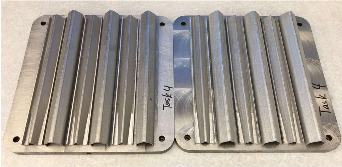
Figure 3.3 Finished linear shaped charge liners on build plate awaiting separation.
