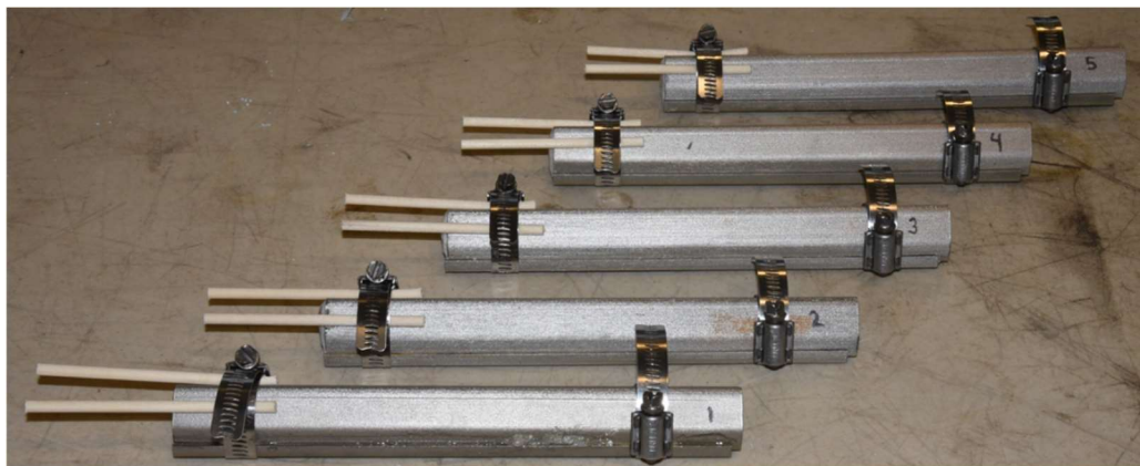
Figure 4.10 Topside view of LSCs. Wooden dowels are attached to help anchor the 8g cast boosters to the LSC charges.
