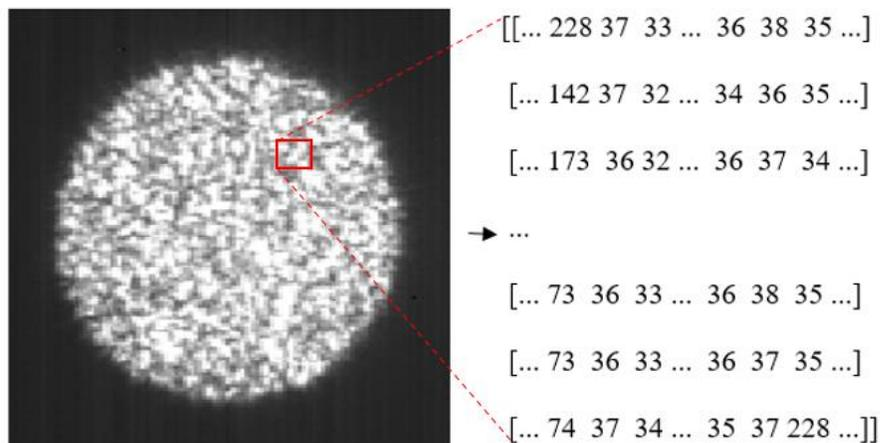
Figure 4.1 Specklegram as a matrix of pixel values.
