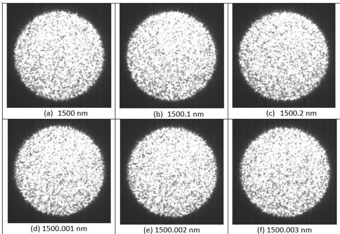
Figure 3.2 Specklegram images (a) – (c) are at a step sizes of 100pm and (d) – (f) at 1 pm.
