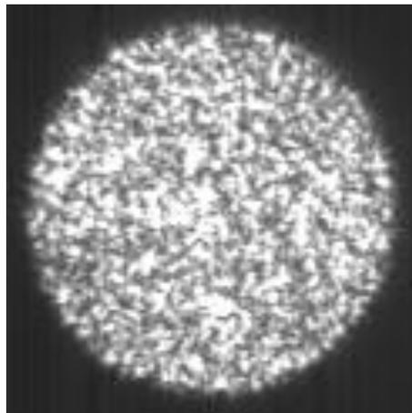
Figure 1.3 A specklegram image at the end facet of a multimode fiber.
