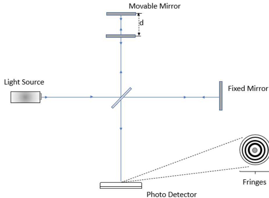
Figure 1.1 Set-up of a Michelson-based Interferometer for Wavelength measurement.
