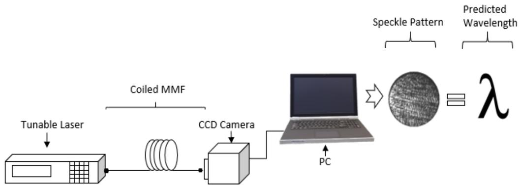
Figure 3.1 Schematic of the Set-up
