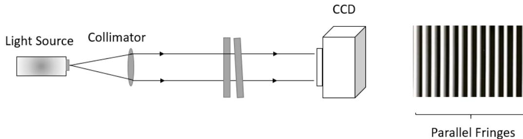
Figure 1.2 Set-up of a Fizeau-based Interferometer for Wavelength measurement.
