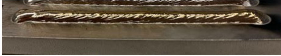
Figure 4.3. Surface defects due to stubbing
