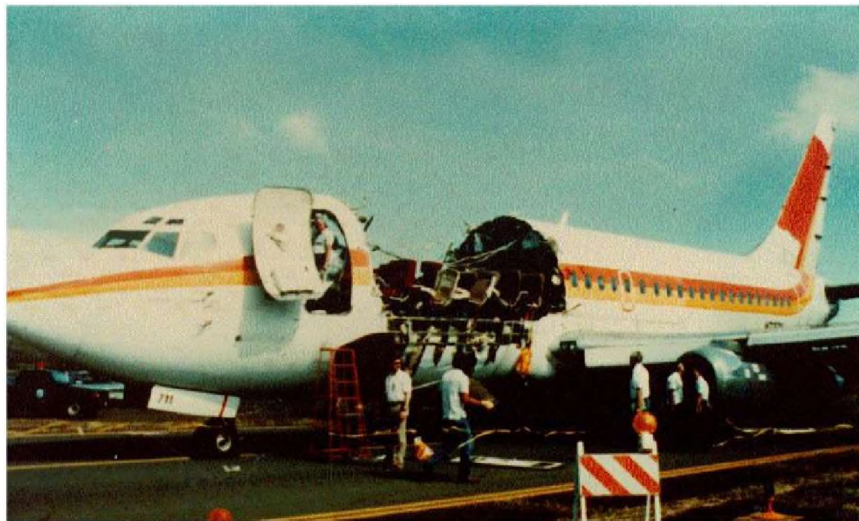
Figure 2-1 B737-200 N73711 Aloha Airlines Fuselage Damage Detail [18].
