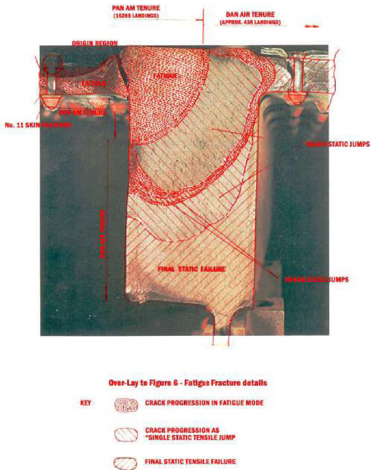
Figure 2-7 Horizontal Stabilizer Spar Chord Fracture Surface [21].
