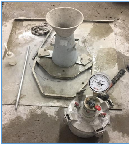
(a) Slump and air meter equipment
