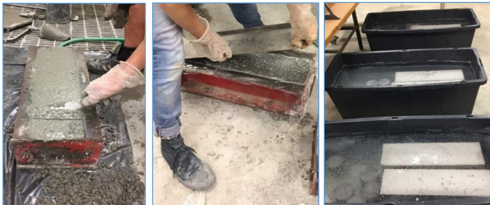
(a) Finishing samples (b) Covering samples (c) Samples curing
