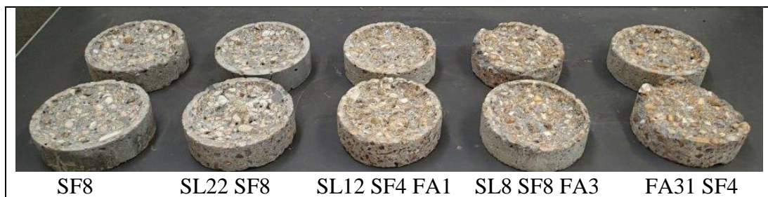
Figure 4.13 Prall samples after testing (Bowthorpe, 2019)
