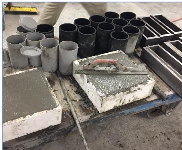
(b) Molds being finished
