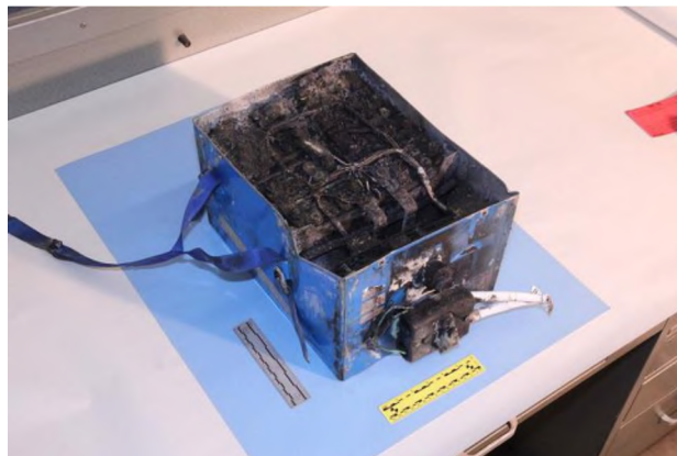
Figure 2. Boeing 787 Li-ion battery explosion [3]
