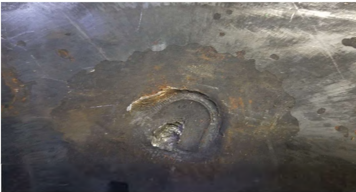
Figure 3.2. Unconfined DetaSheet Plate Dent baseline trial showing the inconsistency in cratering due to chosen loading procedure.
