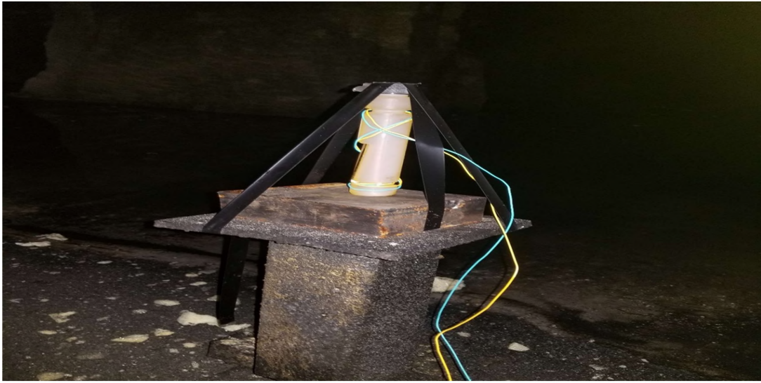
Figure 2.2. Unconfined baseline test for TexPak charge using the fabricated device to protect the load-cell sensor below the blasting site directly.
