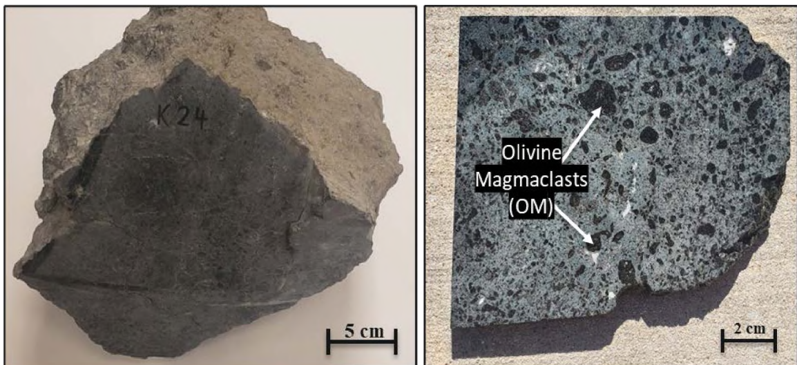
Figure 6: K-24 alnöite sample from the lower diatreme facies. Grey matrix is dominated by subhedral dark-grey olivine domains (magmaclasts) exhibiting porphyritic textures.
