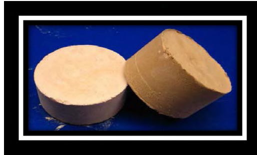
Figure 2.32. High Quality Plugs Formed by Filtration (Wang, 2011)
