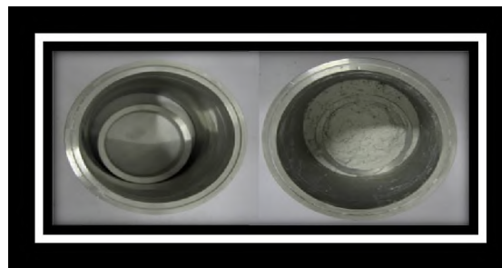
Figure 2.33. Lab Apparatus Showing a Particulate Plug Seal Forming in a Gap that has a varied Size (Wang, 2011)
