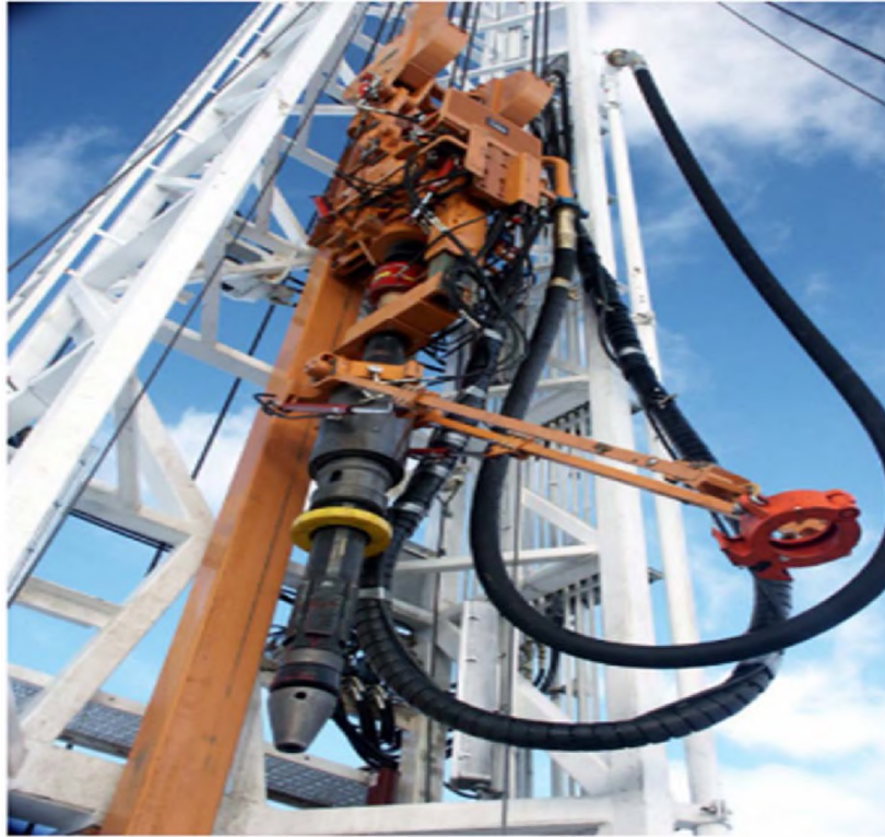
Figure 2.45. Top Drive and Internal Casing Drive (Tessari et al., 2006)
