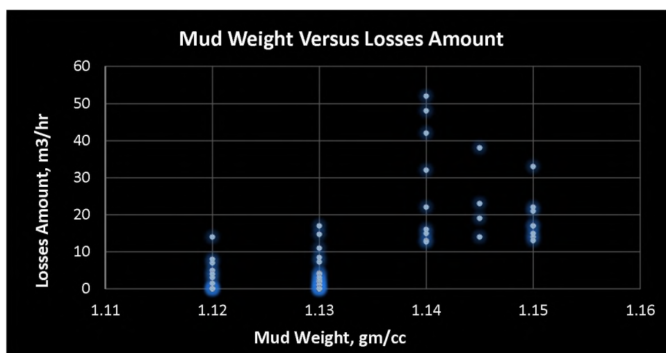
Figure 3.7. Mud Weight versus Losses Amount (Hartha Zone, 50 wells)
