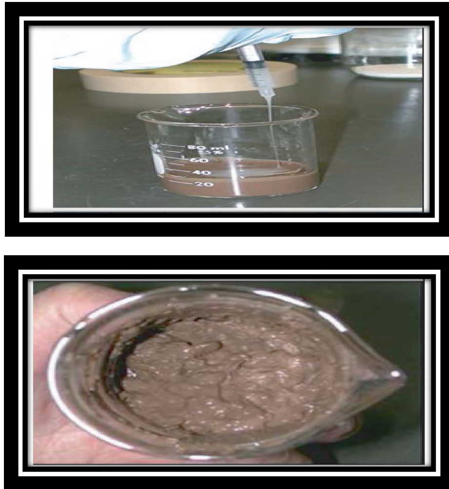
Figure 2.42. The DVC System Reacts with a Water-Based Mud to Form a DVC Sealant. (Wang et al., 2008)
