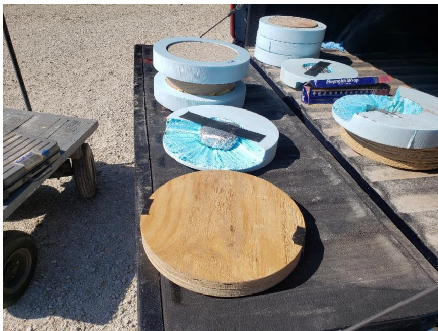
Figure 4.8 Concrete Projectile with Wad and Powder
