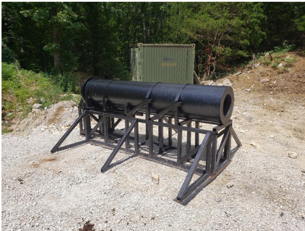
Figure 4.7 Projectile Generator at Test Site
