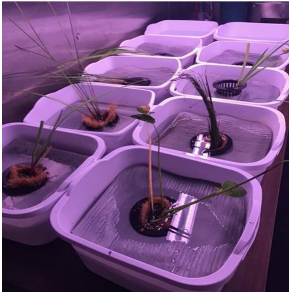
Figure 2.3 Experimental Chambers. Microcosm tubs with floating mat, coconut fiber and emergent macrophyte in hydroponic pot.
