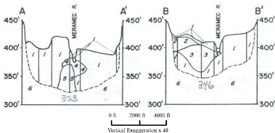
Figure 6.4. Cross-sections A-A' and B-B' oriented looking upstream. Lithology and bedrock depth determined from multiple boreholes obtained throughout the Meramec River Valley (MDNR WR30).
