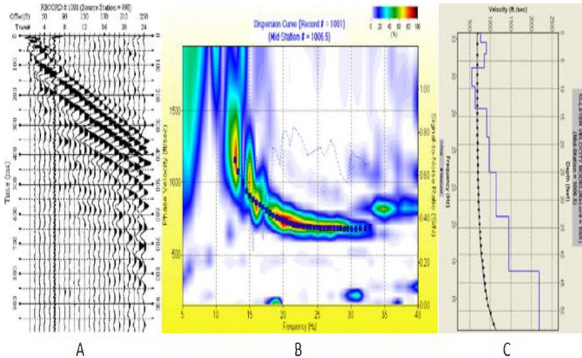
Figure 5.18. Main processing steps using SurfSeis software including: a) a shot gather, b) a picked dispersion curve, and c) 1-D Shear wave velocity profile (Anderson, 2017).
