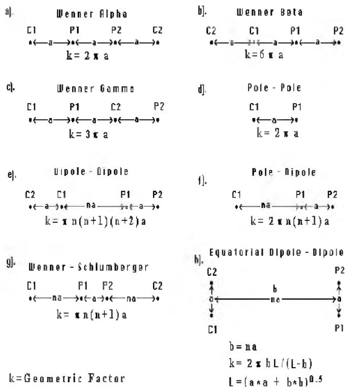
Figure 5.8. Different types of array configurations (Loke, 1999-2016).
