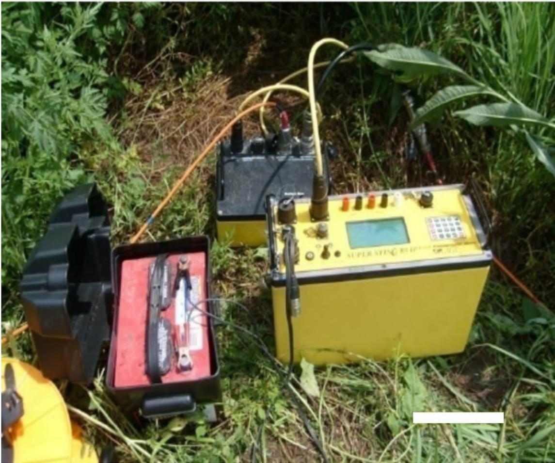
Figure 5.7. The SuperSting R8 unit (right) with 12 volt battery (left) and switchbox (middle) (Ganesh, 2009).
