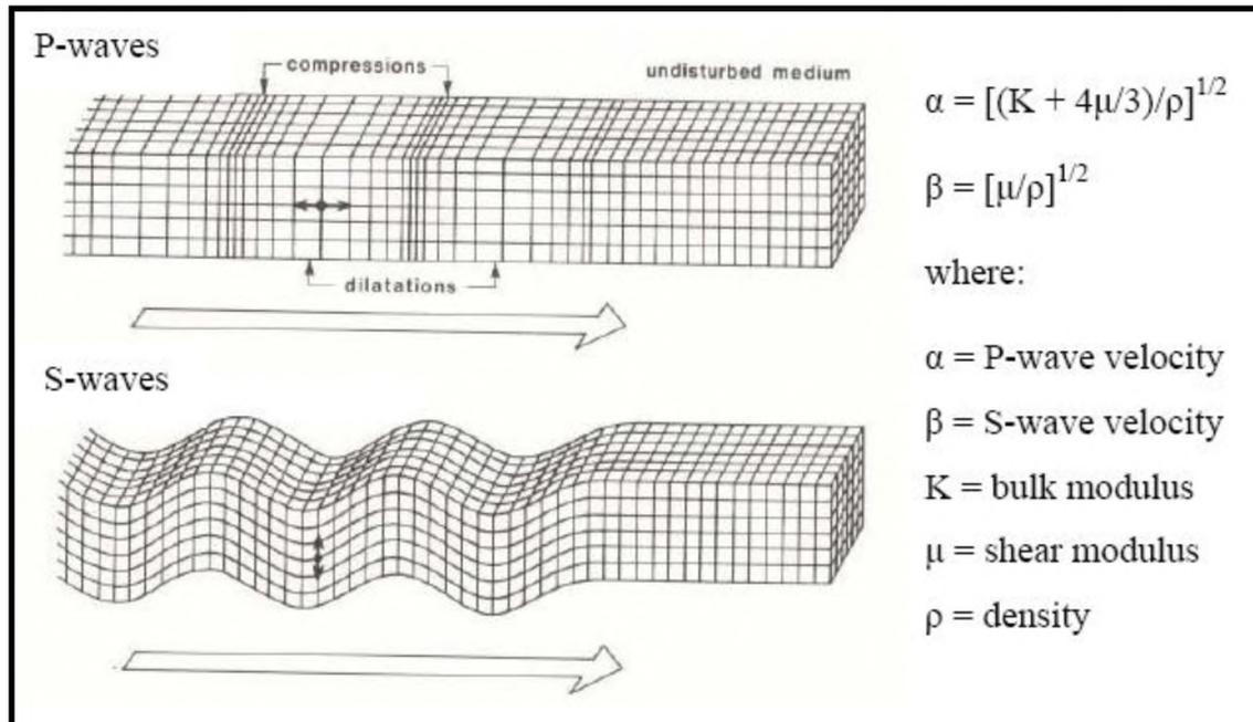
Figure 5.13. Propagation of P-wave and S-wave motion and velocity equations (Thitimakorn and Anderson, 2005).
