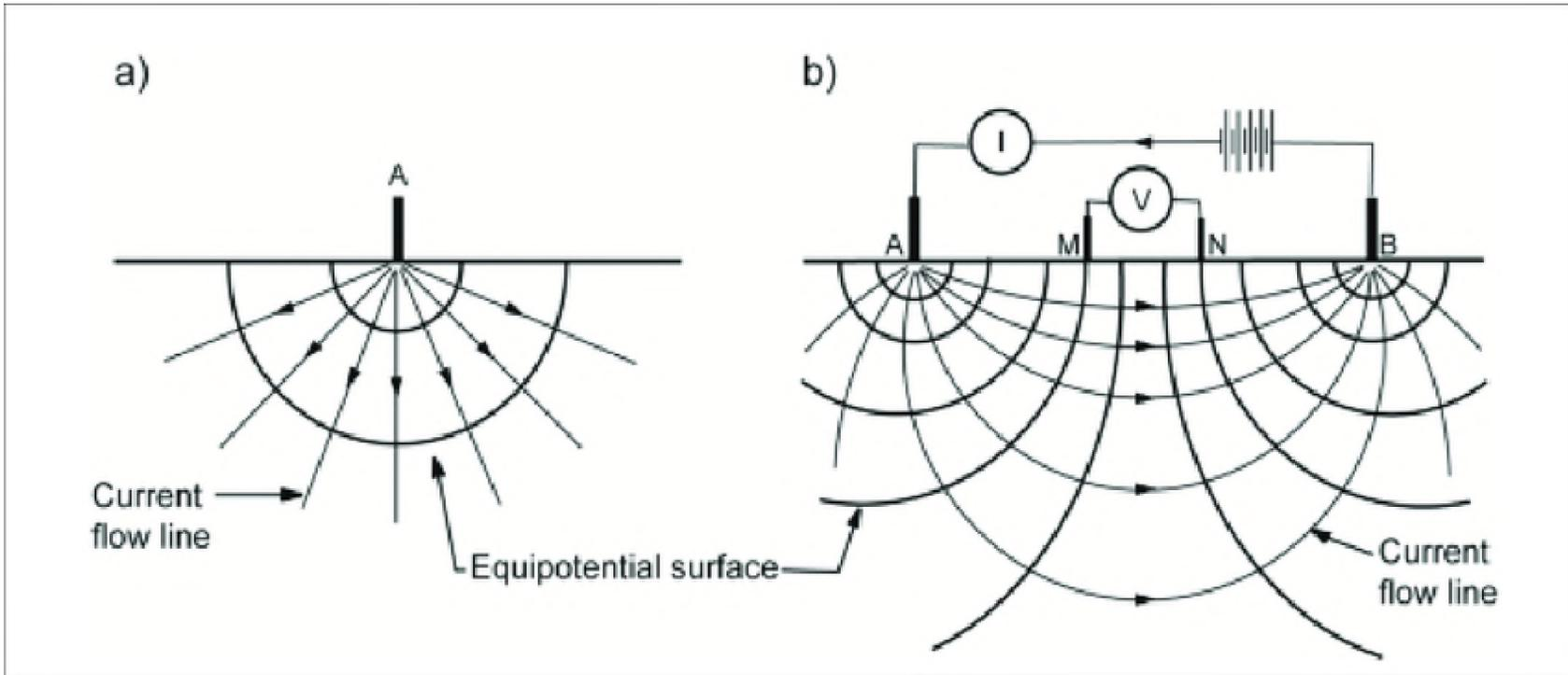
Figure 5.3. Current flow lines and equipotential surfaces. Figure (a) Current or source electrode and figure (b) a simple four electrode array with current source (A and B) and current sink (M and N). These figures illustrate current flow lines and equipotential surfaces with a general array in a homogeneous subsurface.
