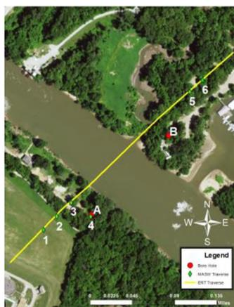
Figure 6.1. Aerial photo of the site with ERT survey traverse, MASW locations, and boreholes shown.
