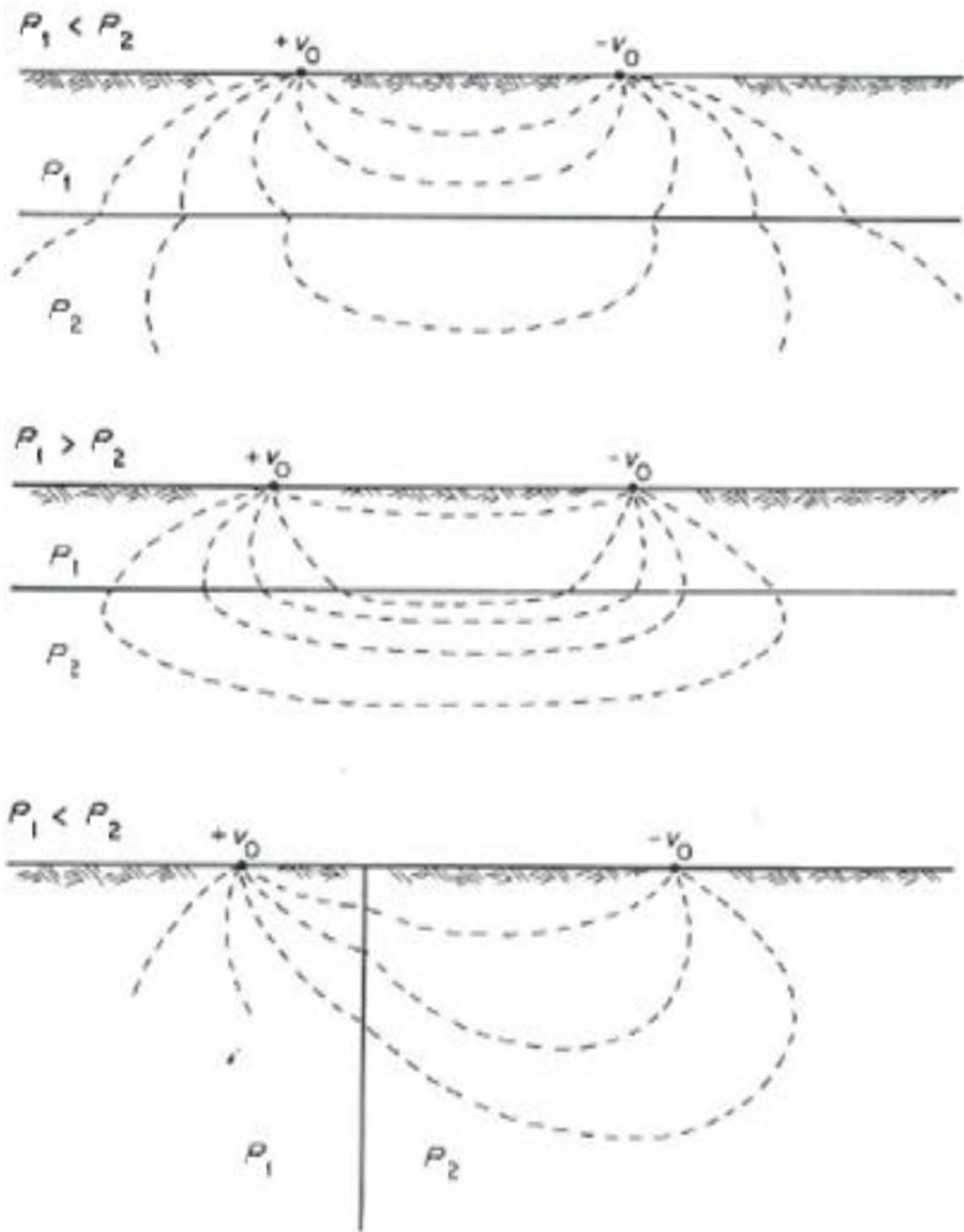
Figure 5.6. Illustrates current flow lines across interfaces with different resistivity ( $\rho_1, \rho_2$ ) (Robinson and Coruh, 1988).
