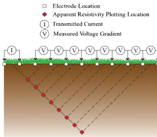
Figure 5.9. Illustration of 2-D Dipole-Dipole array pseudo-section plot.
