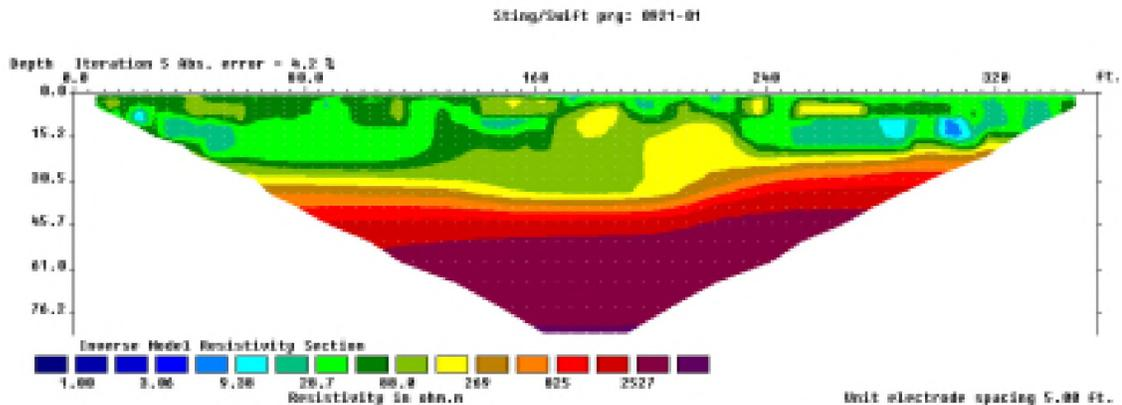
Figure 5.1. Example pseudo-section. Example of a typical 2-D pseudo-section of the area. Nwokebuihe, S. C. (2014).
