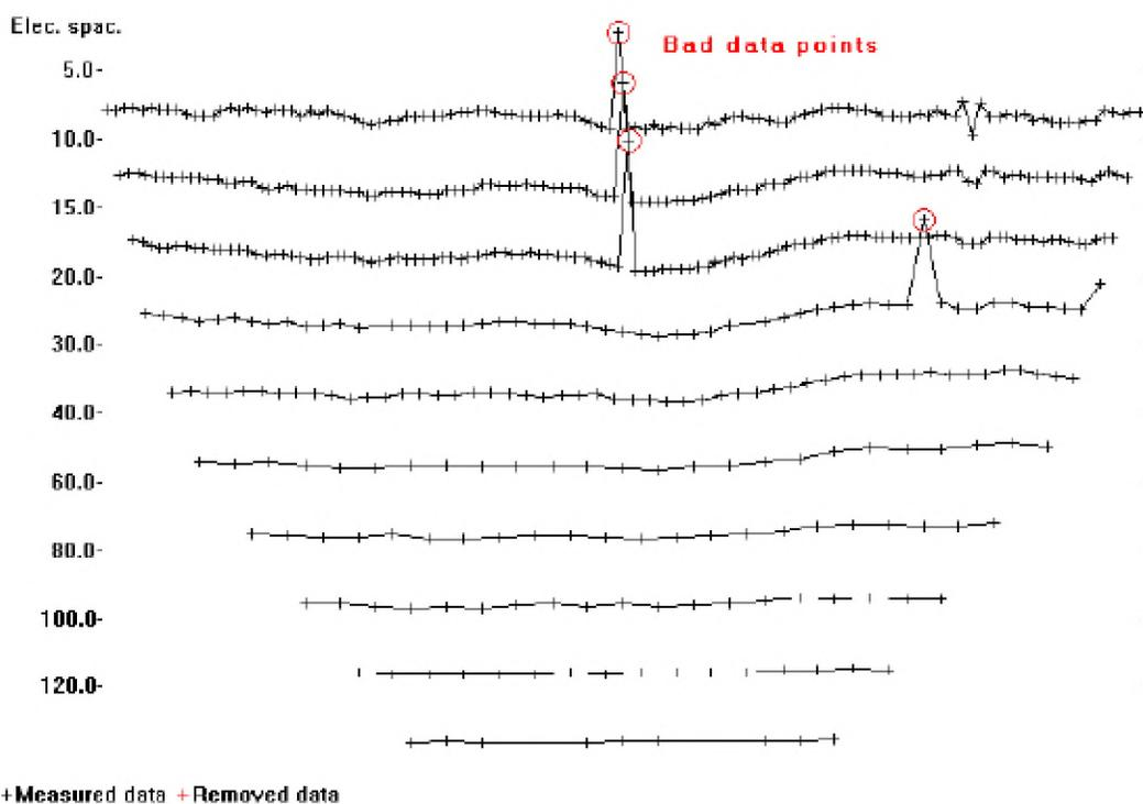
Figure 5.11. Apparent resistivity profile with bad data points (marked with red circles) which need to be removed before the inversion process (Loke, 1999).
