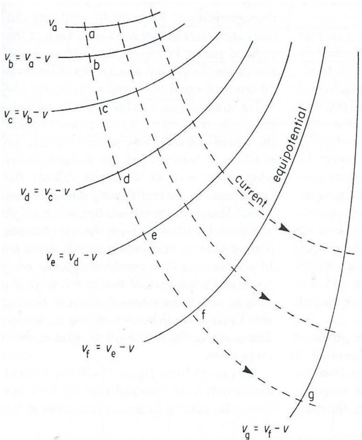
Figure 5.5. Illustration of the change of equal potentials along a current flow line from source/sink (Robinson and Coruh, 1988).
