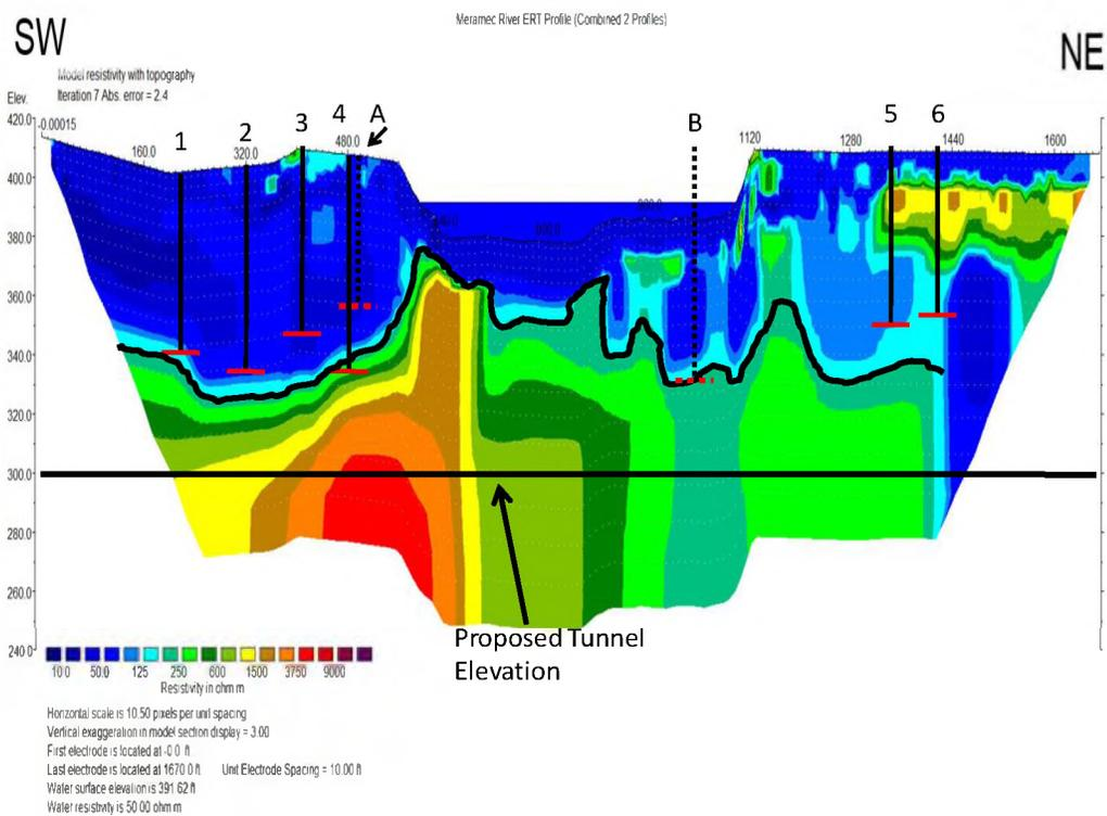
Figure 6.15. Interpreted ERT pseudo-section with interpreted MASW data and boreholes A and B.
