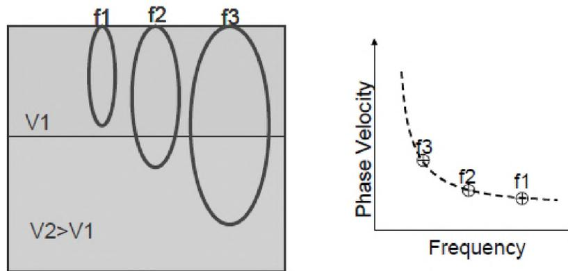
Figure 5.15. Illustration of dispersive components of different frequencies versus velocity (Billington et. al., 2007).
