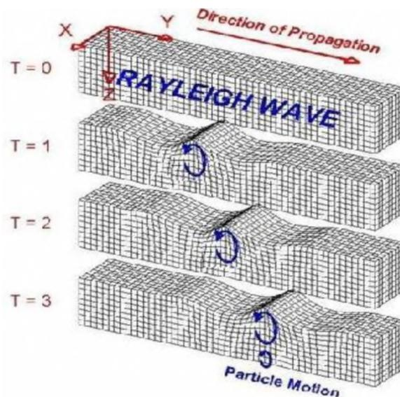
Figure 5.14. Illustrates the propagation of Rayleigh wave motion through the surface with respect to time. (Anderson, 2017).
