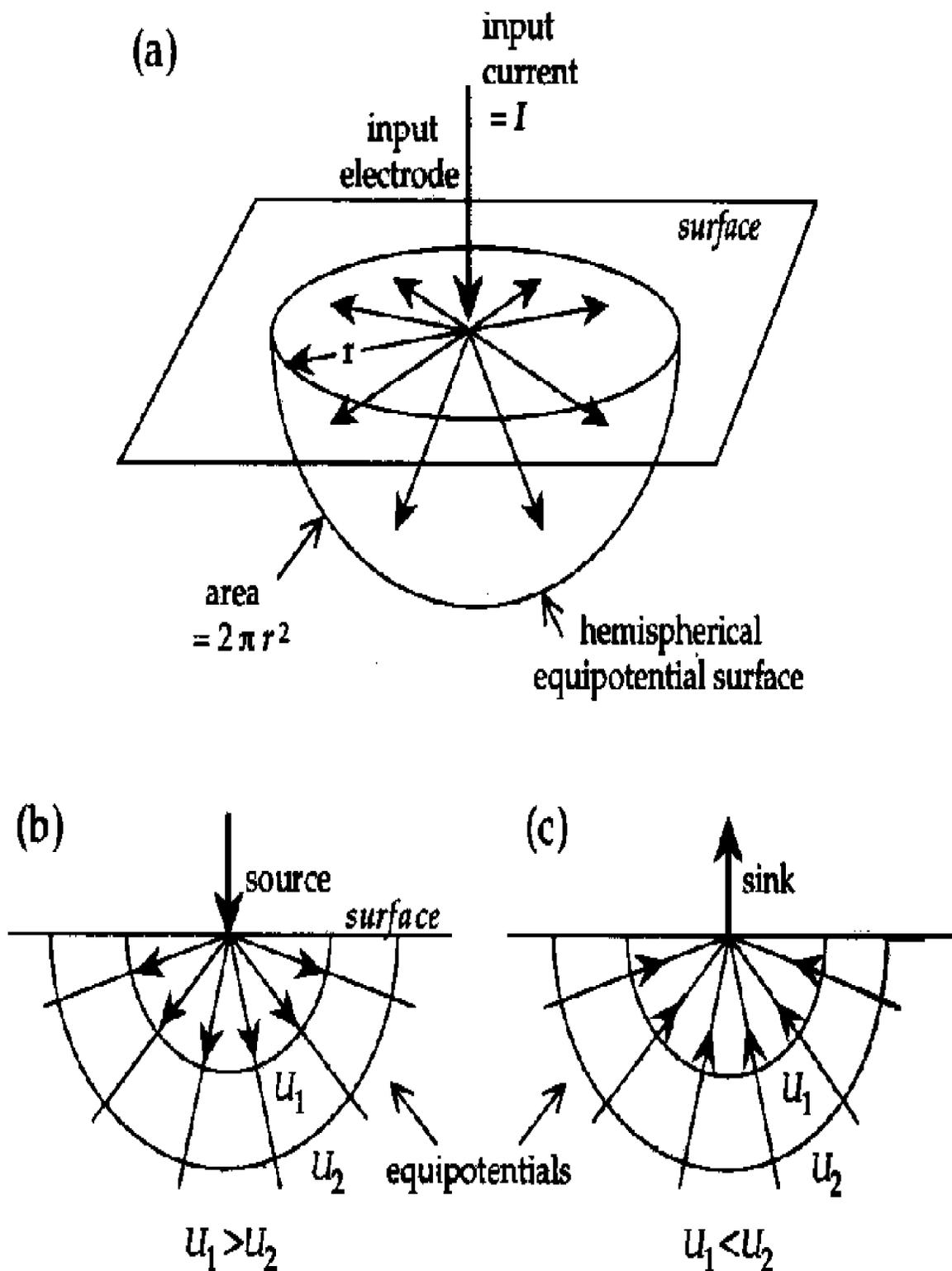
Figure 5.4. Illustration of uniform equipotential surface with current flow lines in all directions (a) and 2-D cross-sections of the hemispherical surfaces at the source (b) and sink (c) electrodes (Lowrie, 1997).
