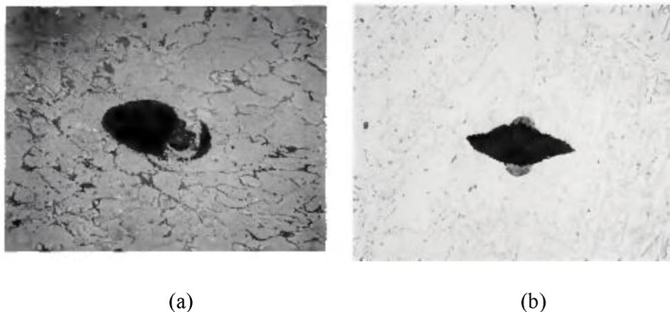
Figure 1.7. Inclusions leading to fracture. (a) An inclusion acting as a nucleation site for microvoid nucleation leading to ductile fracture (b) an inclusion acting as an initiator of a cleavage crack leading to brittle fracture <sup>[35]</sup>
