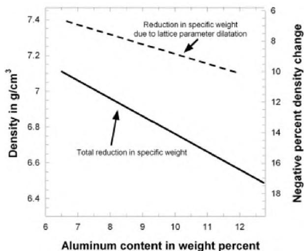
Figure 1.14. Increasing the aluminum from 6.5 to 12% in a Fe-30Mn-XAl-0.9C steel leads to a total reduction in density from 7.5 to 6.2 g/cm<sup>3</sup><sup>[13]</sup>
