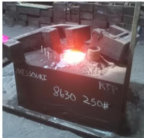
Figure 9. Image of the mold directly after pouring at the industrial partner foundry shows a full pouring basin and no spillage
