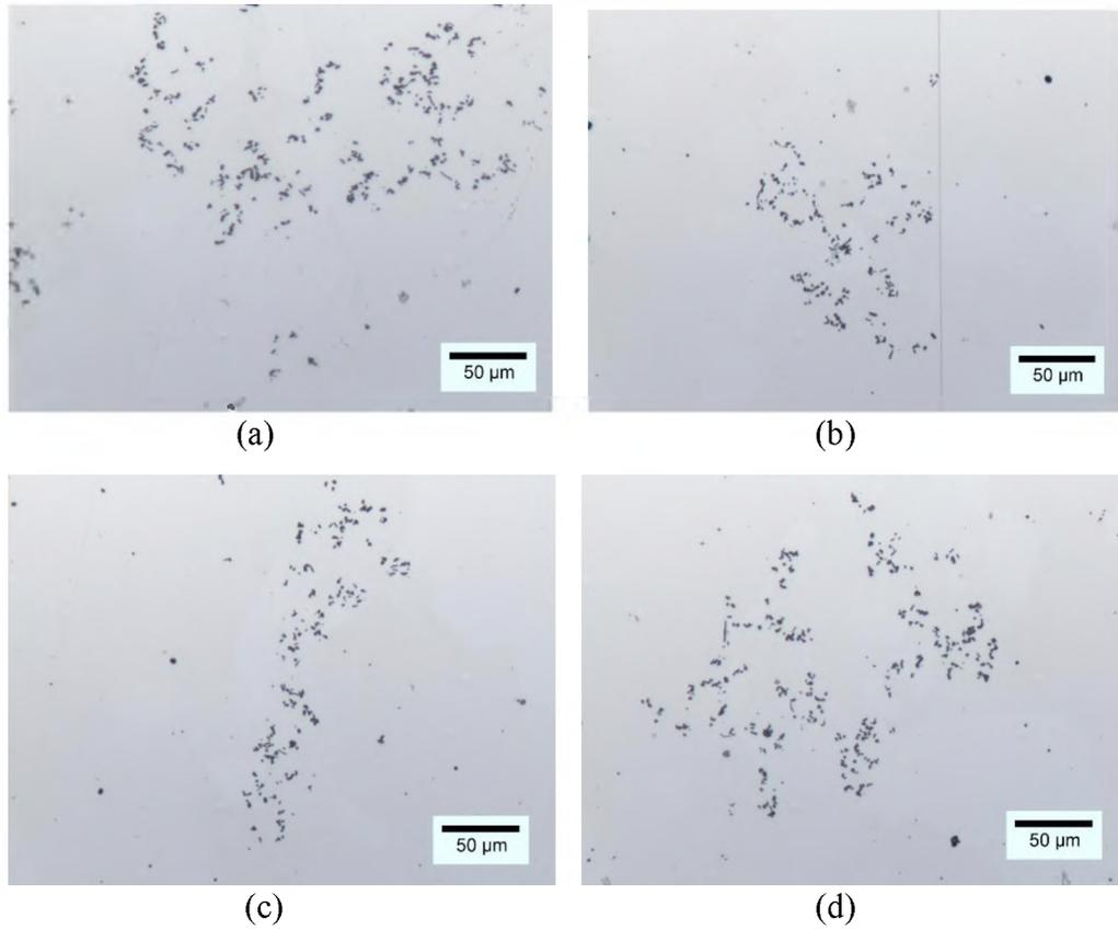
Figure 13. The optical micrographs taken from the different gating systems in mold 1 reveal the presence of inclusions present in clusters throughout the samples. (a) Naturally pressurized top riser (b) Naturally pressurized side riser (c) Non-pressurized system (d) Pressurized system
