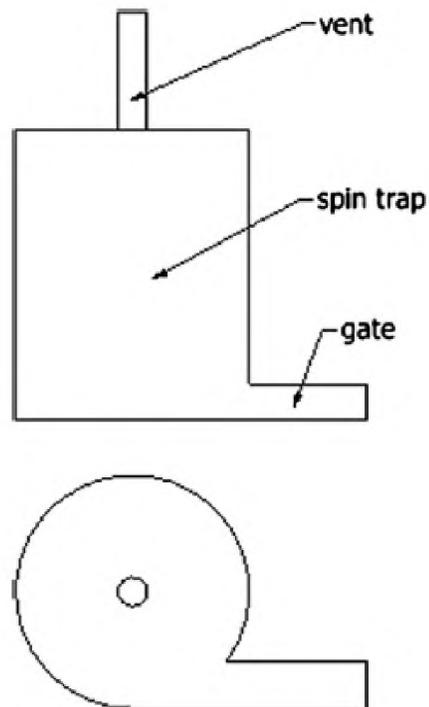
Figure 1.23. The vortex gate showing the presence of a gate and the velocity tracker which collects the incoming metal from the runner and traps all the slag and aids in velocity control <sup>(82,10)</sup>
