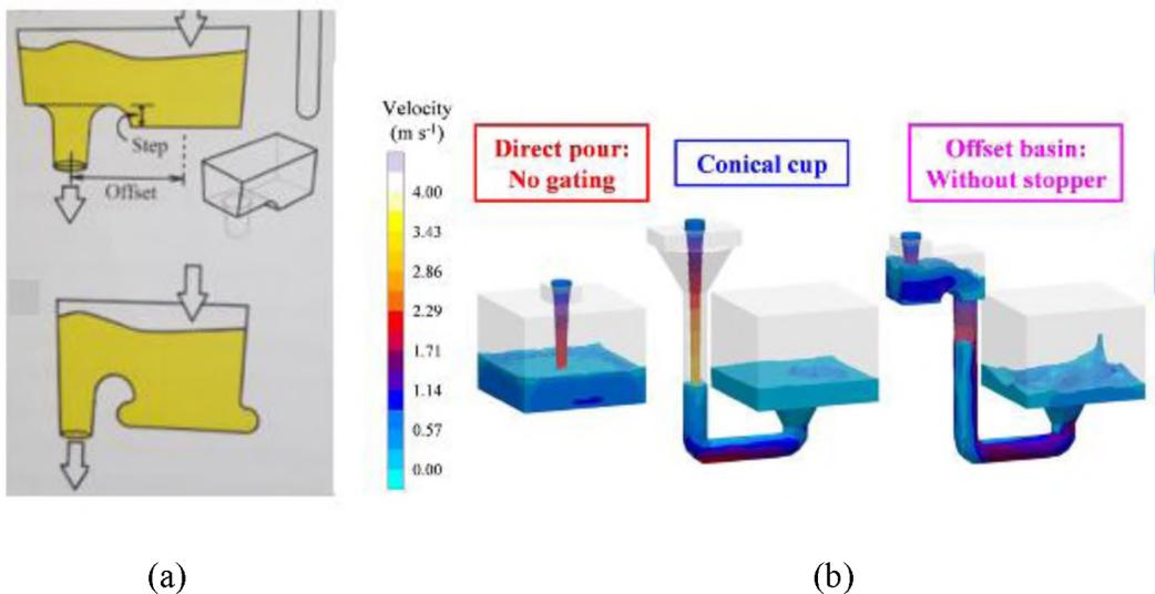
Figure 1.21. Use of offset basin and an undercut (a) An offset pouring basin helps to control the flow of the incoming liquid from the ladles and stabilizes it and an undercut that is provided to the basin to slow down the flow of metal and prevent it from splashing over the pouring basin (c) comparison of flow velocity between the three pouring systems<sup>[81]</sup>
