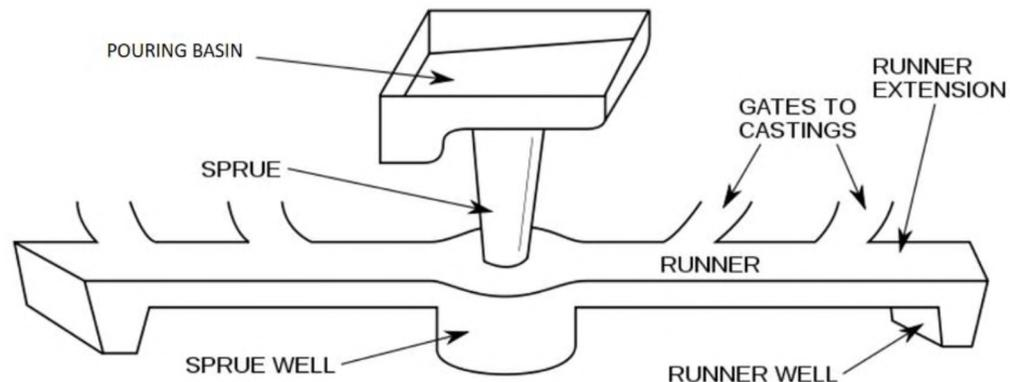
Figure 1. Horizontally parted gating systems that are typically used in the steel casting industry<sup>[9]</sup>
