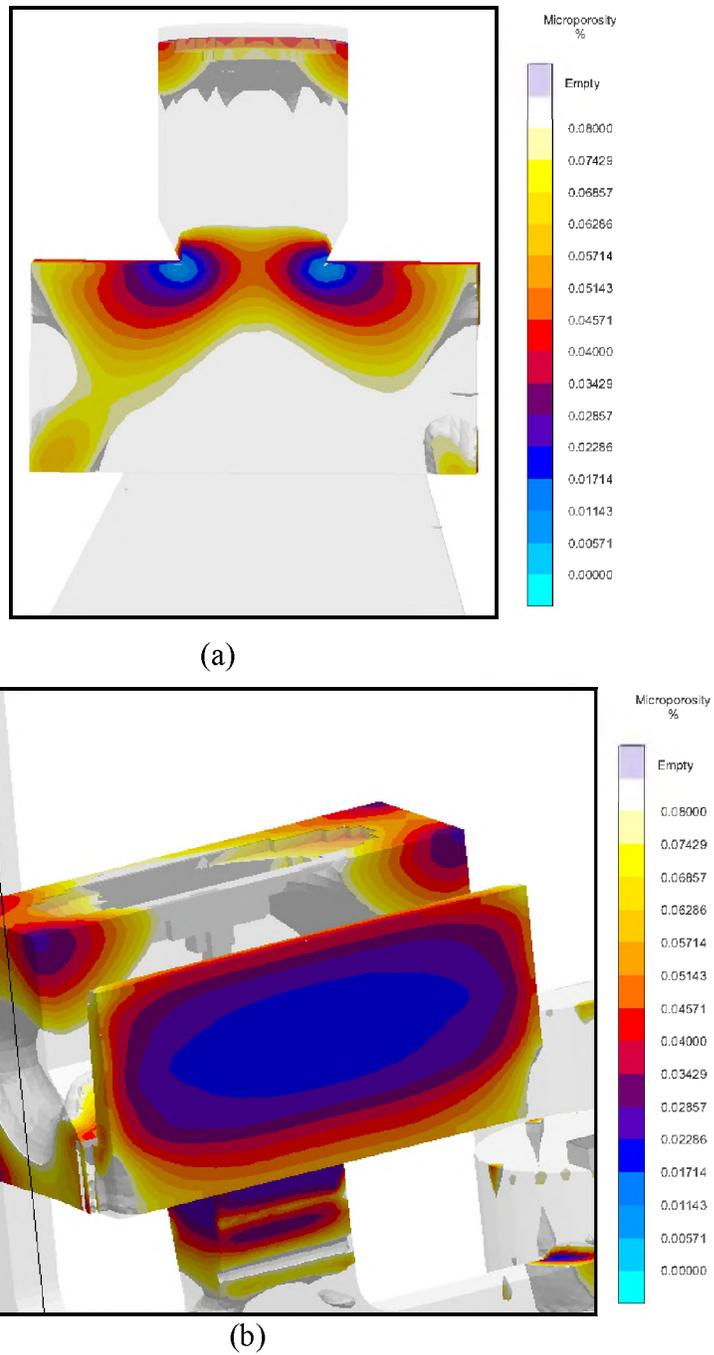
Figure 3. The castings were designed to ensure a microporosity less than 0.08%.
