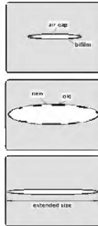
Figure 1.11. Hydrogen induced porosity formation. (a) The bifilm observed with an air gap in the matrix (b) the formation of an dense and an thin layer of bifilm that is formed because of pore expansion due to hydrogen diffusion or pressure change (c) The new enlarged area of the bifilm preventing its return to normal size<sup>[47]</sup>
