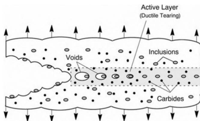
Figure 1.9. The nucleation of micro voids created by the presence of inclusions aiding in crack propagation and subsequent fracture<sup>[38]</sup>
