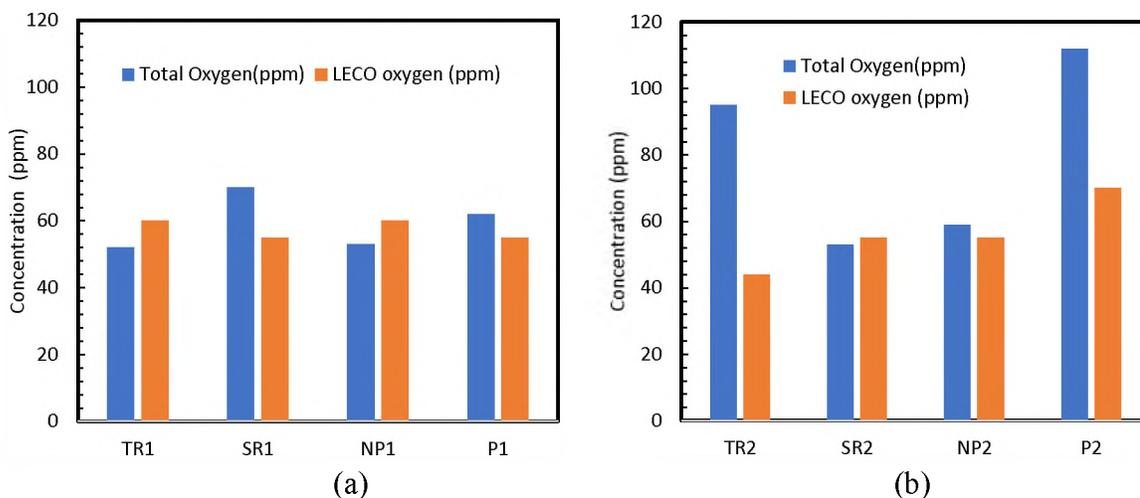
Figure 22. Calculated total oxygen contribution of inclusions from specimens obtained from the top section of the castings as compared to the measured oxygen from LECO analysis
