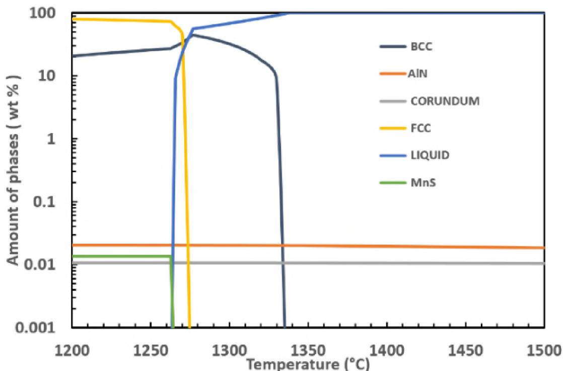
Figure 4. Thermodynamic modeling of the equilibrium solidification of a Fe-30Mn-9Al-1Si-0.9C-0.5Mo steel with 0.007% N, 0.005% O, and 0.005% S. AlN and Al<sub>2</sub>O<sub>3</sub> are stable in the liquid well above the liquidus. MnS forms after the liquidus during solidification
