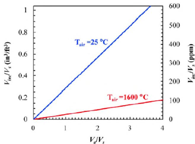
Figure 1.6. For a low carbon alloy steel, the variation in total inclusion volume ( $V_{inc}$ ) is shown as a function of relative entrained air volume ( $V_a$ ) at room temperature and when air is at  $1600\text{ °C}$  [34].  $V_s$  indicates the total steel volume in the mold
