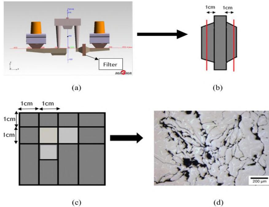
Figure 5. Experimental procedure for sectioning filter and obtaining specimens for AFA analysis. (a) The design showing the position of the filter (b) Representative image showing how the filter was sectioned (c) Representative image showing where the metallographic and inclusion analysis samples sectioned from each side of the filter. (d) Optical micrograph of one of the samples taken before the filter
