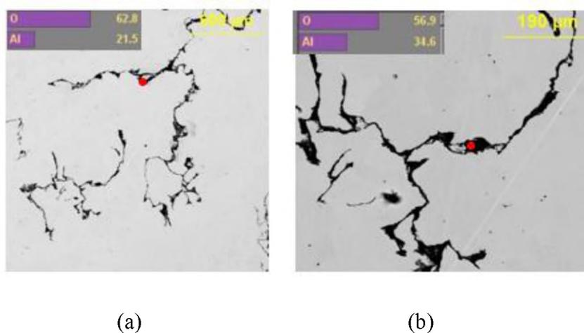
Figure 14. Backscattered electron images of the area sectioned underneath the fractured surface of a Charpy bar from the SR system shows alumina bifilms on the surface confirming that the bifilms were the main reason for failure
