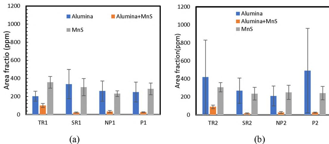
Figure 17. The overall average area fraction of alumina, Al<sub>2</sub>O<sub>3</sub>-MnS complex inclusions and the MnS inclusions for (a) mold 1 and (b) mold 2 respectively. The NP and SR system showed consistent values while the TR exhibited highest values for the complex and MnS inclusions respectively
