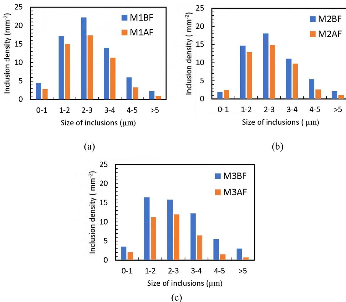
Figure 13. Inclusion density as a function of the size distribution the unfiltered and filtered samples in (a) mold 1 (b) mold 2 and (c) mold 3
