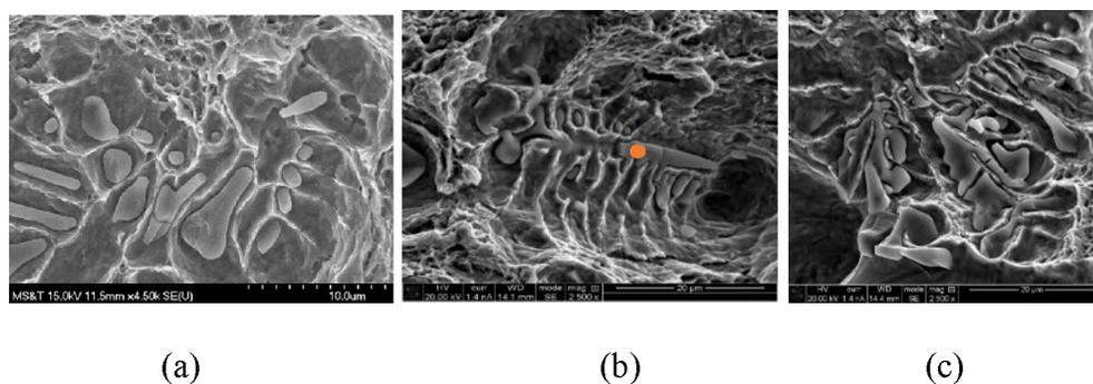
Figure 21. From the pressurized system of mold 1, fractography was performed on the bars which showed the presence of type II eutectic manganese sulfides formed in the chain or fan structure. (b) EDS analysis showed the MnS inclusions were composed of roughly 45%Mn and 27% sulfur by weight
