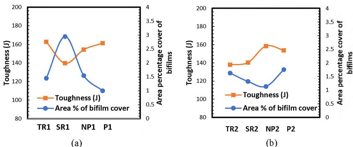
Figure 12. The comparison between the 8-notch toughness obtained from layer 1 and layer 2 of every gating system and the area % of bifilm cover from the top section of the casting for (a) mold 1 and (b) mold 2
