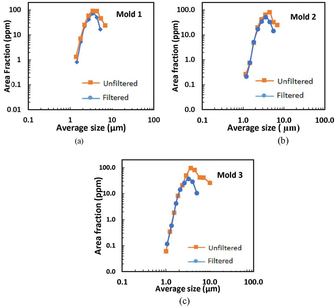
Figure 14. Size distribution of aluminum nitride inclusions as a function of area fraction for filtered and unfiltered samples in (a) mold 1 (b) mold 2 and (c) mold 3
