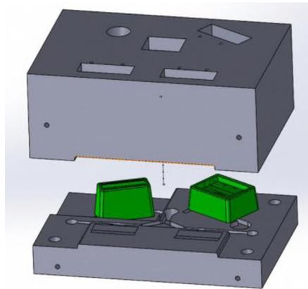
Figure 8. CAD drawing of the mold assembly shows the cope box containing the risers and the casting cavities while the drag box contains the runners and the gates
