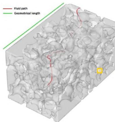
Figure 1.19. The comparison between the streamlined flow of a fluid (green line) and the flow path of the fluid inside a porous media (red line) <sup>(76)</sup>
