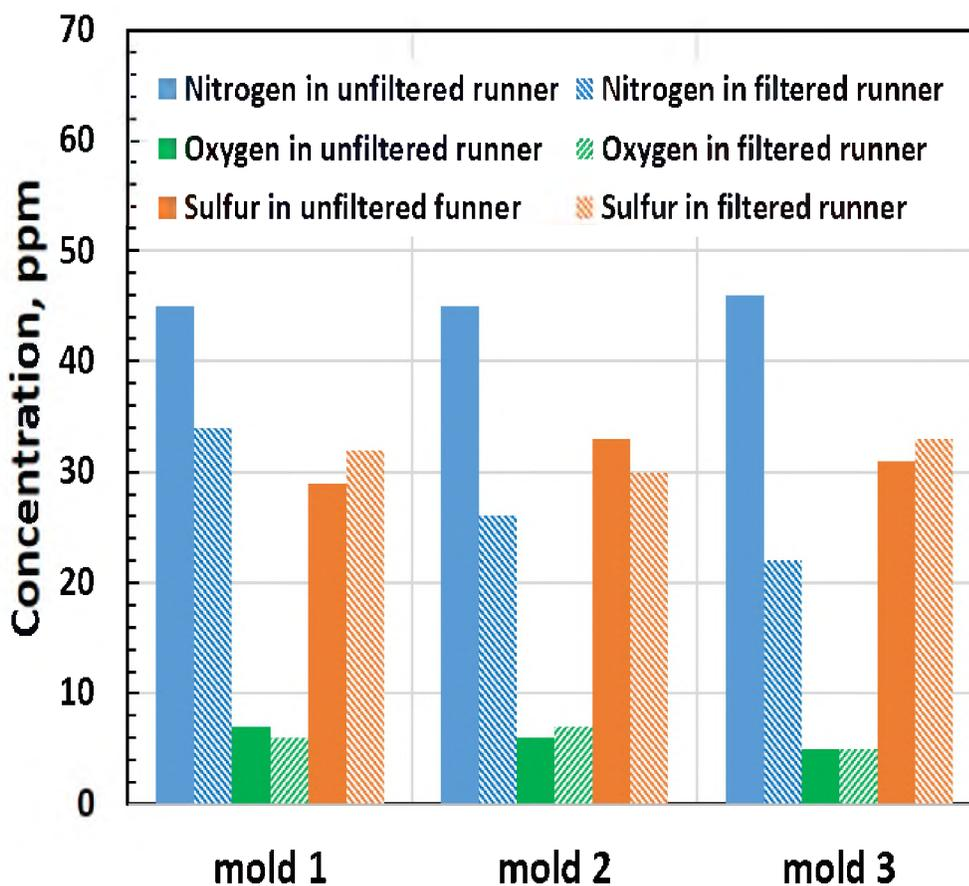
Figure 15. LECO analysis of N, O, and S concentration content from samples taken from the unfiltered runners and in the runners after filters as a function of mold pouring order
