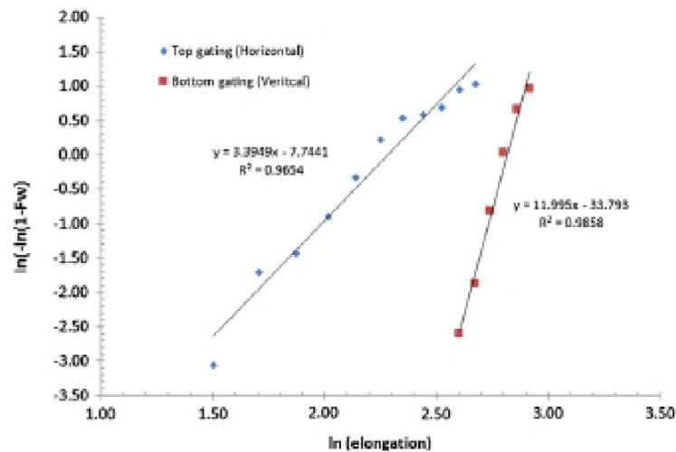
Figure 1.13. The Weibull modulus for the top gated system is 3.4 while for the bottom gated system it was observed to be 12. The difference in elongation, was attributed to the random distribution of bifilms in the top gated system [7]
