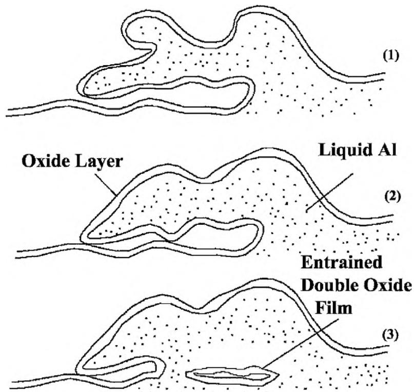
Figure 1.10. The formation of a bifilm defect generally takes place due to turbulent flow of metal. In the image (1) the turbulence in aluminum is observed while the image (2) shows the formation of bifilm with two unbonded internal side wetted by all direction in the outer direction <sup>[43]</sup>
