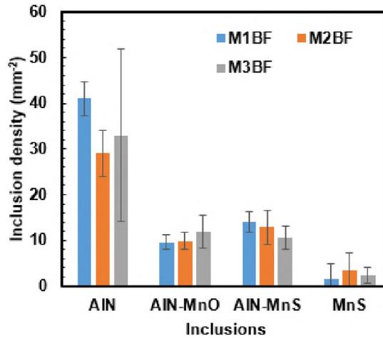
Figure 10. Inclusion density of inclusions by type, taken from the three molds before the filter, indicating a high density of AlN inclusions
