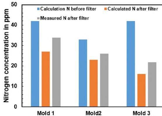
Figure 16. Calculated total nitrogen contribution of inclusions from specimens sectioned before and after the filter as compared to the measured total nitrogen after filtration
