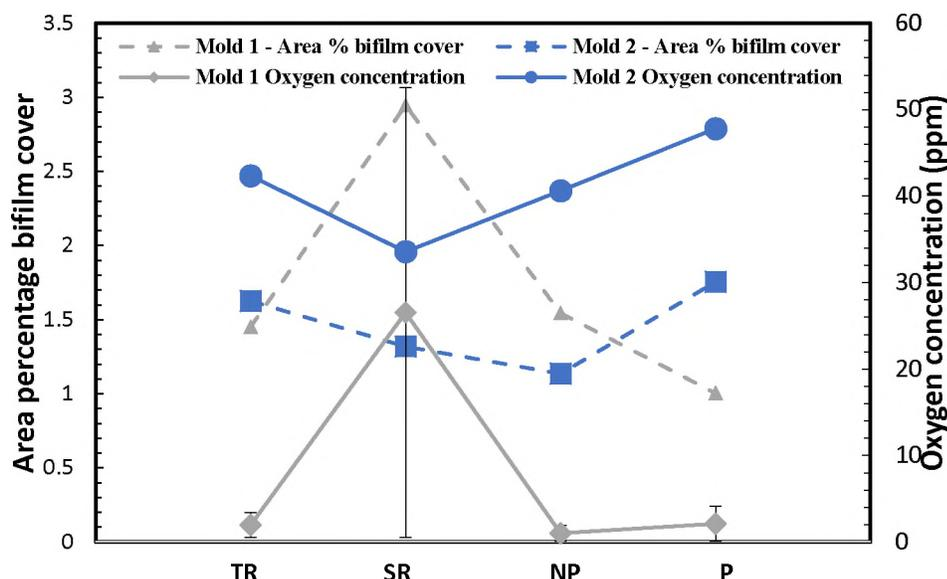
Figure 11. A comparison shown between the total oxygen concentration (ppm) and area % of bifilm cover in the castings obtained from different gating systems for mold 1 and mold 2. The amount of total oxygen was found to correlate to the total amount of bifilm coverage
