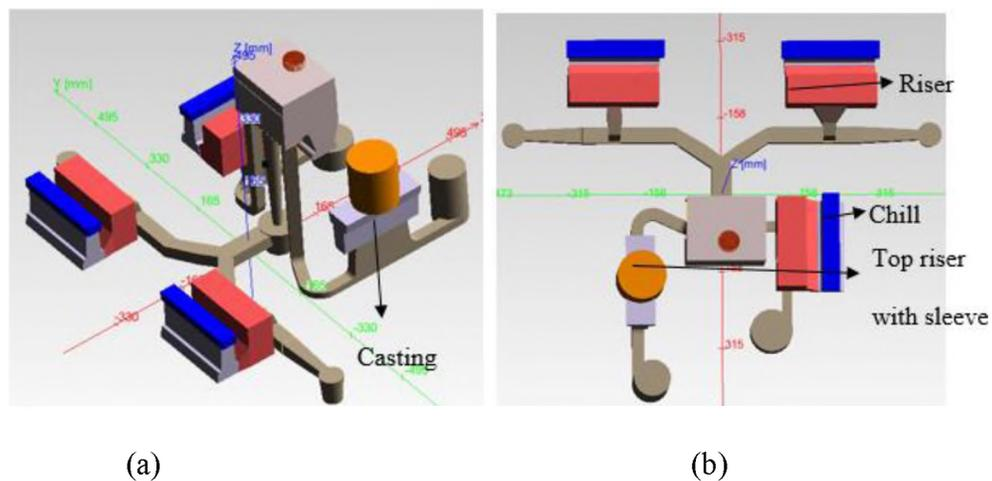
Figure 2. The complete design of the four gating systems in (a) isometric view (b) top view
