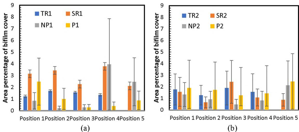
Figure 7. The percentage area of bifilm cover obtained as a function of position in the casting as referenced in Figure 4 for (a) mold 1 and (b) mold 2
