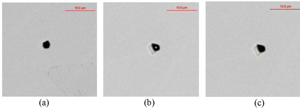
Figure 9. SEM images of different inclusions found in the steel (a) An image of an aluminum nitride inclusion (b and c) A complex AlN-MnS inclusion with the AlN at its core and (c) a MnS inclusion around the AlN
