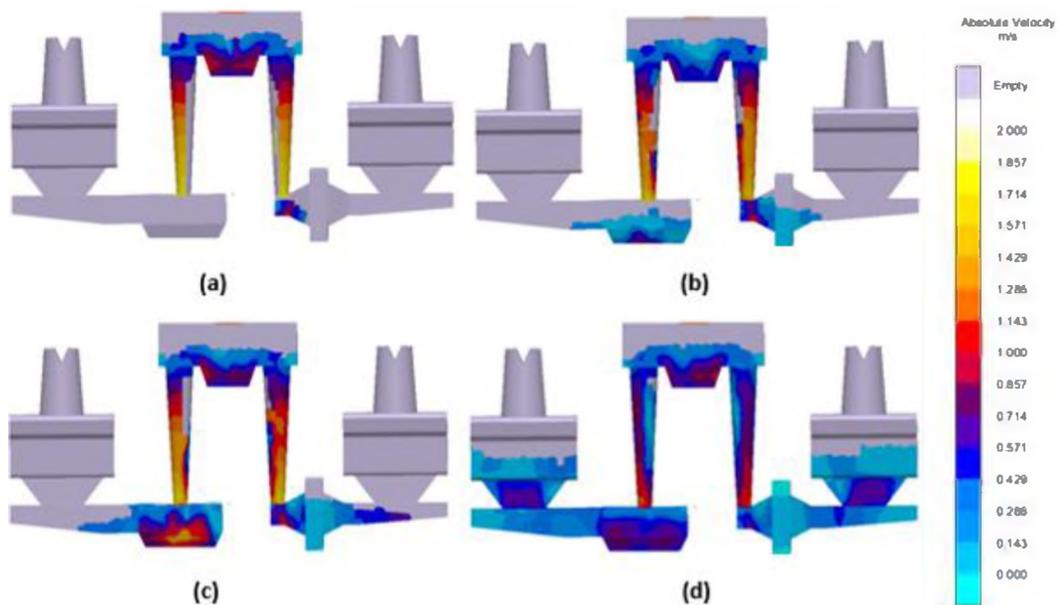
Figure 2. The velocity profile during filling at (a) 10% (b) 20% (c) 30% and 50% filled
