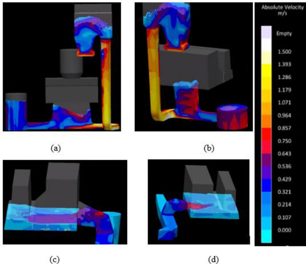
Figure 6. The velocity profile of filling when the molten metal enters the casting in (a) the naturally pressurized top riser system (b) the naturally pressurized side riser system (c) the pressurized system and (d) the non-pressurized system. In (c and d), gate velocity was slightly higher in the traditional pressurized and non-pressurized systems and increased from less than 0.5 m/s to 0.8m/s
