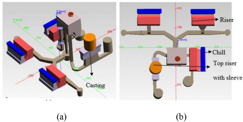
Figure 1. The complete design of the four gating systems in (a) isometric view (b) top view
