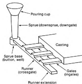
Figure 1.20. Elements of a gating system showing the pouring cup, sprue, sprue base, runner, runner extension, and multiple gates leading into the casting <sup>(78)</sup>
