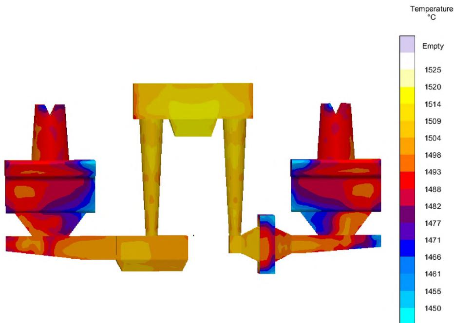
Figure 3. The temperature profile directly after filling shows that all temperatures are above the calculated liquidus temperature of 1338°C at all points in the design
