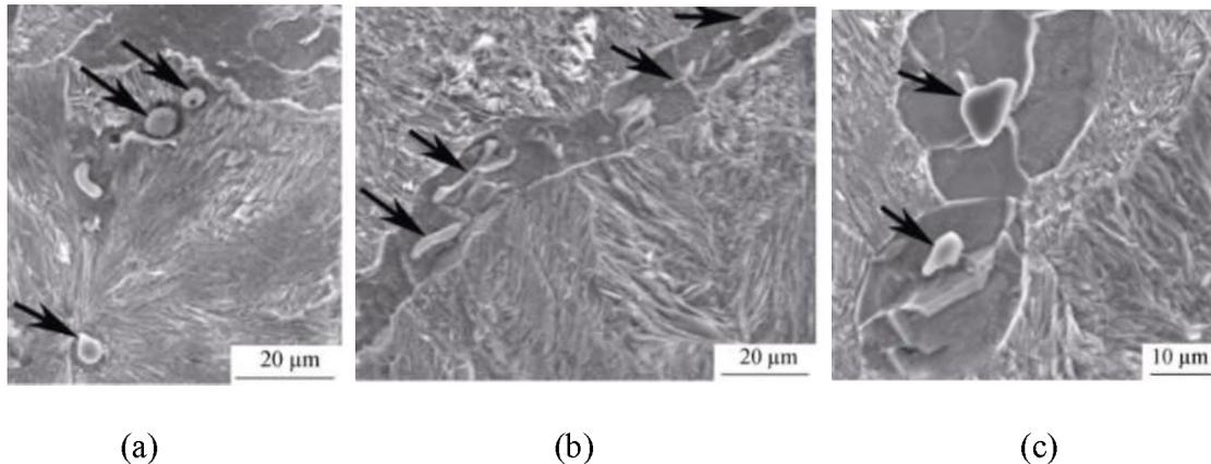
Figure 1.4. The manganese sulfides appear in various morphologies as shown in (a) globular type I sulfide (b) eutectic type II sulfide (c) type III angular faceted sulfide<sup>[20]</sup>
