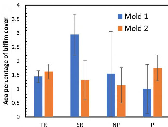
Figure 8. The percentage area of bifilm cover obtained as an average of all the samples obtained from the different positions of top layer of the castings as referenced in Figure 4 of various gating systems for mold 1 and mold 2
