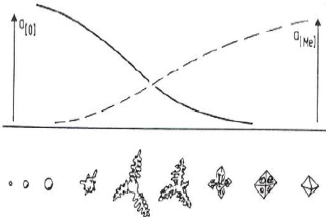
Figure 1.3. The growth of the different morphologies of oxide inclusions shown as a function of the deoxidizer activity (dashed line) and O activity (solid line) <sup>[19]</sup>
