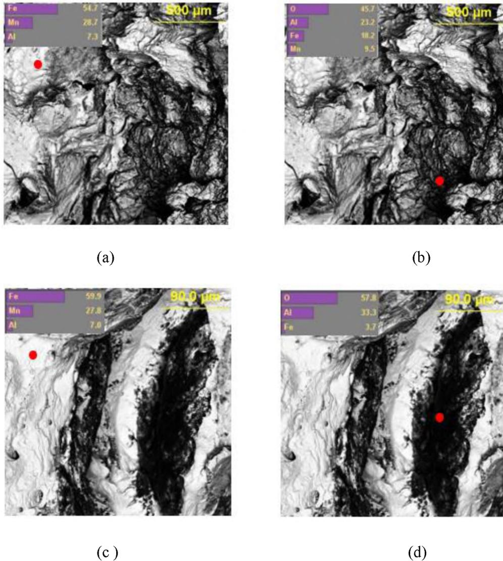
Figure 10. Backscattered electron images of fractured Charpy bars obtained from the SR system of mold 2 showing a dense layer of bifilms rich in aluminum oxide. The red dots indicate the location for chemistry analysis presented in the inset images. (a and c) The matrix chemistry was similar to the nominal steel composition. (b and d) The composition of the bifilms was determined to be mainly alumina
