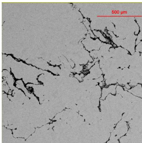
Figure 8. The backscattered electron image of a network of bifilms present in the sectioned sample taken before the filter from mold 1. It shows areas of bifilms that were determined to be mainly aluminum oxide
