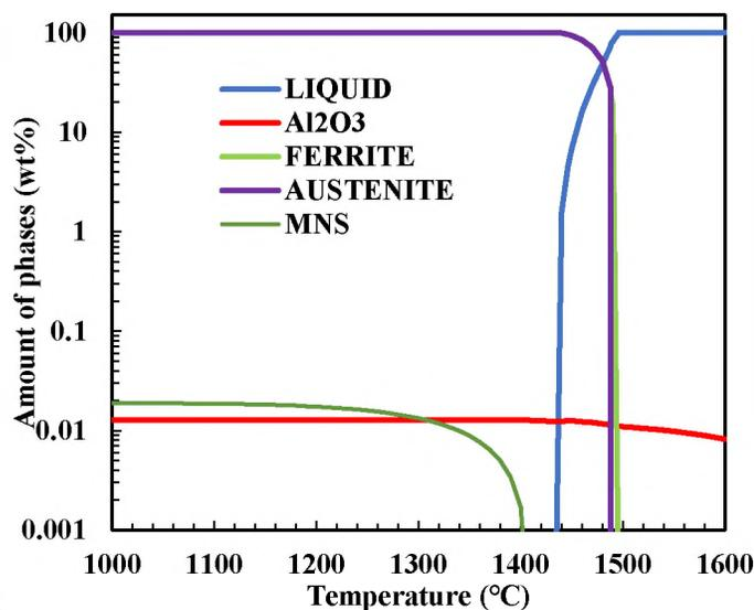
Figure 23. Thermodynamic modeling of the equilibrium solidification of 8630 steel with 0.0075% N, 0.006% O, and 0.007% S. Al<sub>2</sub>O<sub>3</sub> is stable in the liquid well above the liquidus. MnS forms after the liquidus during solidification
