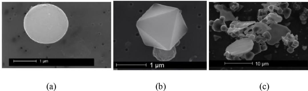
Figure 1.2. Morphologies of alumina inclusions. (a) The alumina inclusions are formed in various morphologies like (a) spherical (b) faceted and (c) clusters. The faceted inclusions are products of slow growth rates while clusters are formed because of high convective currents in the melt <sup>[18]</sup>
