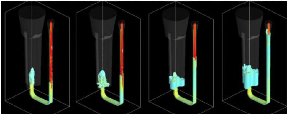
Figure 1.22. The transition of a sprue from a circular opening to a slim rectangular cross section ensures smooth filling and flow velocity. (red = high velocity) (blue = low velocity)<sup>[82]</sup>
