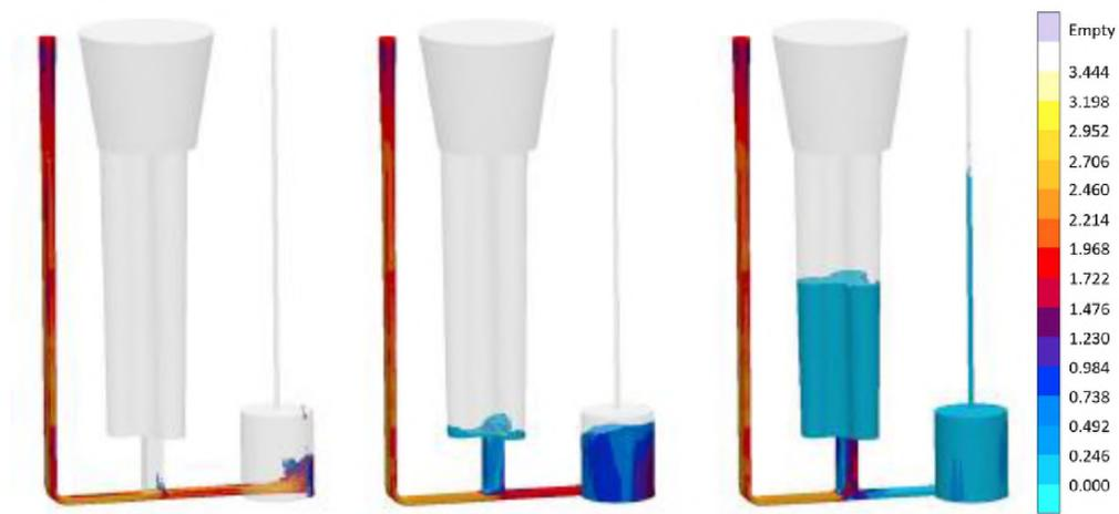
Figure 1.24. A gating system with a terminal trap. The terminal trap apart from controlling the incoming velocity, also collects the slag, dross and the inclusions carried by the incoming metal. This ensures the casting filled with new metal and a stable velocity as shown where the scale is absolute velocity in m/s [82]
