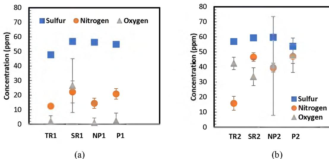
Figure 5. Measured concentrations of oxygen, sulfur, and nitrogen (in ppm) for samples taken from the castings of different gating systems for (a) mold 1 and (b) mold 2
