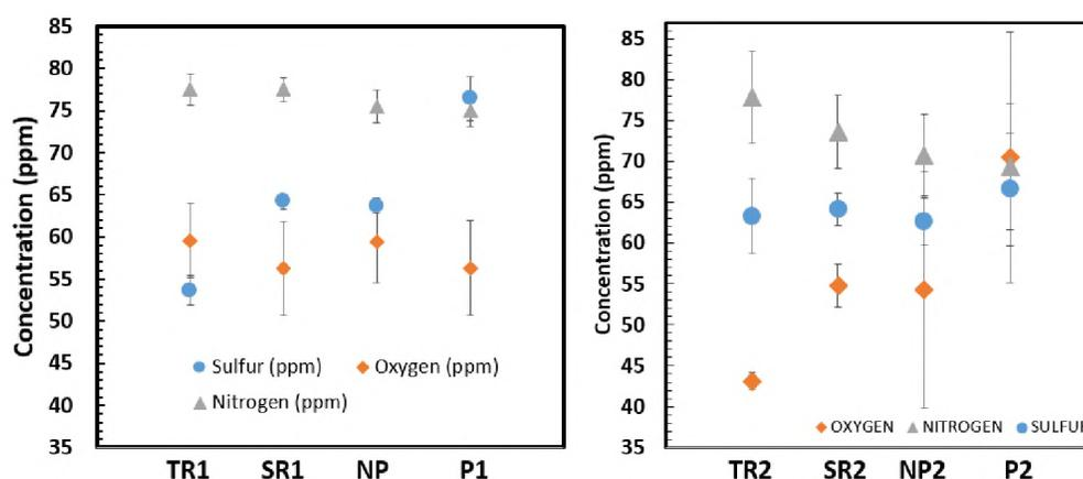
Figure 12. Total oxygen, sulfur, and nitrogen (in ppm) for samples taken from the castings of different gating systems. (a) The naturally pressurized top riser (TR) and side riser (SR) systems and traditional nonpressurized (NP) and pressurized (P) gating systems for (a) mold 1 and (b) mold 2
