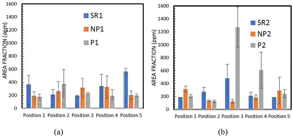
Figure 15. The area fraction of alumina inclusions with respect to the different positions from the top sections of castings from (a) mold 1 and (b) mold 2. The gating systems in mold 1 had an area fraction between 180-500 ppm. The pressurized system of mold two had high inclusion density compared to the rest of the systems
