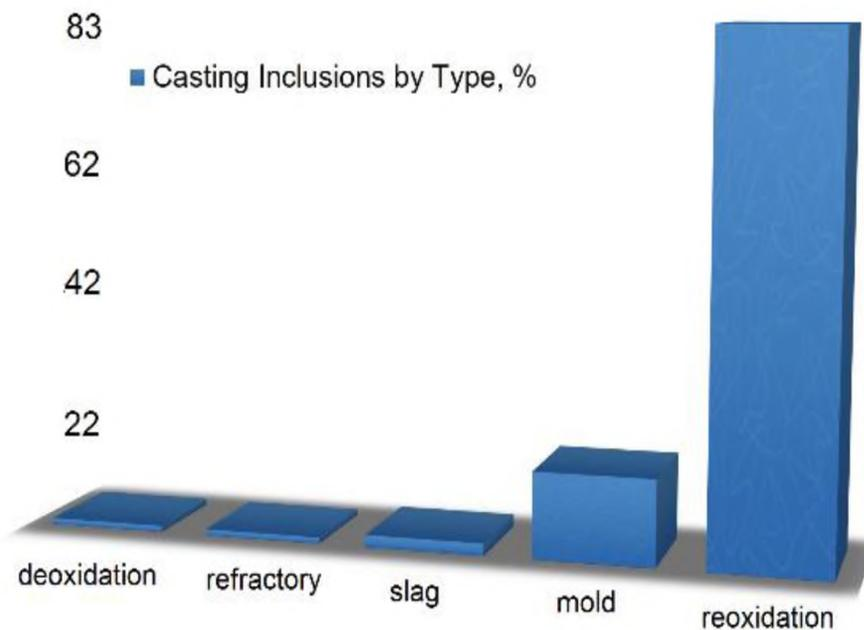
Figure 1.5. The work by Griffin and Bates showed that 83 % of all inclusions in low alloy steel castings are caused as the result of reoxidation <sup>[5]</sup>
