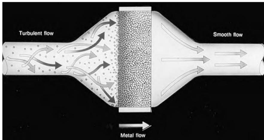
Figure 1.18. A filter enables in trapping particles from the incoming metal and helps to reduce turbulence when the metal passes to the other side of the filter <sup>[74]</sup>
