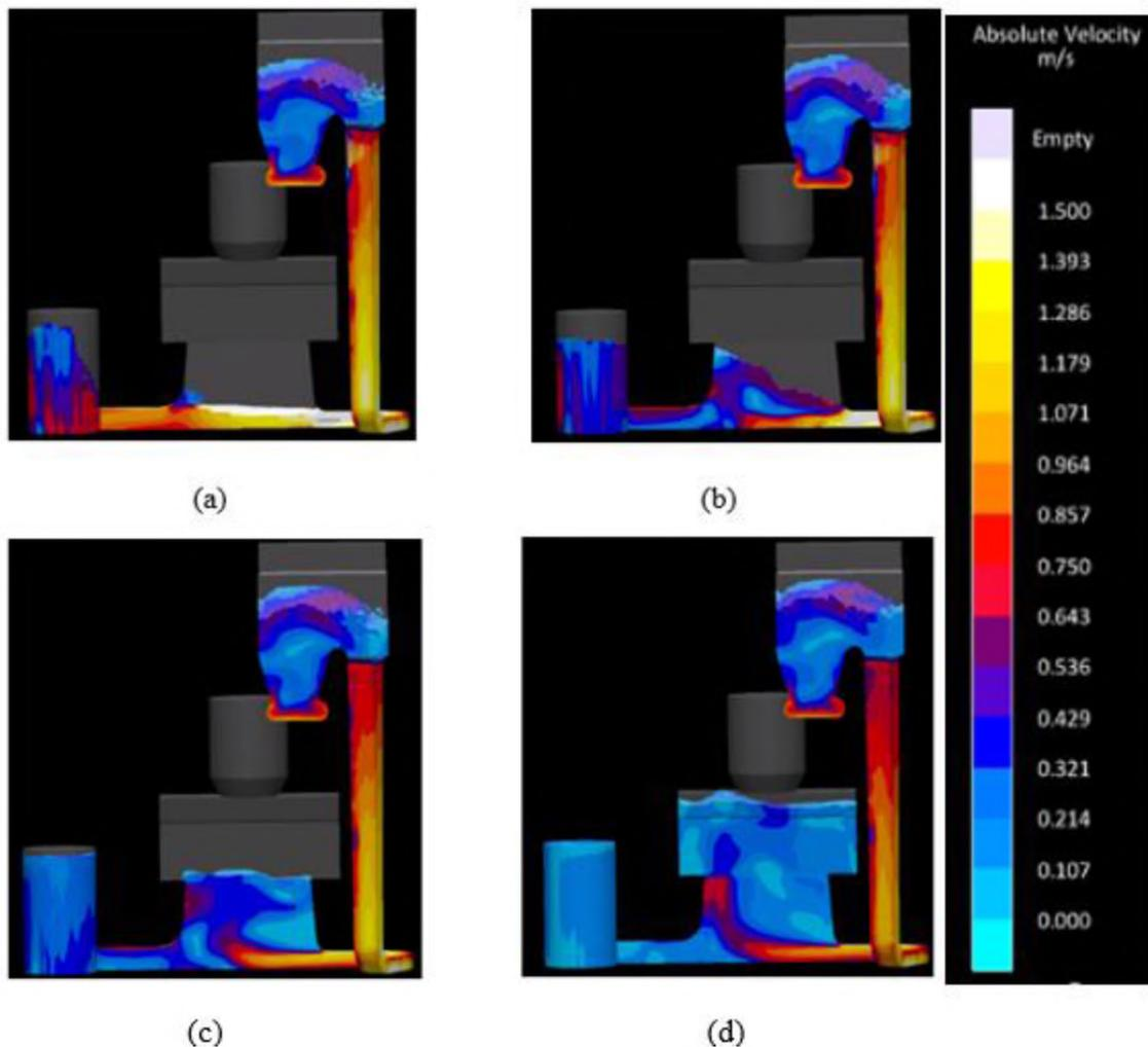
Figure 5. The velocity profile during filling for the top riser naturally pressurized gating system at (a) 30% (b) 35% (c) 50% and (d) 75% of complete filling of the mold observed between a scale of 0-1.5m/s. Molten metal is shown to enter the casting at less than 0.5 m/s and with a flat and quiescent filling profile
