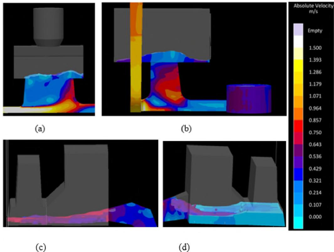
Figure 3. The velocity for filling when the metal enters the casting at various filling times in the (a) naturally pressurized top riser system (b) naturally pressurized side riser system (c) pressurized system (d) the non-pressurized system. All the castings were designed to have ingate velocities less than 0.8m/s
