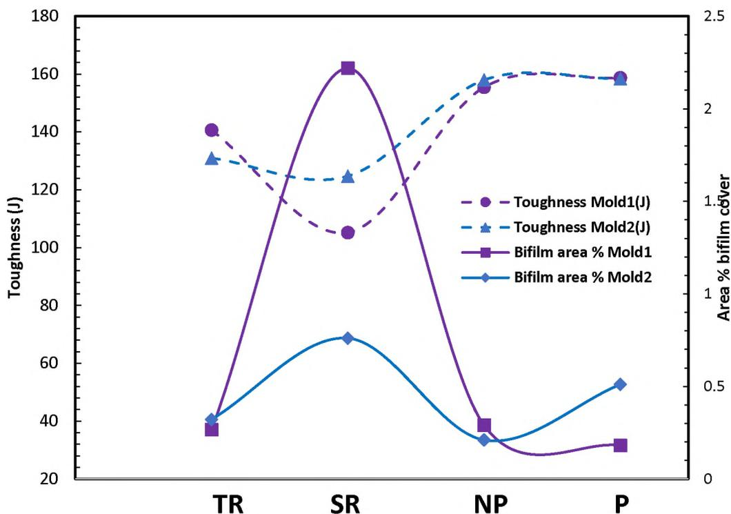
Figure 13. A comparison between the breaking energy and the area cover of bifilms obtained from right underneath the Charpy bar. It can be observed that the bifilms were the reason for failure and had a direct impact on the toughness of the steel
