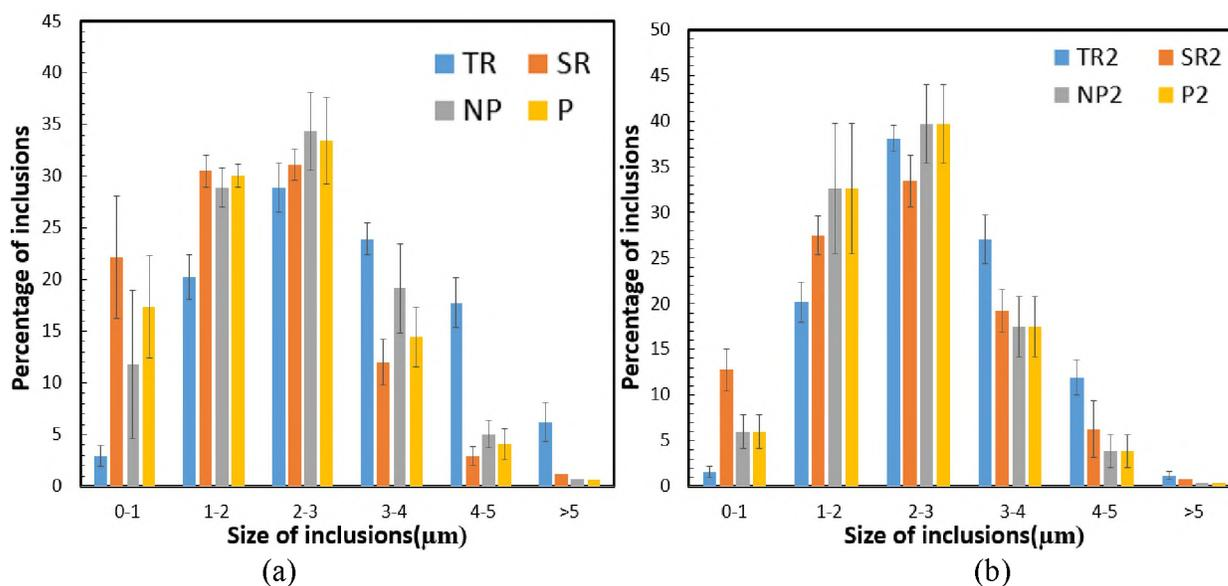
Figure 18. Comparison of size distribution of alumina and the complex inclusions for all the four systems in (a) mold 1 and (b) mold 2. It is seen that 60-70% of all inclusions are <3 μm. Mold 2 has higher size of inclusions than mold 1 which is attributed to inclusion floatation in teapot ladle
