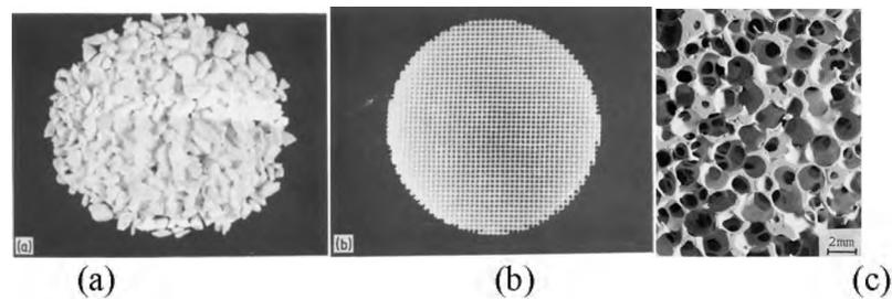
Figure 1.16. Photographs showing (a) tabular filters (b) monolithic filters<sup>(9)</sup> (c) ceramic foam filters<sup>[72]</sup>
