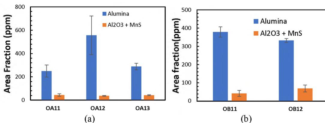
Figure 19. Inclusion analysis in overflows. (a) The area fraction of alumina and the complex inclusions plotted for the different sections of the overflow for the TR system (b) positions in the SR systems
