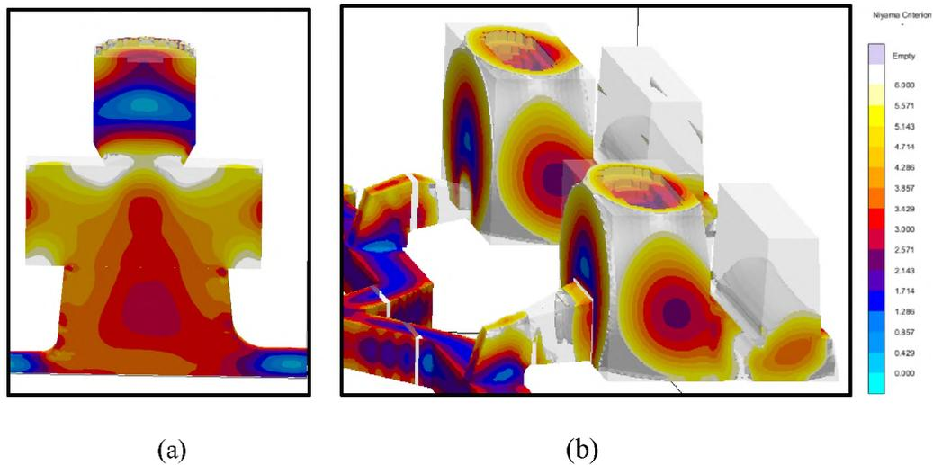
Figure 2. The castings were designed to have a Niyama number of greater than  $6(C-s)^{1/2}/\text{mm}$  for obtaining quality castings with low levels of microporosity. (a) The casting from top riser naturally pressurized system (b) Castings from the pressurized and non-pressurized systems
