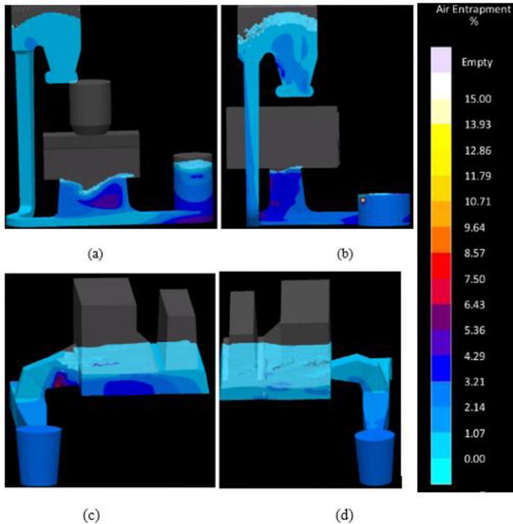
Figure 7. The air entrapment for filling when the metal enters the casting in (a) TR system (b) SR system (c) NP system (d) P system taken between a scale of 0-15%. All the castings were designed to have air entrapment lower than 15%
