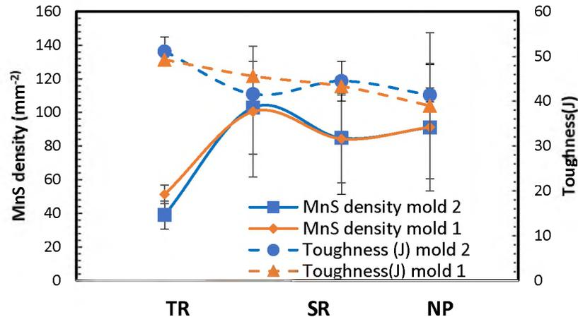
Figure 25. Notch toughness plotted along with the density of manganese sulfide inclusions for (a) mold 1 and (b) mold 2. It was observed that the toughness and the inclusion density display an inverse trend for both the molds
