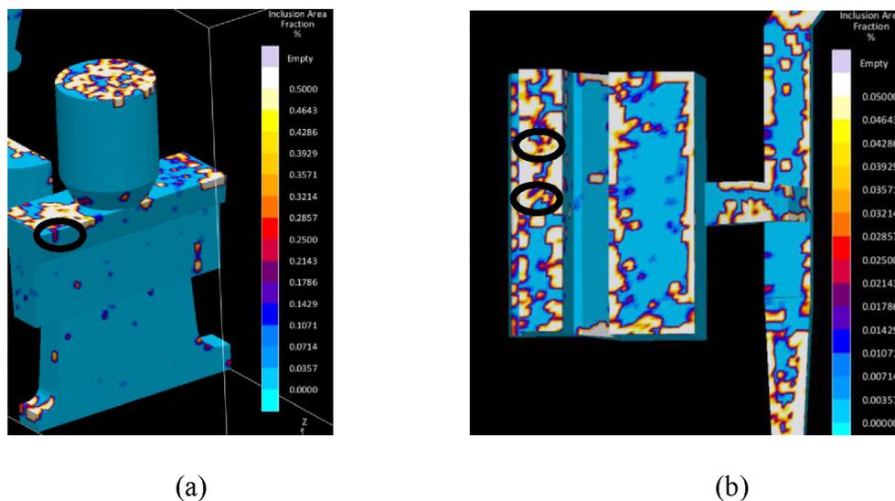
Figure 24. Magmasoft inclusion tracer analysis showing the position of reoxidation inclusions after filling. (a) The accumulation of alumina inclusions observed in the TR system where sample 3 was obtained for analysis (b) The alumina inclusion accumulation in pressurized system where samples 3 and 4 were obtained for analysis indicated using black circles on the castings
