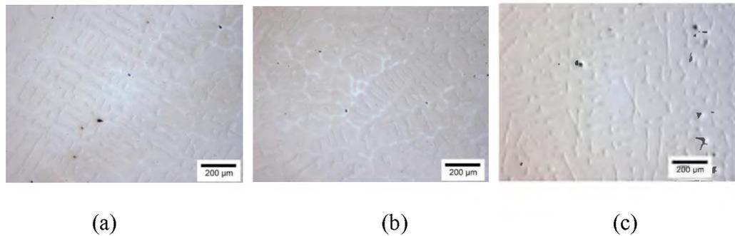
Figure 7. Optical micrographs of samples taken after the filter in (a) mold 1 (b) mold 2 (c) mold 3 show that bifilms have been effectively removed by filtration
