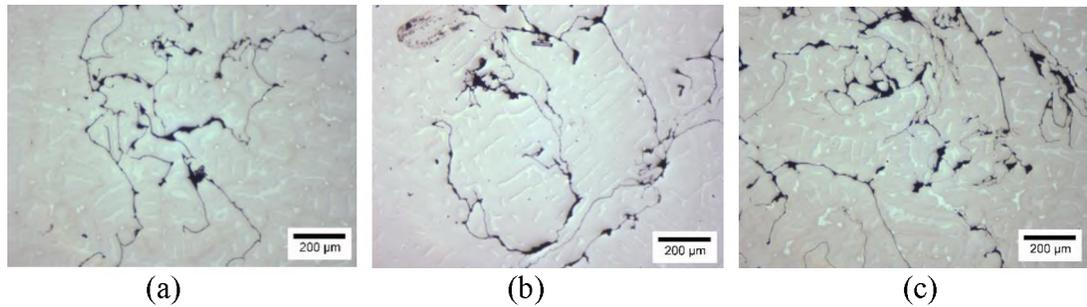
Figure 6. Optical micrographs of sections taken before the filter show a matrix of mainly austenite with less than 15% ferrite. Extensive bifilm defects and associated porosity are shown in the microstructure
