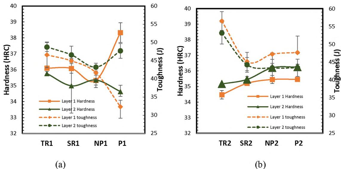
Figure 20. The hardness and toughness properties were compared for the bars obtained from the two layers of the castings from each gating system in (a) mold 1 and (b) mold 2. The hardness and toughness properties were inversely proportional, and the TR system exhibited the highest impact toughness in both the molds
