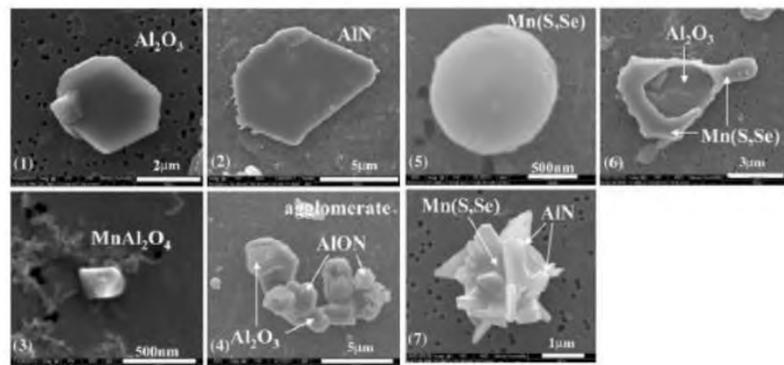
Figure 1.15. Secondary electron images of the different inclusions identified by Park et al. in a Fe-(10-20) Mn-(1-6) Al composition steel [70]
