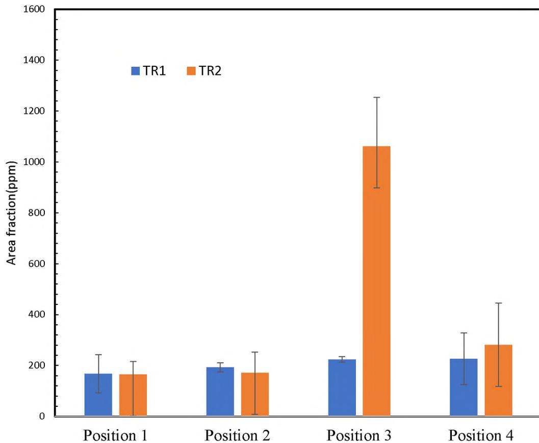
Figure 16. The area fraction of alumina inclusions comparison between the two molds for the TR gating system across different positions. An area fraction between 120-300ppm was found consistently for all positions except one peak of 1200ppm
