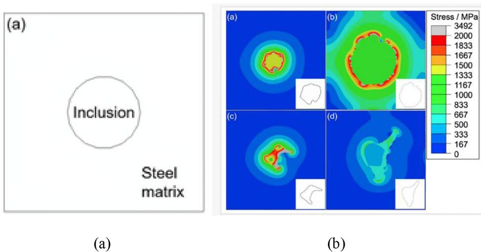
Figure 1.8. The stress concentration between different inclusions and steel matrix was simulated for different inclusion types and morphologies. (a) MgAlO (b) Al-Ca-O-S (c) TiN (d) MnS <sup>[37]</sup>
