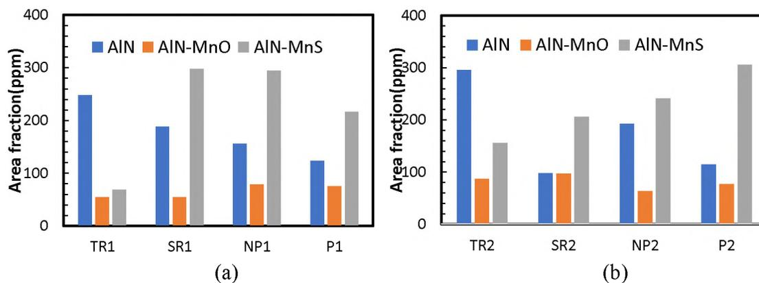
Figure 15. The area fraction of the AlN, AlN-MnO and AlN-MnS inclusions shown for the different gating systems obtained from the surface underneath the fractured Charpy bars. No trends were observed in the inclusion analysis correlating them to fracture toughness
