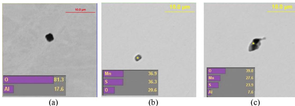
Figure 14. Backscattered electron images of different inclusions and their corresponding chemistries observed in the 8630 steel castings. (a) An alumina inclusion, (b) type 1 MnS, (c) an image showing a complex alumina-manganese sulfide inclusion
