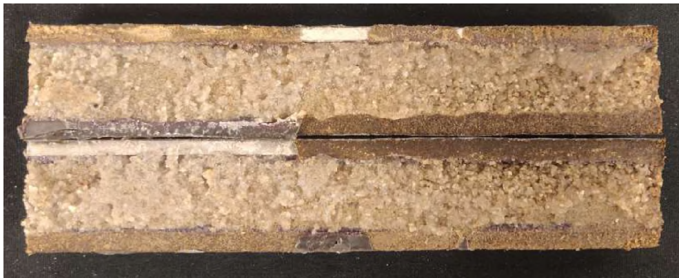
Figure 3.35 The cross-sectional view of experiment model with injecting 170-230 mesh size gel.
