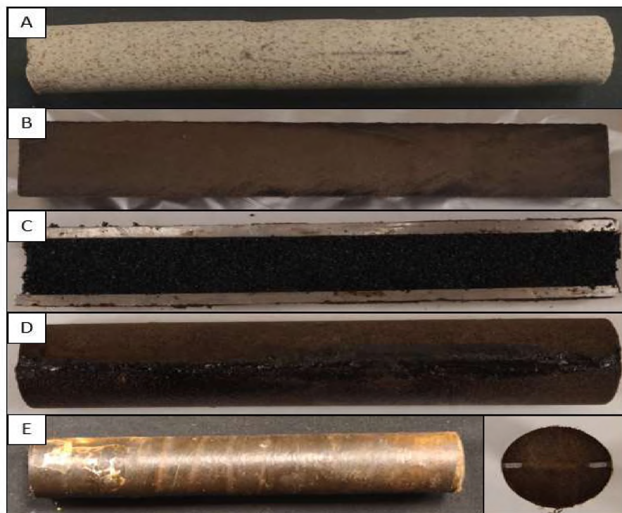
Figure 3.5 The preparations of experiment model. a) core sample before cut. b) saturate and cut the core sample. c) create open fracture and fill the sand. d) glue the fracture with epoxy. e) pack the core sample with Teflon.
