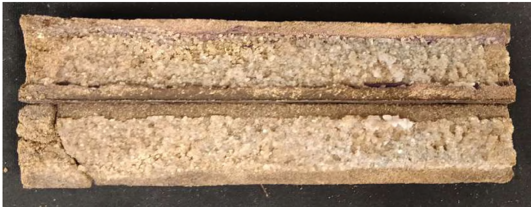
Figure 3.34 The cross-sectional view of experiment model with injecting below 230 mesh size gel.
