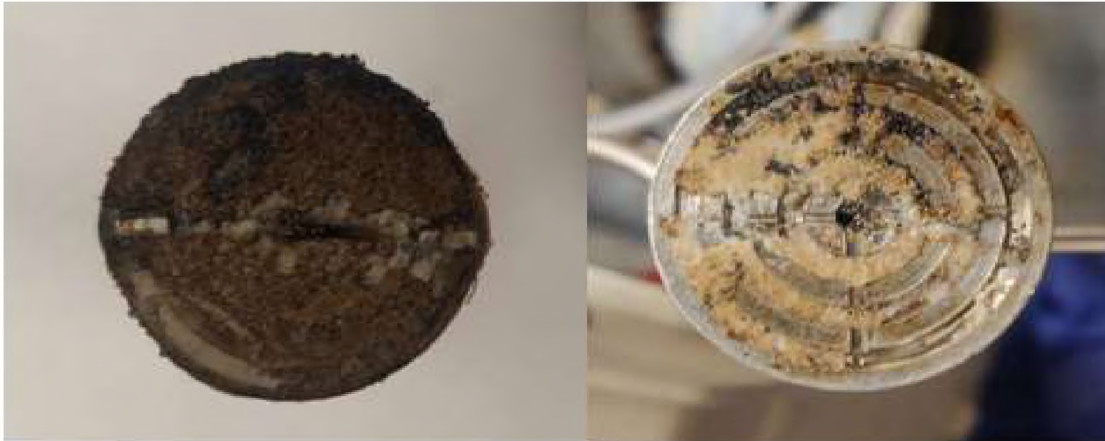
Figure 3.21 The lateral view of experimental model after all procedures were finished. a) the experimental model, the brown color means matrixes and white color means gel particles. b) the inlet injector, the silver color means the surface of injector, the white color means the gel particle.
