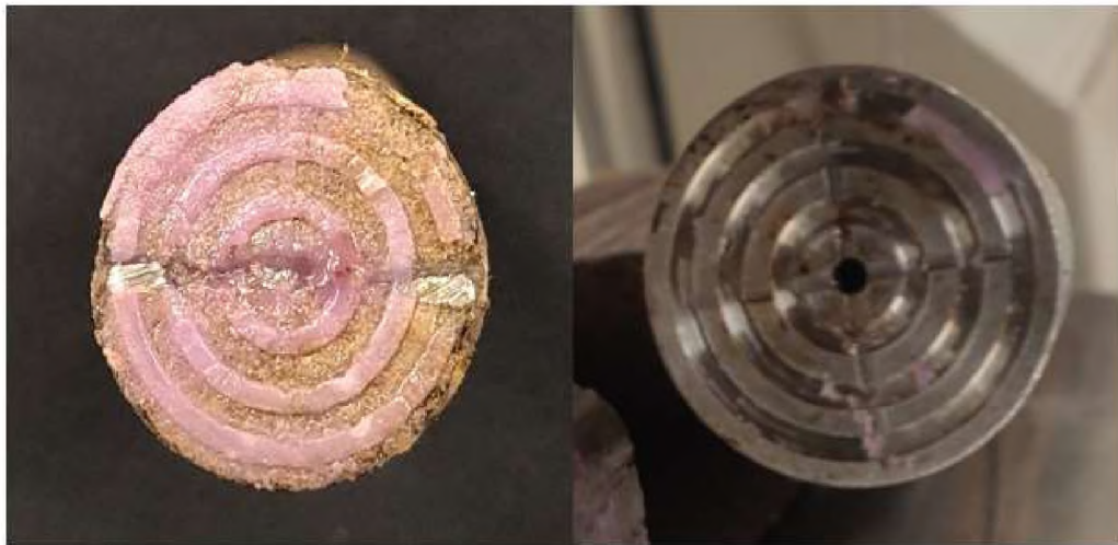
Figure 3.36 The lateral view of experiment model with injecting below 230 mesh size gel.
