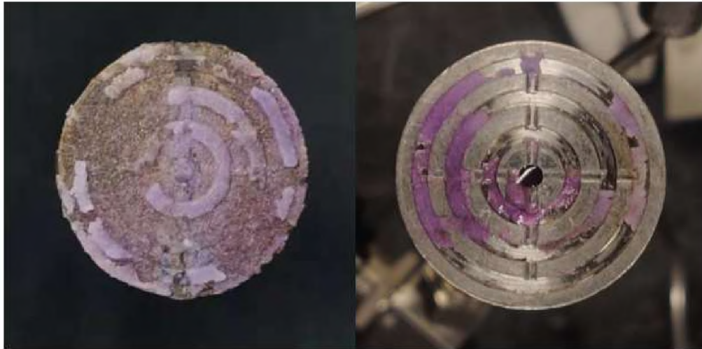
Figure 3.37 The lateral view of experiment model with injecting 170-230 mesh size gel.
