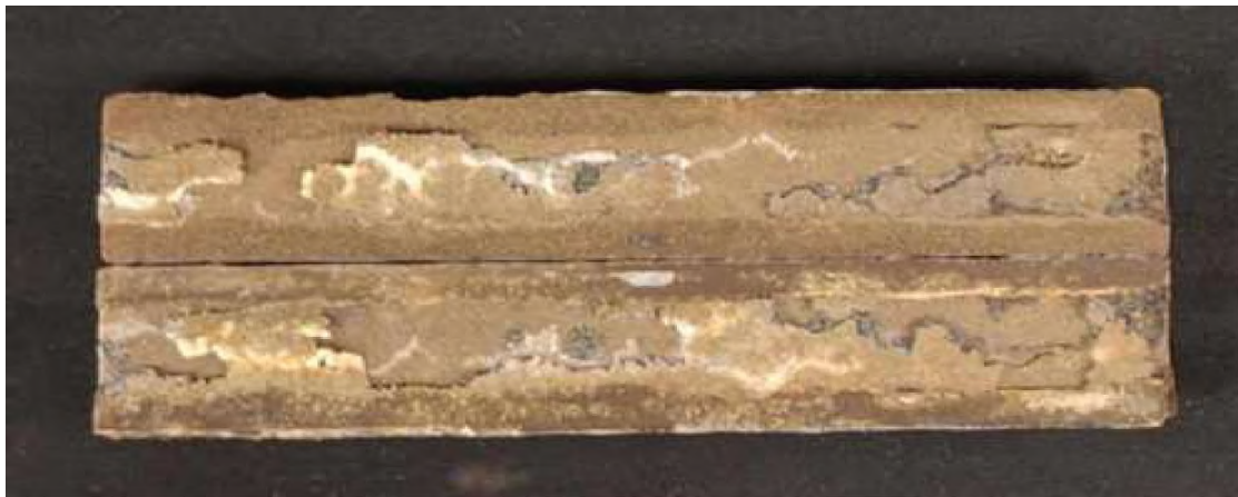
Figure 3.16 The cross-sectional view of experimental model after all procedures were finished (The brown color means sand and white color means gel particle).
