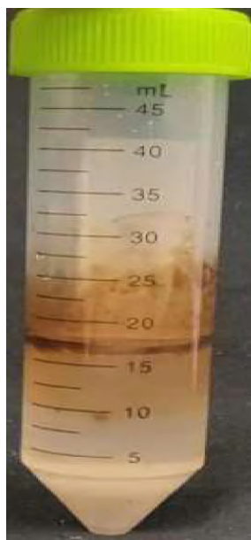
Figure 3.15 Gel particles produced during the second polymer solution injection.
