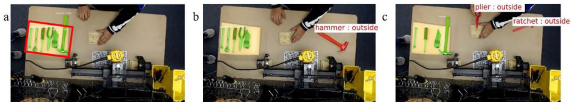
Figure 6. Setup of the workstation. (a) Six tools are highlighted with green mask. From left to right, the tools are wrench, ratchet, screwdriver, plier, Allen key and hammer. The red box indicates the designated area for these tools; (b) a notification is generated by highlighting the hammer with red mask as it gets out of its predefined designated area; (c) notifications generated for plier and ratchet
