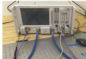
Figure 2.21. Four-port PNA with frequency band up to 50GHz
