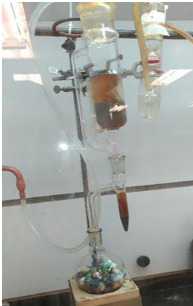
Figure 5.1 The Soxhlet Extraction Apparatus
