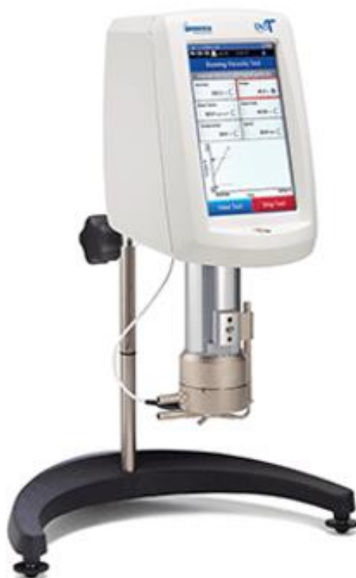
Figure 3.3 The Brookfield DV3T viscometer
