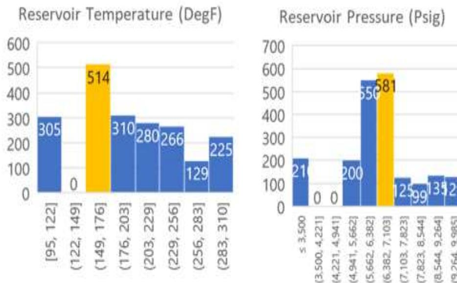
Figure 3-30 Reservoir Temperature and Pressure for Field Scale Simulations
