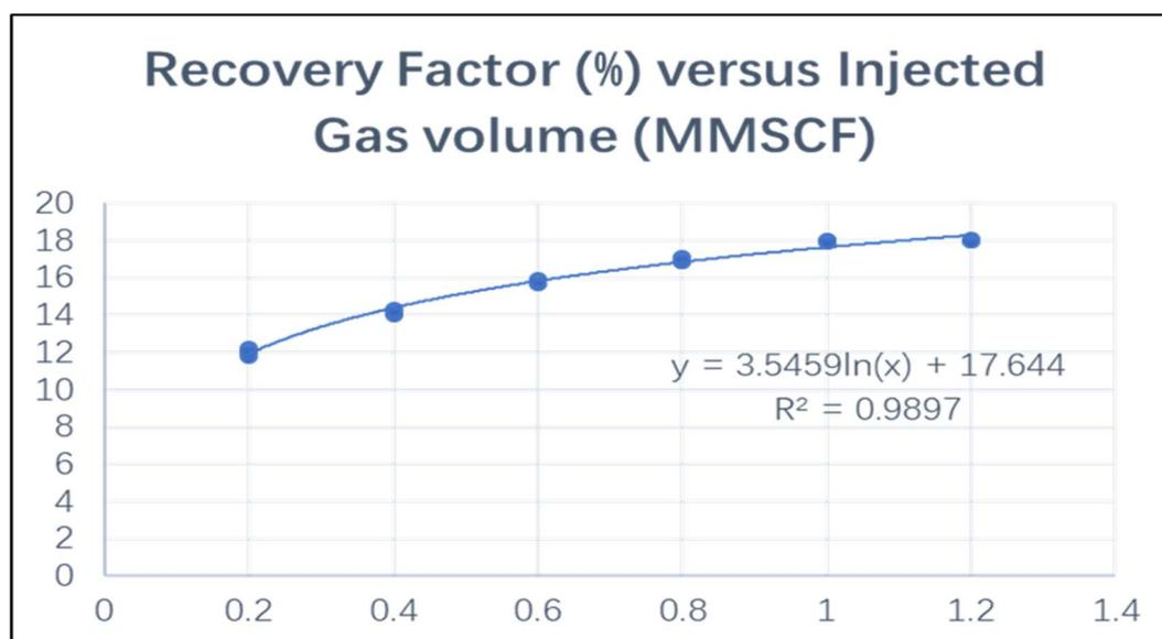
Figure 3-26 Recovery Factors Versus Gas Injected for Core Simulations
