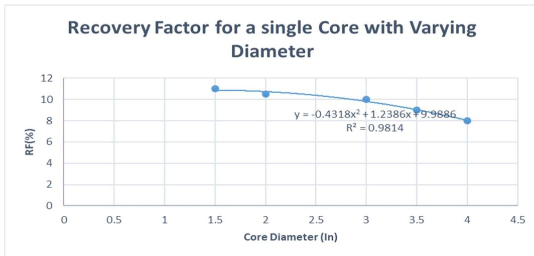
Figure 3-12 Relationship between RF and the Size of the Core
