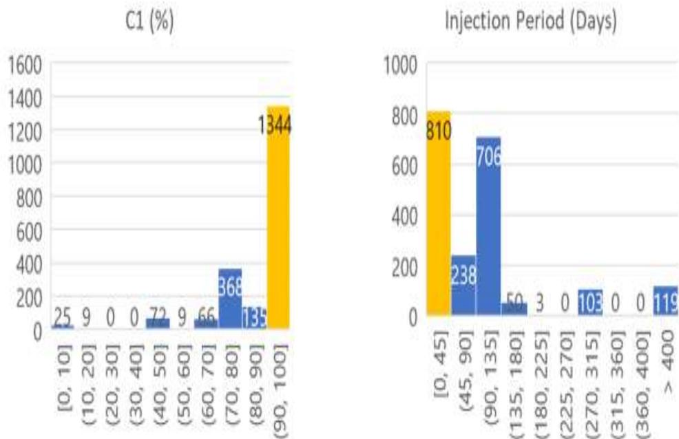
Figure 3-32 Injection Period and C1 % for Field Scale Simulations
