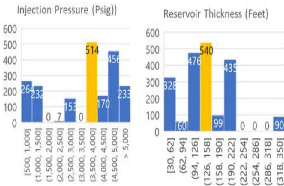
Figure 3-31 Injection Pressure and Thickness for Field Scale Simulations
