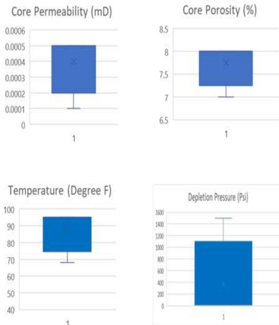
Figure 3-9 Data Ranges for Permeability, Porosity, Temperature, Depletion Pressure
