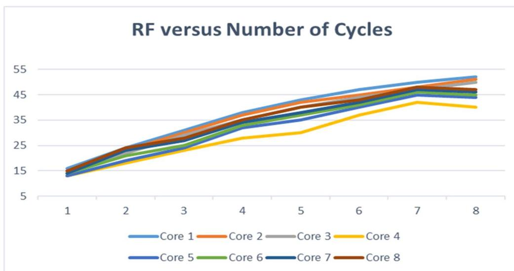
Figure 3-27 Recovery Factor Versus Number of Cycles for Core Simulations
